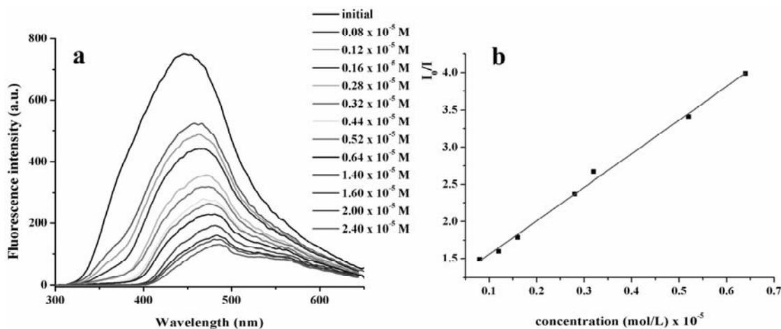
Fig. 4 – Fluorescence spectra of 2% polymer PATrpF in DMF solution, in the absence and presence of *o*-nitrophenol at different concentrations (a),  $\lambda_{\text{exc}} = 280$  nm; the Stern-Volmer plot (b).
