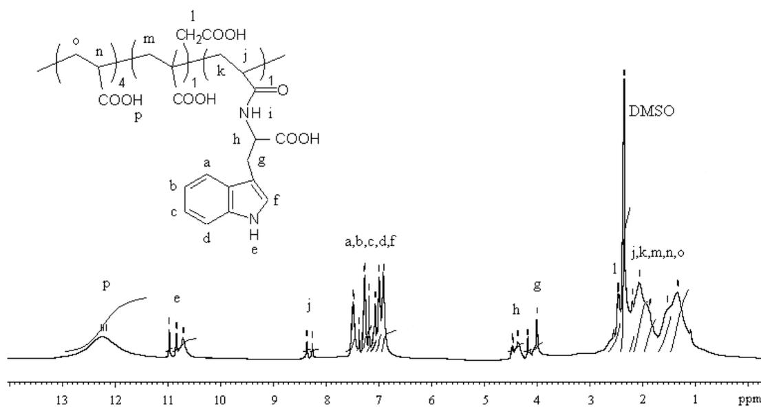
Fig. 1 – <sup>1</sup>H NMR spectrum of copolymer poly(AA-co-IA-co-ATrp) in DMSO-d<sub>6</sub>.
