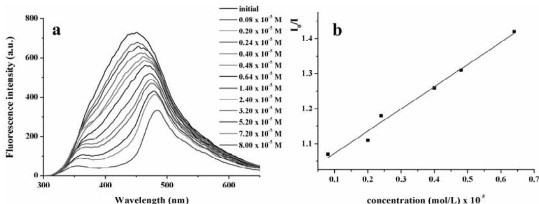
Fig. 3 – Fluorescence spectra of 2% copolymer PATrpF in DMF solution, in the absence and presence of picric acid at different concentrations (a);  $\lambda_{\text{exc}} = 280$  nm; the Stern-Volmer plot (b).
