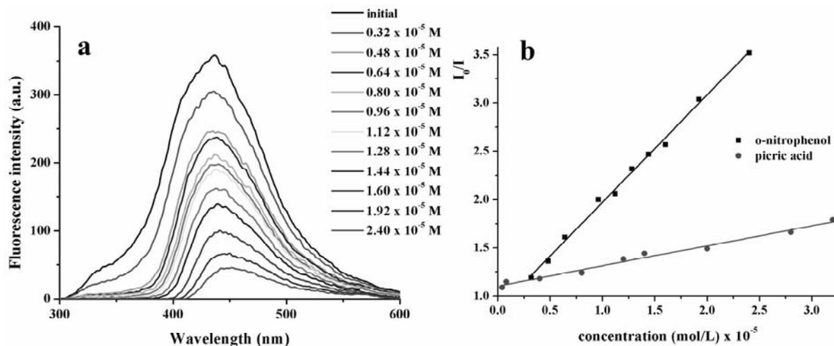
Fig. 5 – Fluorescence spectra of 2% polymer PATrp in dioxane solution, in the absence and presence of *o*-nitrophenol at different concentrations (a),  $\lambda_{\text{ex}} = 280$  nm; the Stern-Volmer plots for fluorescence quenching with picric acid and *o*-nitrophenol (b).
