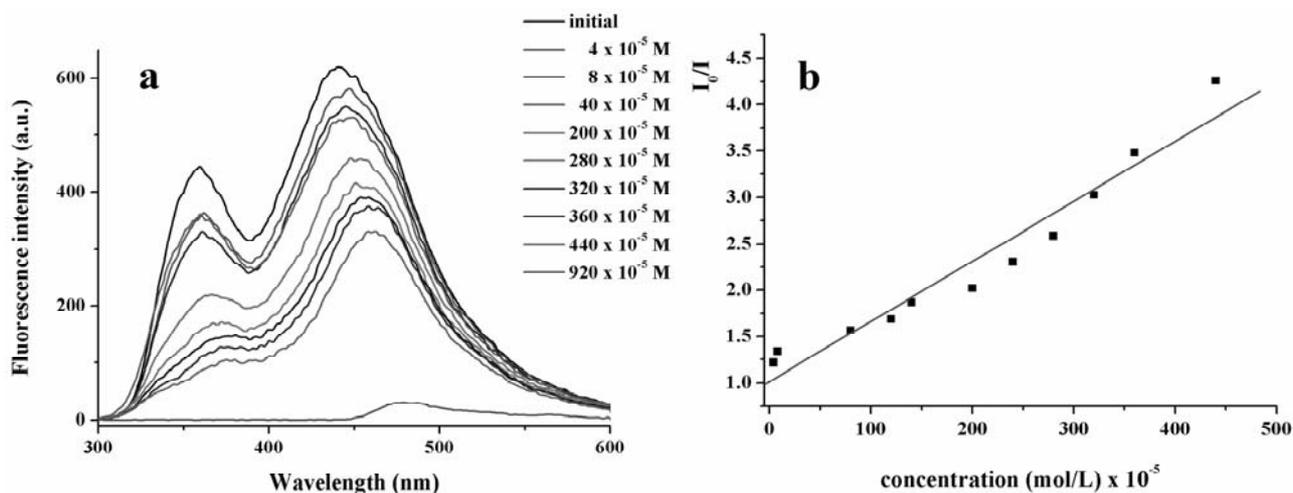
Fig. 6 – Fluorescence spectra of 1% polymer PATrp in dioxane solution in the absence and presence of picric acid at different concentrations (a),  $\lambda_{\text{ex}} = 280$  nm; the Stern-Volmer plot (b).
