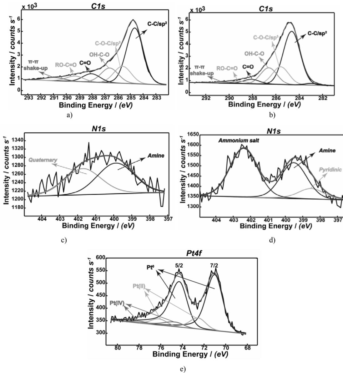
Fig. 6 – XPS C1s deconvoluted spectrum for graphene (a), XPS C1s deconvoluted spectrum for Pt/graphene, XPS N1s deconvoluted spectrum for graphene (c), XPS N1s deconvoluted spectrum for Pt/graphene (d), XPS Pt4f deconvoluted spectrum for Pt/graphene (e).
