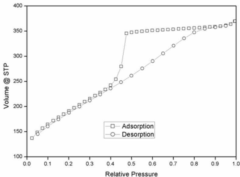
Fig. 2 – The adsorption–desorption isotherms for graphene.
