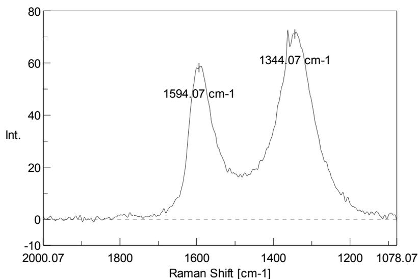
Fig. 4 – Raman spectra for Pt/graphene.
