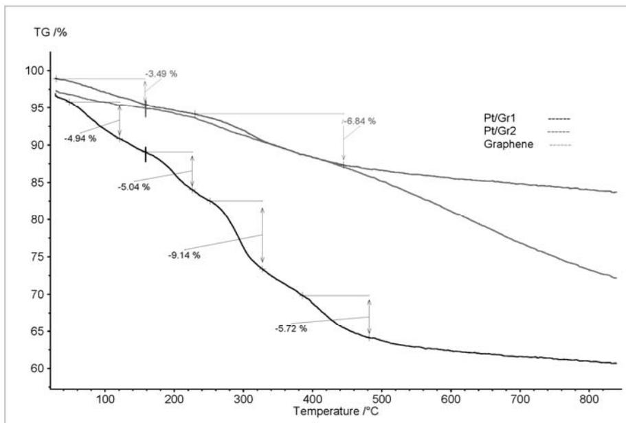
Fig. 5 – Thermogravimetric analysis of graphene and Pt/graphene.
