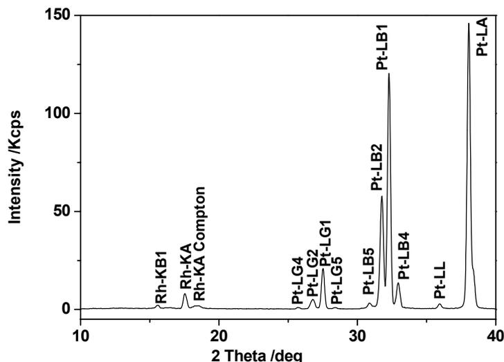
Fig. 3 – X-ray fluorescence spectrum of the Pt/graphene nanocomposite.
