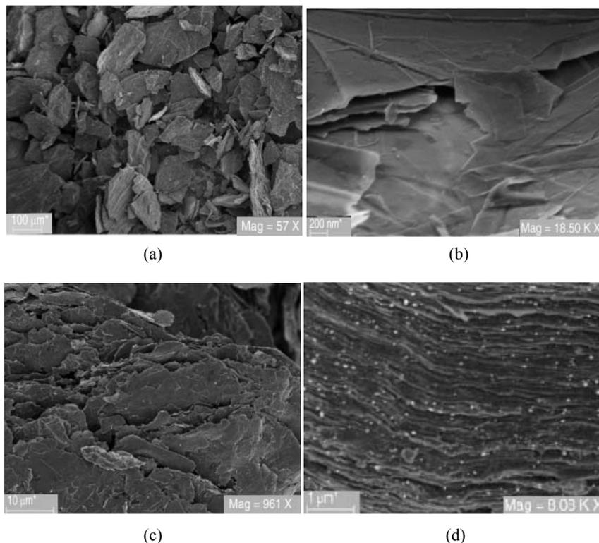
Fig. 1 – The SEM micrographs of the graphite oxide (a), graphene (b), graphene nanocomposites (c, d).
