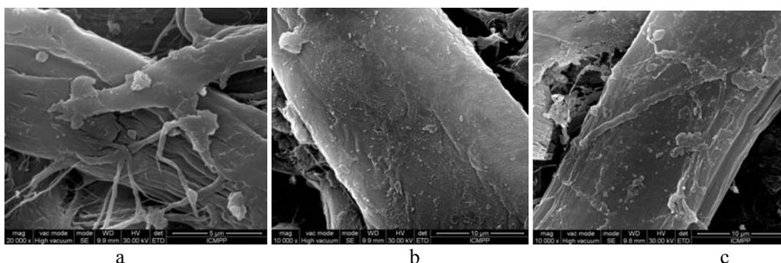
Fig. 4 – SEM micrographs – the superficial aspect of industrial paper – sample P<sub>2</sub>. a – initial aspect of the cellulose fiber structure, b – cellulose fiber structure after 20 min treatment in N<sub>2</sub>, c – cellulose fiber structure after 20 min treatment in Ar/O<sub>2</sub>.
