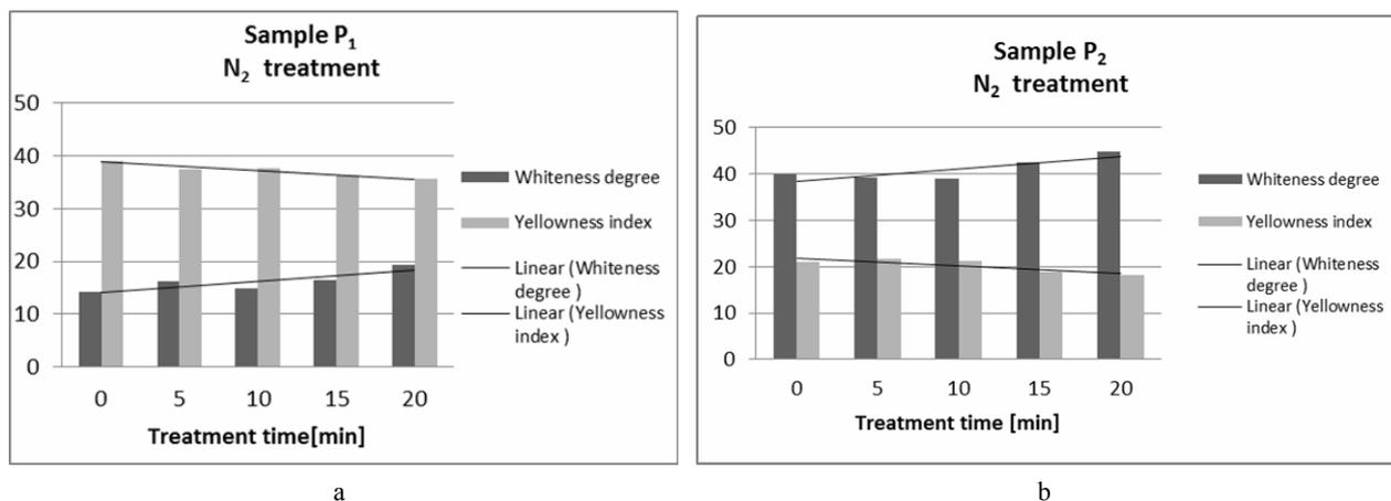
Fig. 6 – Variation of whiteness degree and yellowness index for N<sub>2</sub> plasma treatment. a – P<sub>1</sub> sample treated in nitrogen plasma, b – P<sub>2</sub> sample treated in nitrogen plasma.
