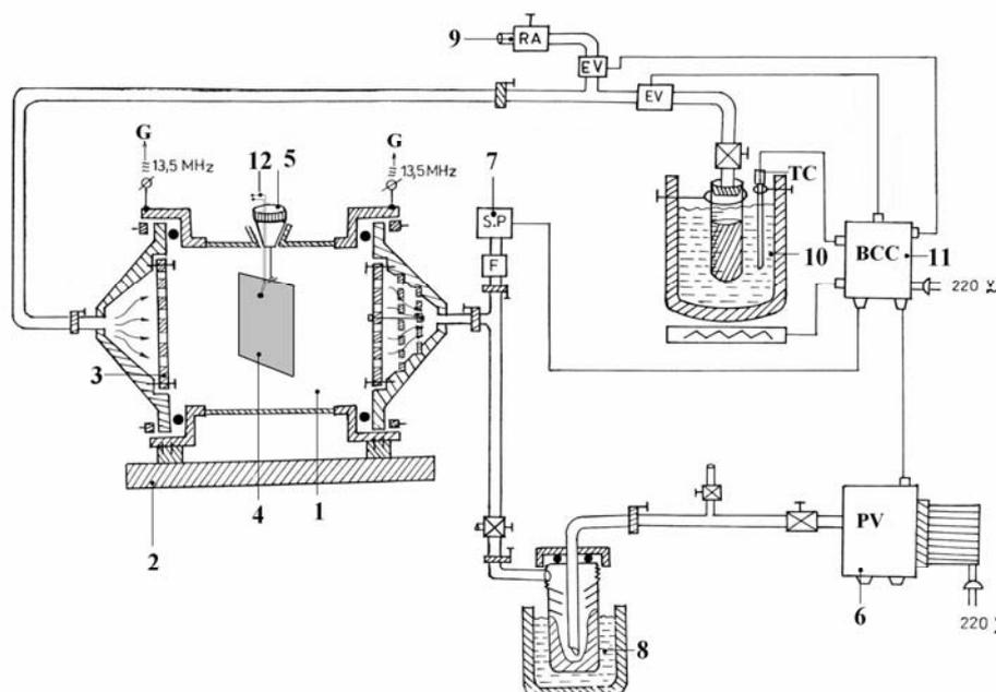
Fig. 1 – Schematic presentation of the RF plasma unit.
