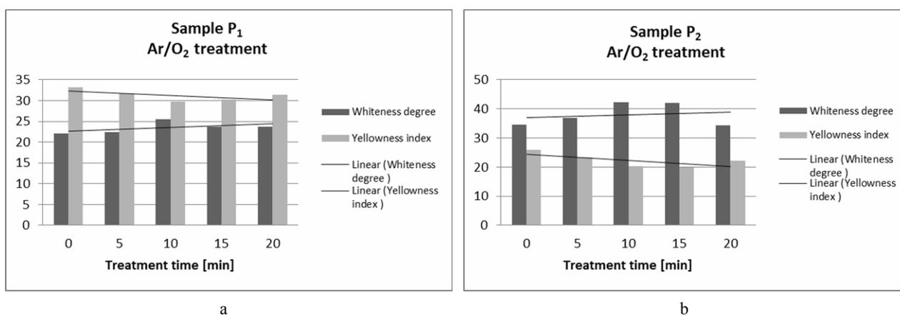
Fig. 7 – Variation of whiteness degree and yellowness index for Ar/O<sub>2</sub> plasma treatment. a – P<sub>1</sub> sample treated in Ar/O<sub>2</sub> plasma, b – P<sub>2</sub> sample treated in Ar/O<sub>2</sub> plasma.
