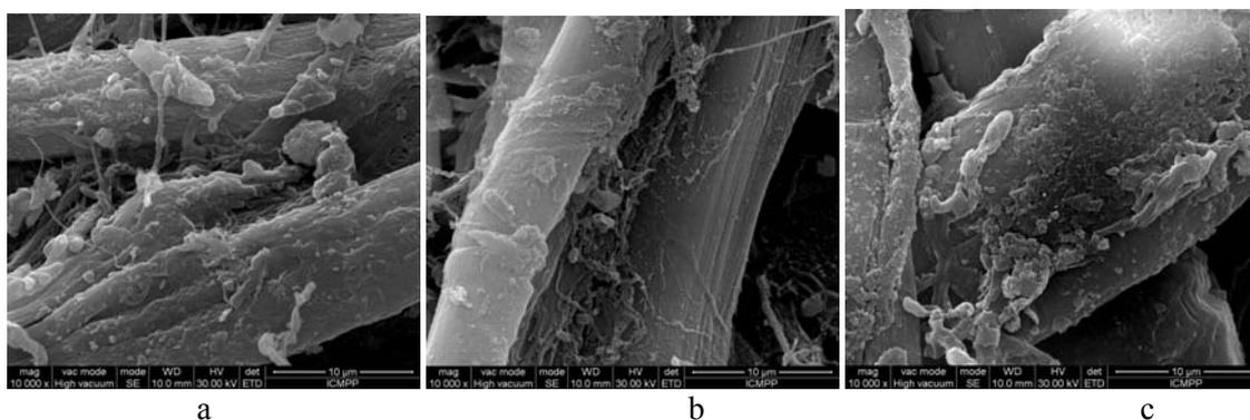
Fig. 3 – SEM micrographs- the superficial aspect of handmade paper - sample P<sub>1</sub>; a – initial aspect of the cellulose fiber structure, b – cellulose fiber structure after 20 min treatment in N<sub>2</sub>, c – cellulose fiber structure after 20 min treatment in Ar/O<sub>2</sub>.
