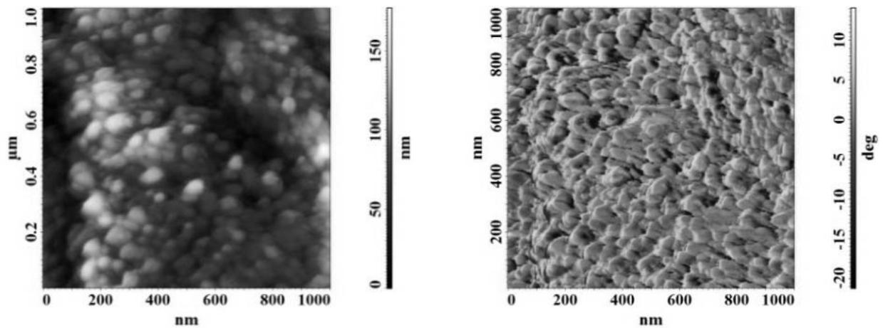
Fig. 2 – AFM height (a) and phase (b) images for the sample prepared with 0.05 wt.% PHOS-*b*-PMAA.
