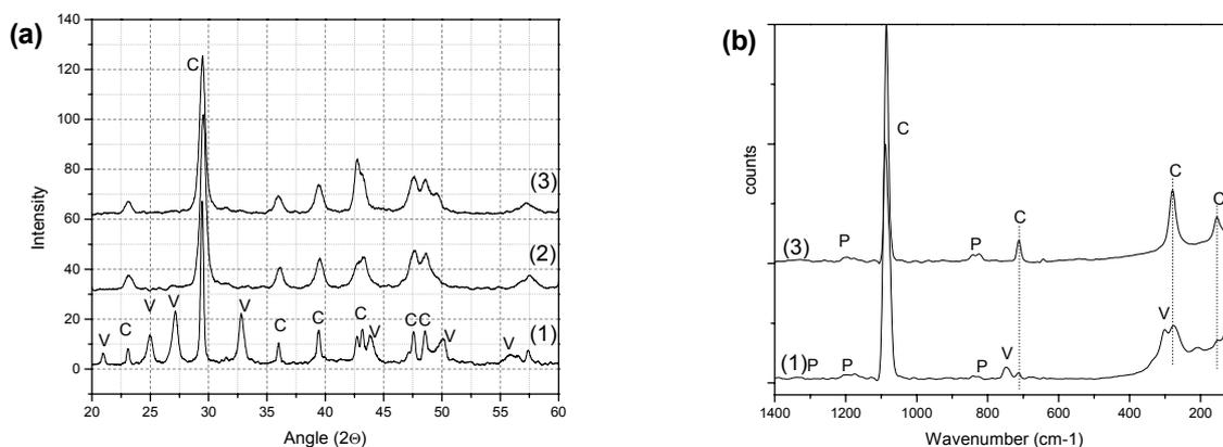
Fig. 3 – (a) XRD diffractograms and (b) Raman spectra of CaCO<sub>3</sub>/PHOS-*b*-PMAA microparticles, prepared with different polymer concentrations; (1) 0.05 wt.%, (2) 0.07 wt.%, (3) 0.10 wt. %
