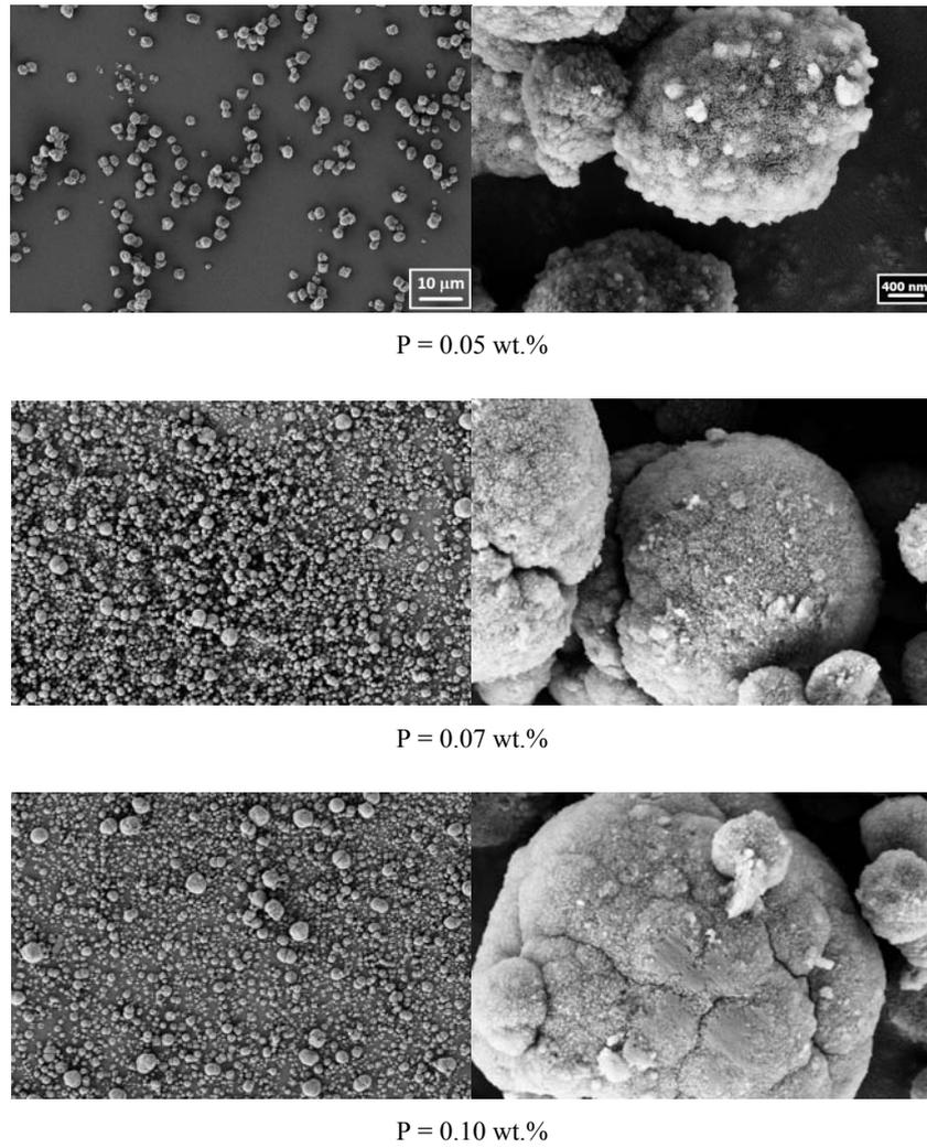
Fig. 1 – SEM images of  $\text{CaCO}_3/\text{PHOS-}b\text{-PMAA}$  particles prepared at  $\text{pH} = 12$ , using 0.2 M calcium and carbonate ions concentration and different polymer concentrations.
