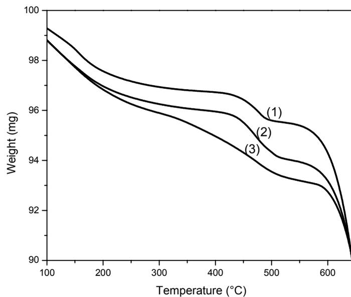
Fig. 4 – TGA plots of CaCO<sub>3</sub>/PHOS-*b*-PMAA composites with various contents in block copolymer; (1) 0.05 wt.%, (2) 0.07 wt.%, (3) 0.10 wt.%
