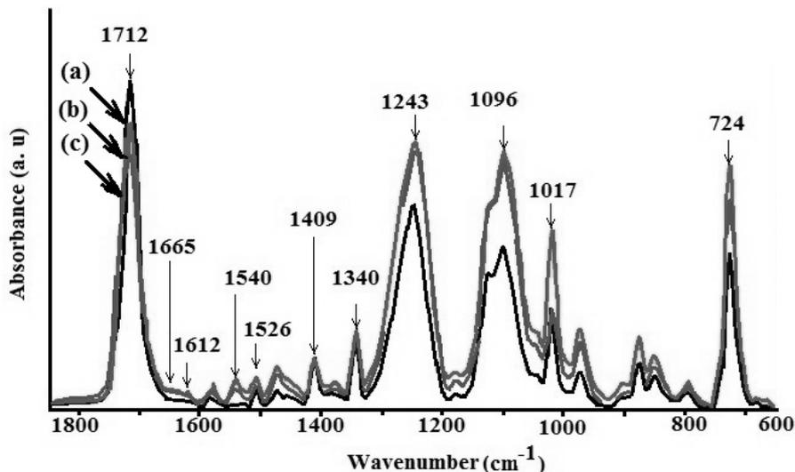
Fig. 1 – ATR-FTIR spectra for (a) untreated PET; (b) adsorbed collagen on plasma action PET film P1 and (c) P2.
