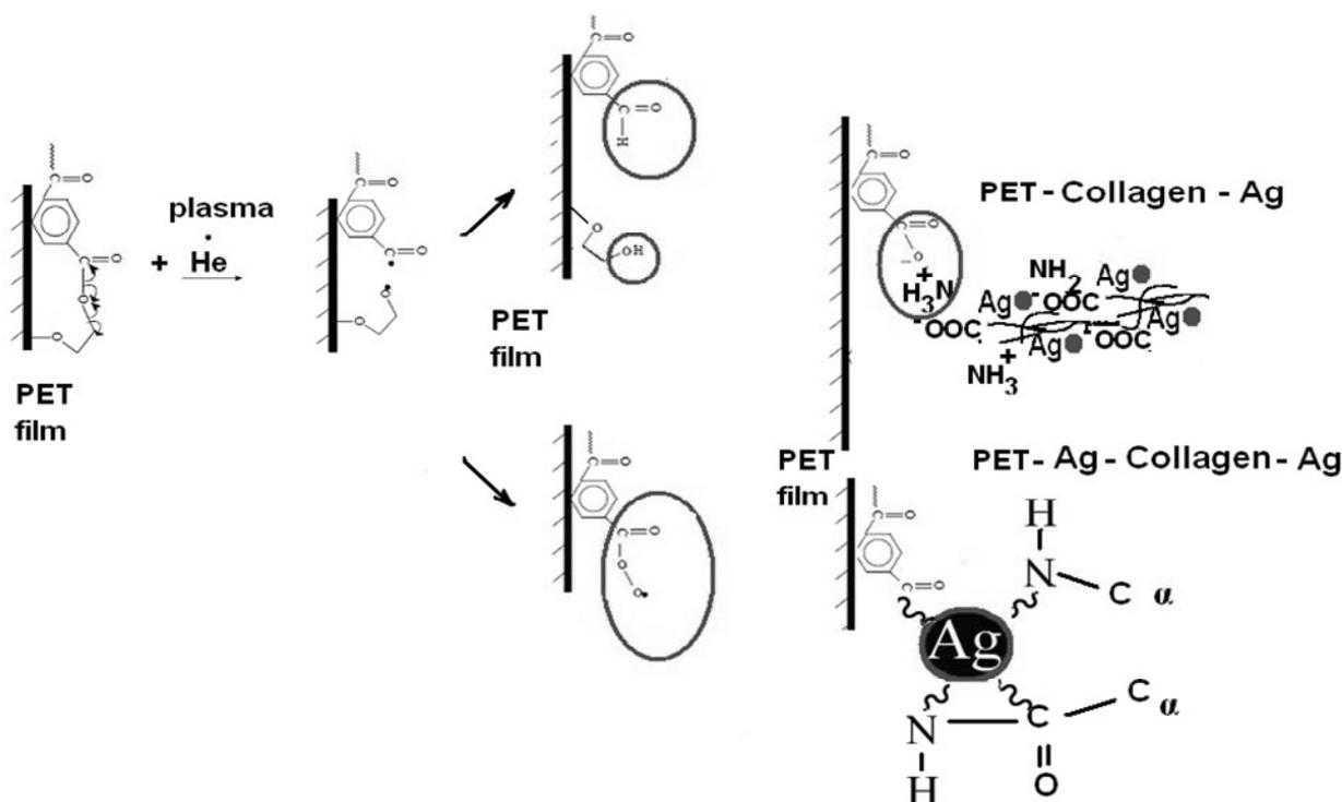
Fig. 2 – A schematic mechanism of collagen adsorption on functionalized PET film.
