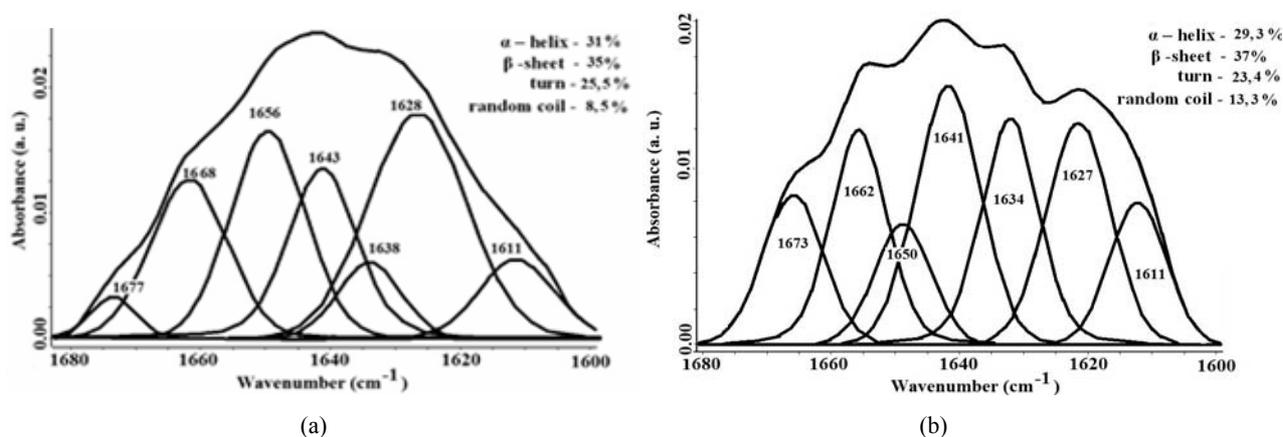
Fig. 4 – Curve-fitted amide I ( $1700 - 1600 \text{ cm}^{-1}$ ) band from FTIR spectra of collagen immobilized on functionalized PET films P<sub>1</sub> (a) and P<sub>2</sub> (b).
