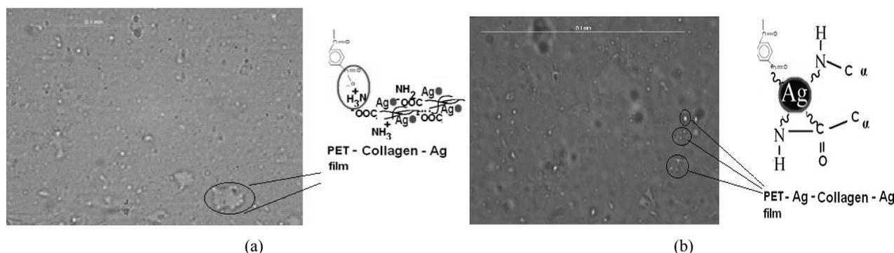
Fig. 3 – Optical microscopy images of Ag-collagen regions immobilized on PET plasma treated (a) P1 and (b) P2.
