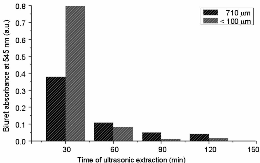
Fig. 1 – The biuret absorbance of alcoholic extracts sampled at different extraction times under ultrasonication at 25  $^\circ\text{C}$ .
