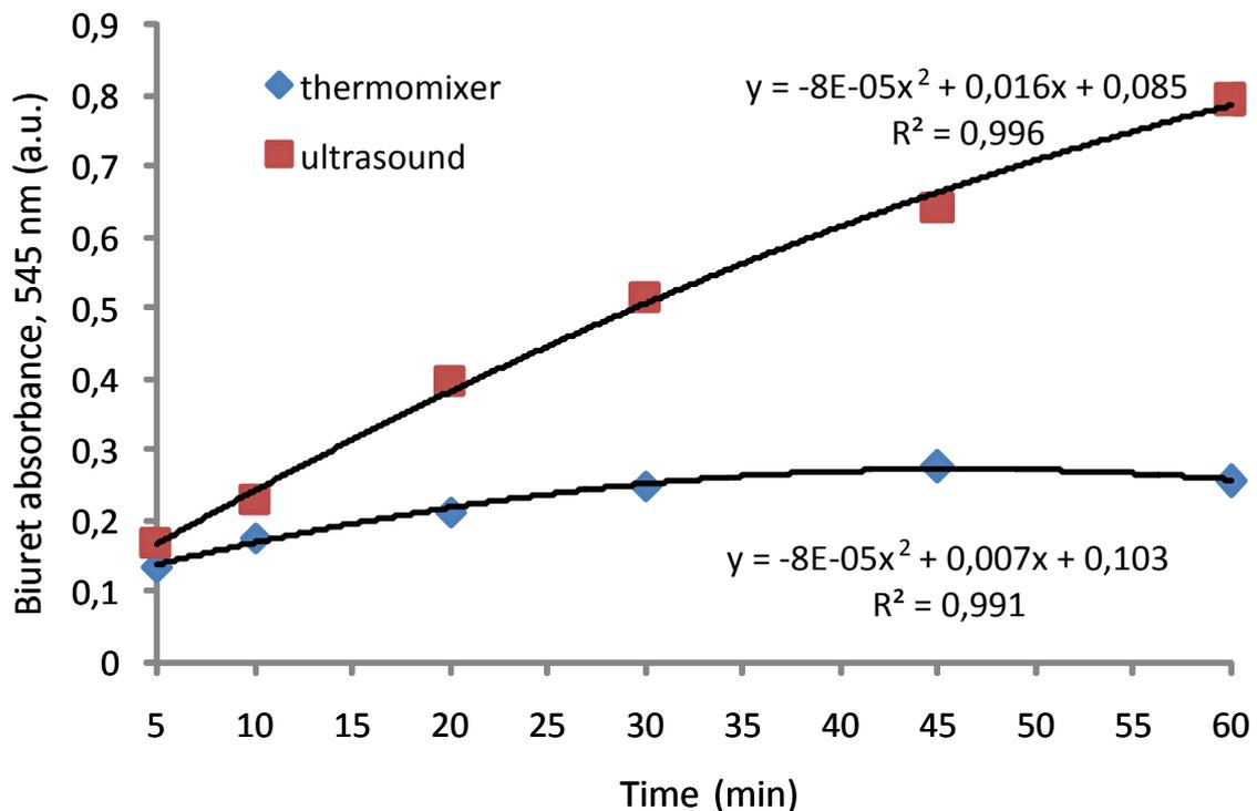
Fig. 4 – The kinetic of zein extraction from the 500  $\mu\text{m}$  maize flour followed by the biuret absorbance measurement. The biuret absorbance was read at 545 nm and at 5 min, 10 min, 20 min, 30 min, 45 min, and 60 min, respectively.
