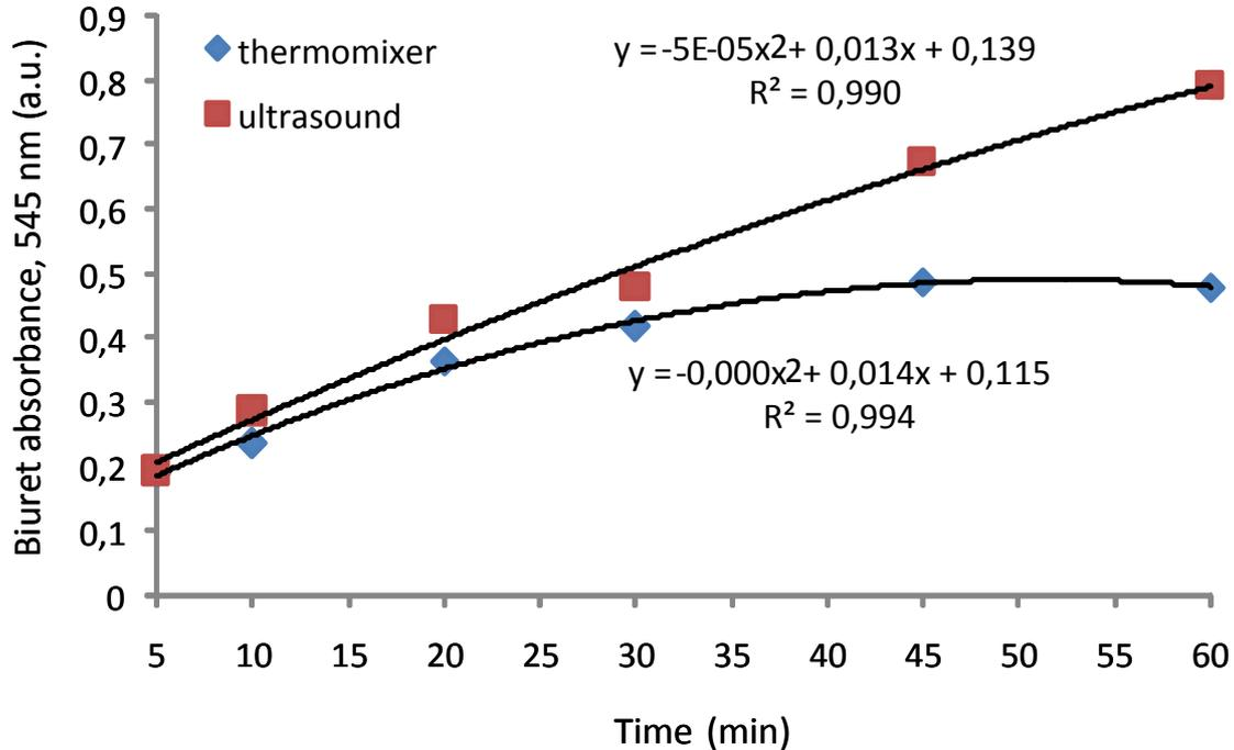
Fig. 3 – The evolution of biuret absorbance during the zein extraction from 250  $\mu\text{m}$  maize flour. The 545 nm spectrophotometric reading was made at 5 min, 10 min, 20 min, 30 min, 45 min, and 60 min, respectively.
