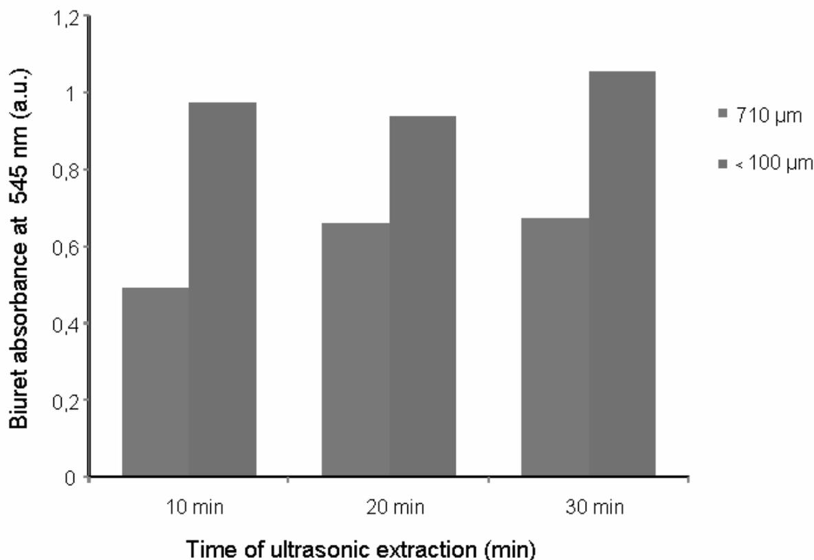
Fig. 2 – The biuret absorbance of the extracts sampled at different extraction times under ultrasonication at 60 °C.
