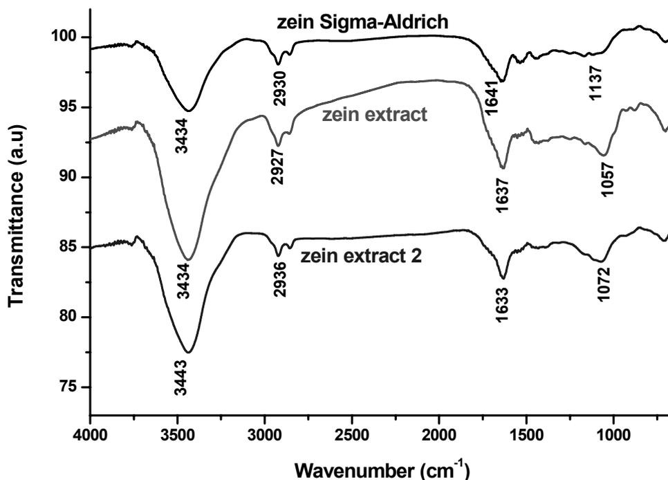
Fig. 5 – FT-IR spectra of zein extracts: zein from Sigma-Aldrich, used as control sample, the crude zein from the alcoholic extract (zein extract) and zein from zein extract, purified by two time washing with water (zein extract 2).
