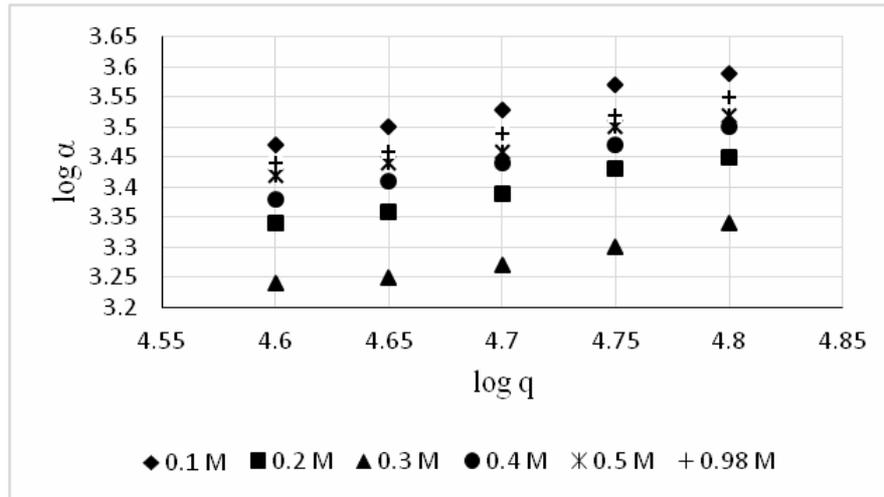
Fig. 3 – Boiling heat transfer coefficient as a function of heat flux at different molar concentrations of n-propanol – water solutions.
