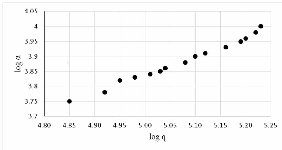
Fig. 1 – Boiling heat transfer coefficient as a function of heat flux for water.
