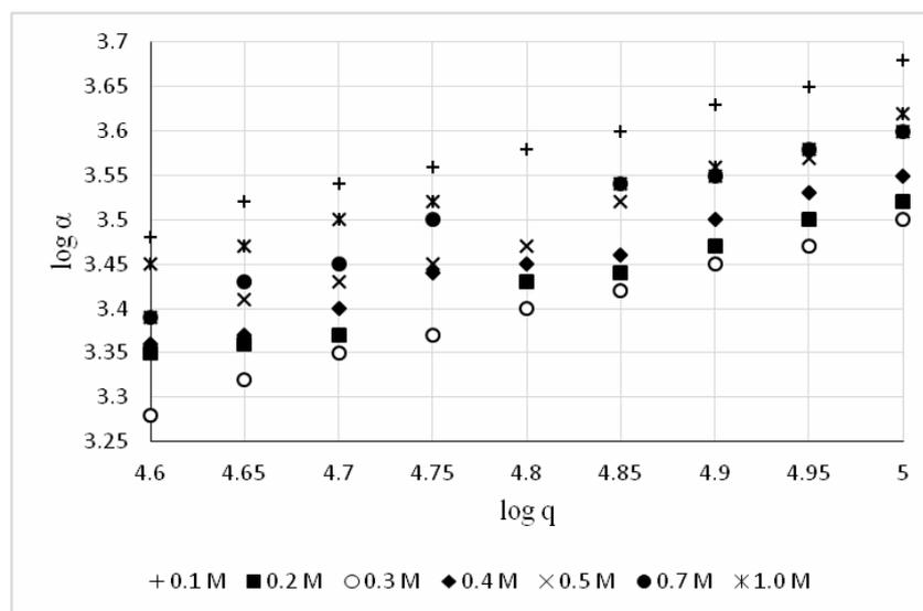
Fig. 2 – Boiling heat transfer coefficient as a function of heat flux at different molar concentrations of ethanol – water solutions.
