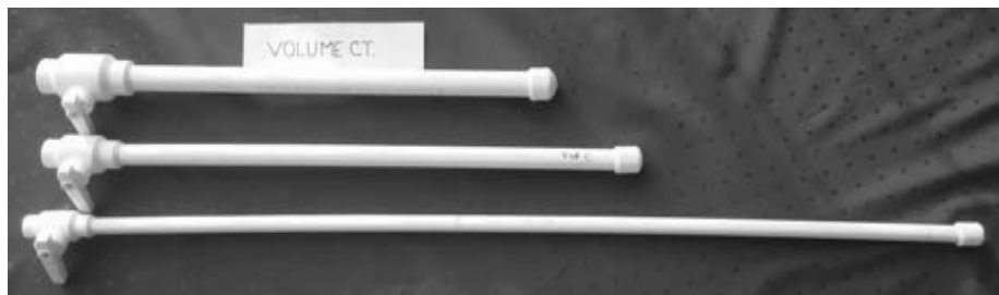
Fig. 1 – PPR pipes having the same volume but exhibiting different surfaces for contact with water.
