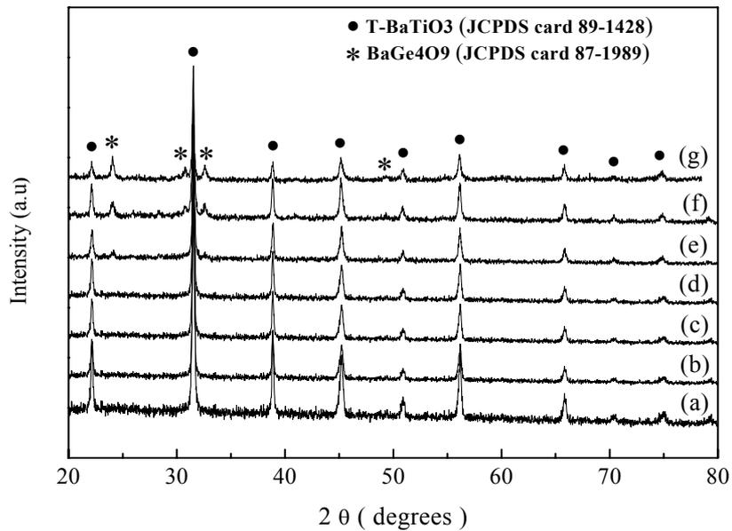
Fig. 1 – XRD patterns for pure  $\text{BaTiO}_3$  (a) And  $\text{Ge}_x\text{BaTiO}_3$  samples where:  $x = 0.01$  (b) 0.05 (c) 0.1 (d) 0.2 (e) 0.5 (f) and 1 (g).
