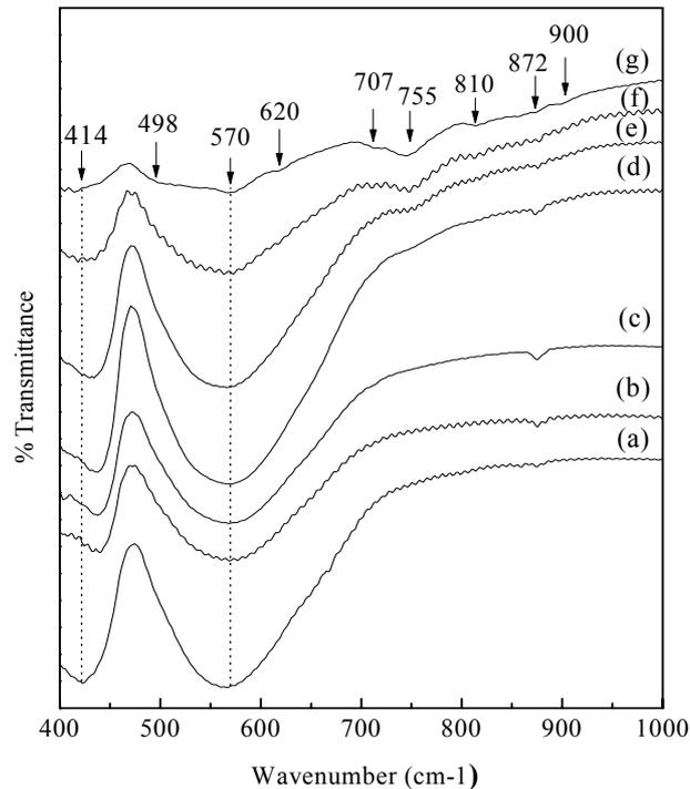
Fig. 4 – FT-IR spectra for pure BaTiO<sub>3</sub> (a) and Ge<sub>x</sub>BaTiO<sub>3</sub> samples where : x= 0.01 (b) 0.05 (c) 0.1(d) 0.2 (e) 0.5 (f) and 1 (g).
