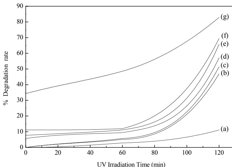
Fig. 6 – Photocatalytic degradation rate under UV irradiation of Methyl Red solution in the presence of: pure  $\text{BaTiO}_3$  (a),  $\text{Ge}_x\text{BaTiO}_3$  where:  $x=0.01$  (b) 0.05 (c) 0.1 (d) 0.2 (e) 0.5 (f) and 1 (g).
