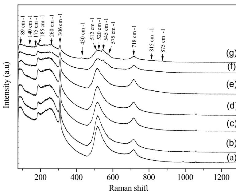
Fig. 3 – Micro-Raman Spectra for pure  $\text{BaTiO}_3$  (a) and  $\text{Ge}_x\text{BaTiO}_3$  samples where :  $x = 0.01$  (b)  $0.05$  (c)  $0.1$  (d)  $0.2$  (e)  $0.5$  (f) and  $1$  (g).
