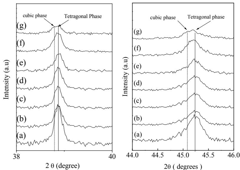
Fig. 2 – XRD patterns, in the ranges  $2\theta = 36 - 38^\circ$  and  $2\theta = 44 - 46^\circ$  for pure  $\text{BaTiO}_3$  (a) And  $\text{Ge}_x\text{BaTiO}_3$  samples where:  $x = 0.01$  (b) 0.05 (c) 0.1 (d) 0.2 (e) 0.5 (f) and 1 (g).
