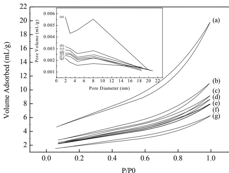
Fig. 5 – Nitrogen adsorption-desorption isotherms and pore size distributions for pure BaTiO<sub>3</sub> (a), Ge<sub>x</sub>BaTiO<sub>3</sub> where x= 0.01 (b) 0.05 (c) 0.1(d) 0.2 (e) 0.5 (f) and 1 (g).
