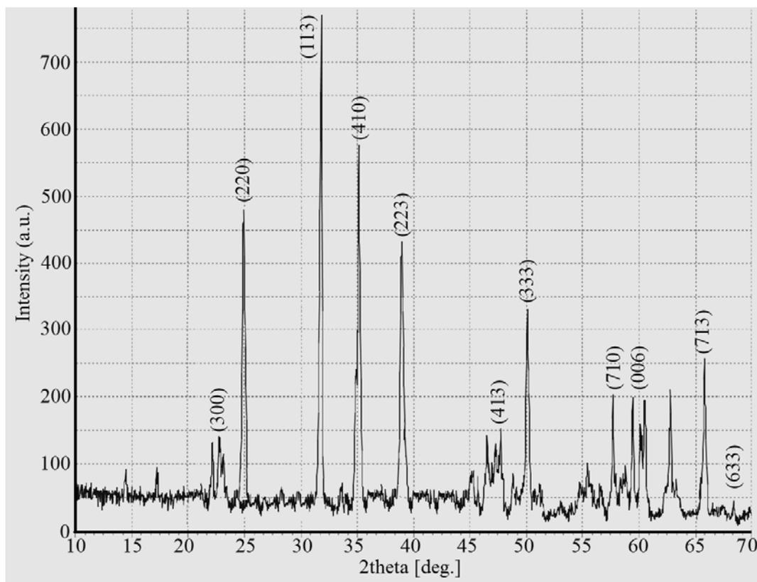
Fig. 4 – The XRD spectrum of manganese-doped  $\text{Zn}_2\text{SiO}_4$  nanoparticles.
