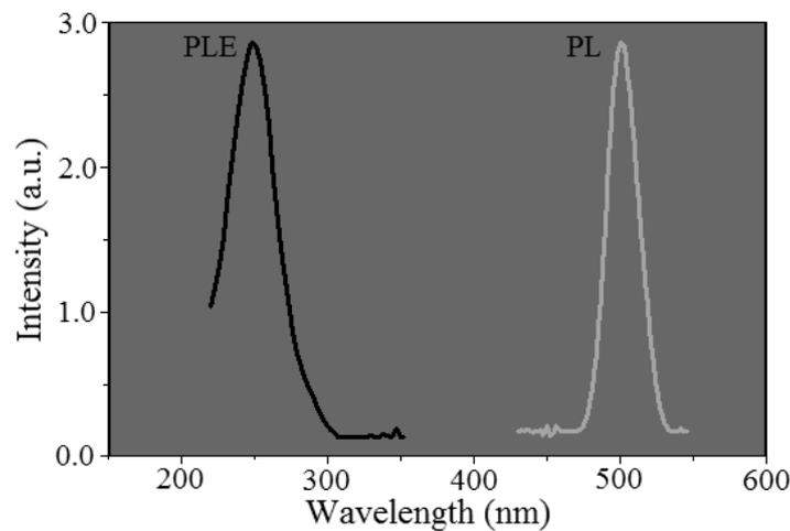
Fig. 5 – The luminescence spectrum of manganese-doped  $\text{Zn}_2\text{SiO}_4$  nanoparticles.
