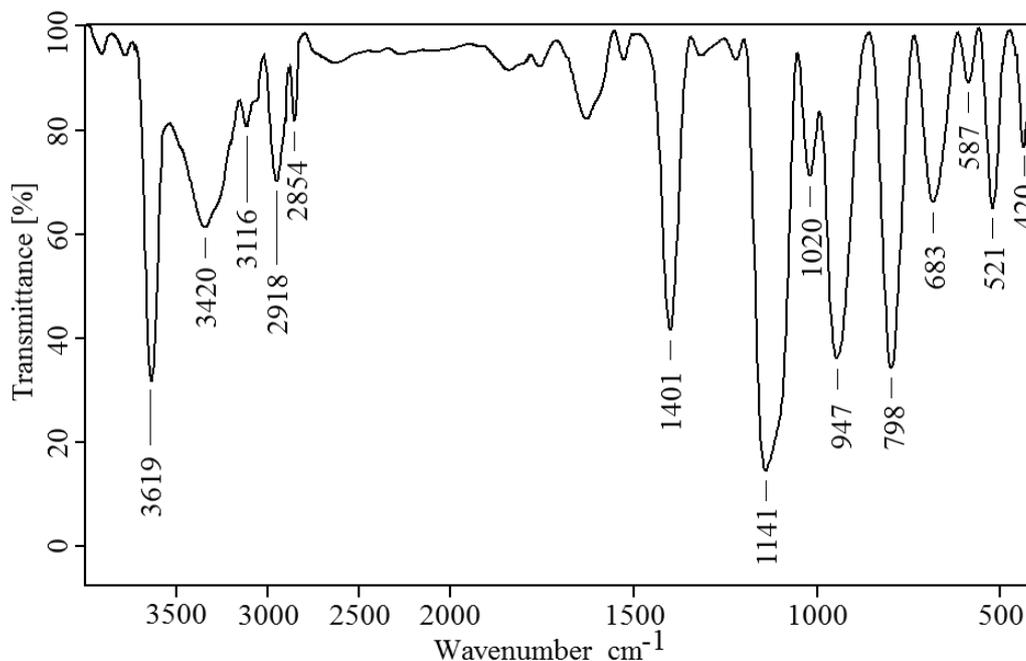
Fig. 3 – The FT-IR spectrum of the synthesized  $\text{Zn}_2\text{SiO}_4:\text{Mn}^{2+}$  nanoparticles (after smoothing, baseline correction and normalization).
