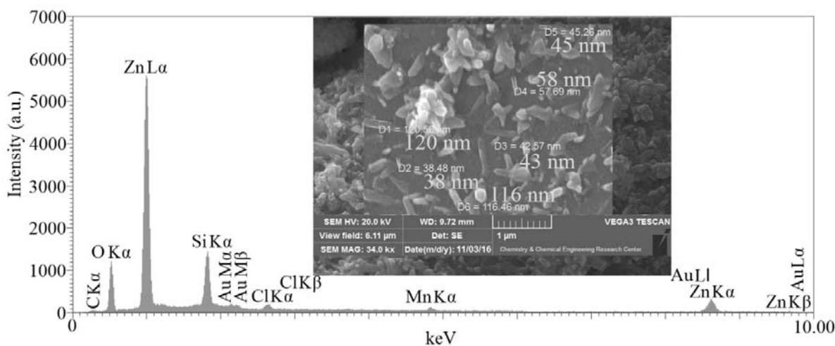
Fig. 2 – EDX spectrum and the electron microscopy image of manganese-doped  $\text{Zn}_2\text{SiO}_4$  nanoparticles.
