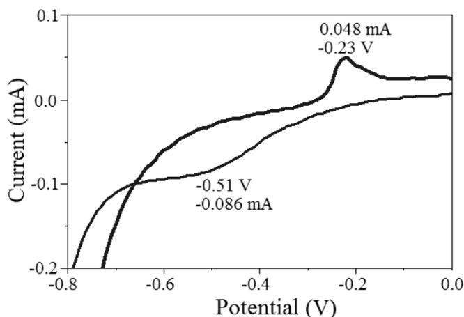
Fig. 1 – The cyclic voltammogram of  $\text{SiO}_2$  formation starting with  $(\text{NH}_4)_2\text{SiF}_6$  solution containing  $\text{KCl}$  0.5 M on the composite graphite electrode. The range of the potential was -0.8–0.0 V with a scan rate of 100 mV/s.
