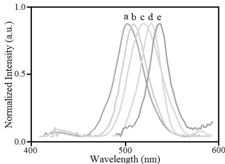
Fig. 6 – The luminescence diagram of zinc silicate particles doped with different concentrations of manganese in the electrosynthesis process. (a–e) Changes in the concentration of manganese nitrate from 0.01 to 0.02, 0.04, 0.06, and 0.08 M, respectively.
