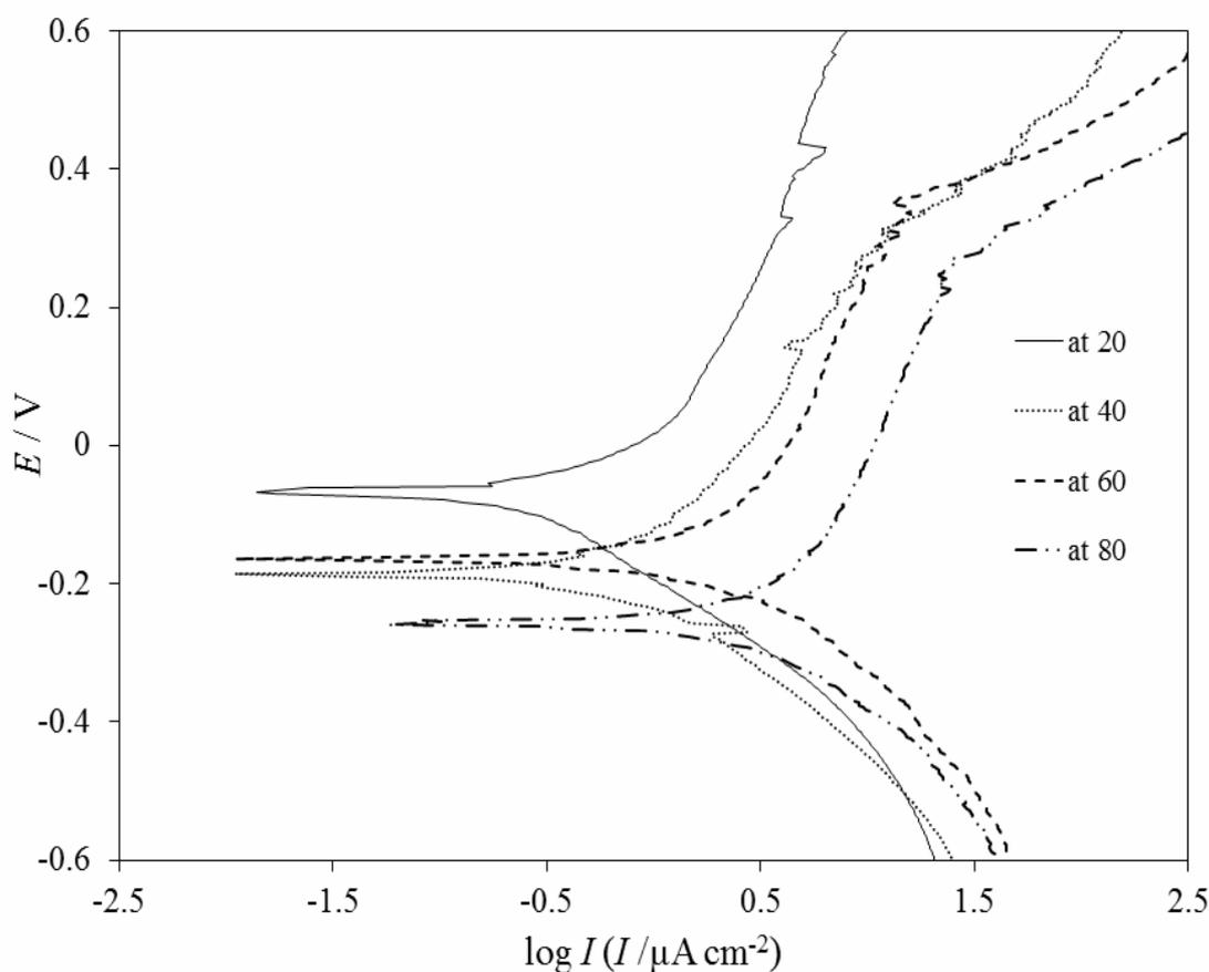
Fig. 6 – Polarization curves of duplex stainless steel electrode in 100 ppm NaCl and 10% ethylene glycol-water solution at different temperature.
