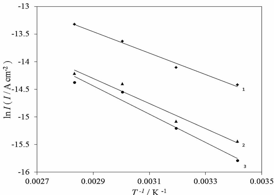
Fig. 7 – Typical Arrhenius plots of  $\ln(I_{corr})$  vs.  $T^{-1}$  for steel alloy in  $100 \times 10^{-6}$  NaCl at different concentrations of ethylene glycol: 1: 10; 2: 30; 3: 50 %V/V ethylene glycol.
