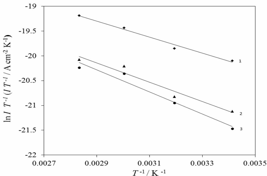
Fig. 8 – Typical Arrhenius plots of  $\ln(I_{corr} T^{-1})$  vs.  $T^{-1}$  for steel alloy in 100 ppm NaCl at different concentrations of ethylene glycol: 1: 10; 2: 30; 3: 50 %V/V ethylene glycol.
