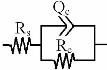
Fig. 5 – Equivalent circuits compatible with the experimental impedance data for corrosion of duplex steel alloy electrode in ethylene glycol solution.
