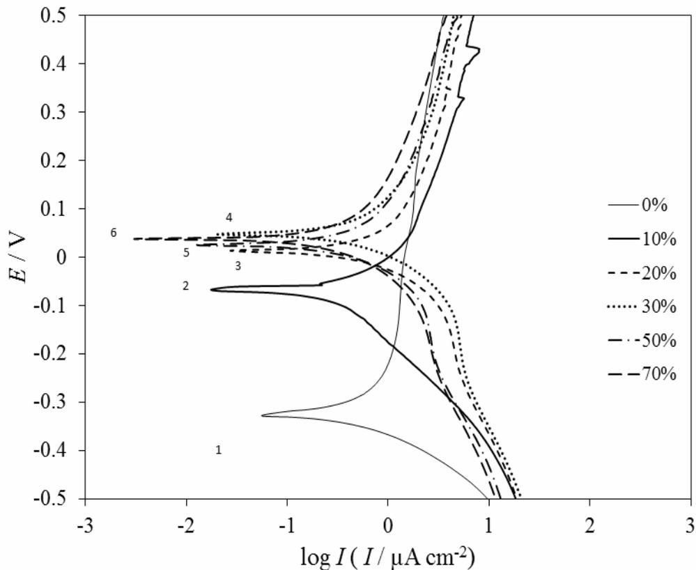
Fig. 1 – Polarization curves of duplex steel alloy electrode in 100 ppm NaCl and ethylene glycol-water solution with different concentrations of ethylene glycol: 1: 0 ; 2: 10; 3: 20; 4: 30; 5: 50; 6: 70 %V/V ethylene glycol.
