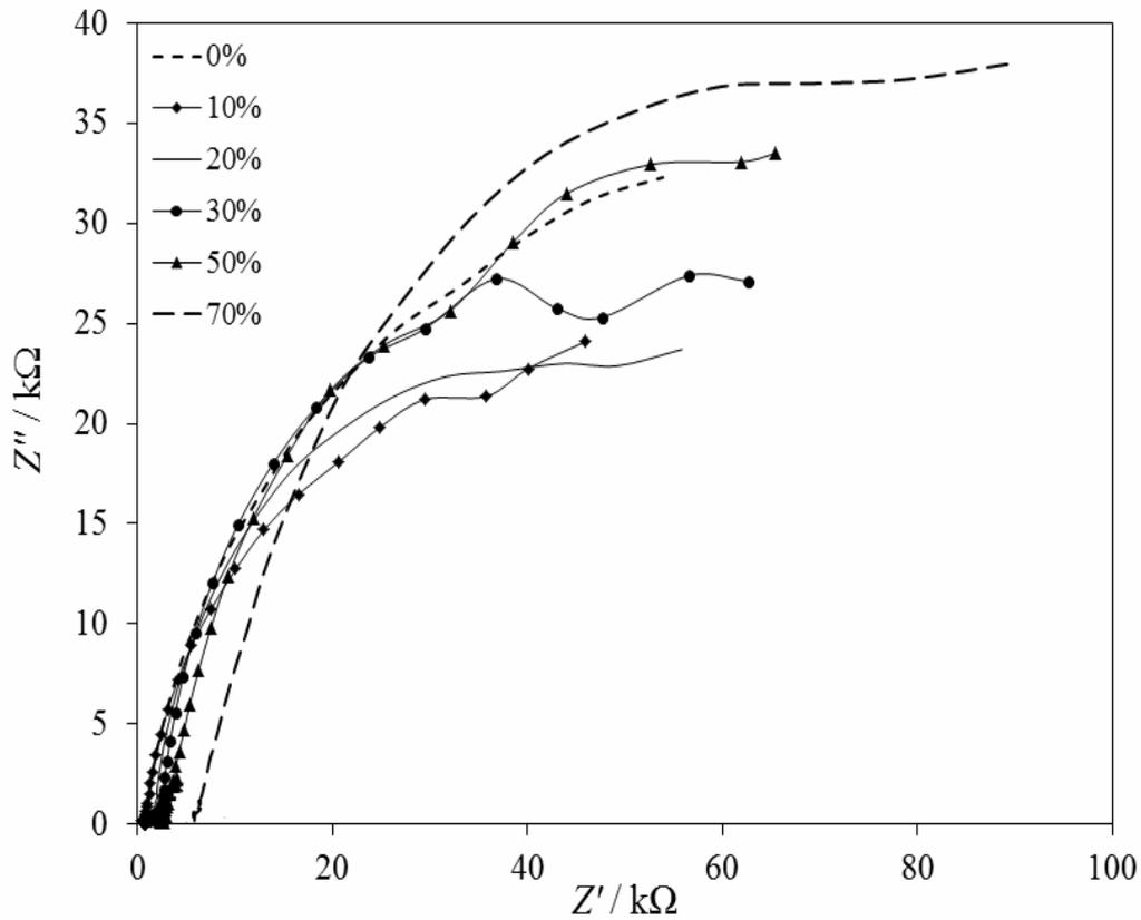
Fig. 4 – Nyquist diagrams of duplex steel alloy electrode in 100 ppm NaCl and ethylene glycol-water solution with different concentrations of ethylene glycol.
