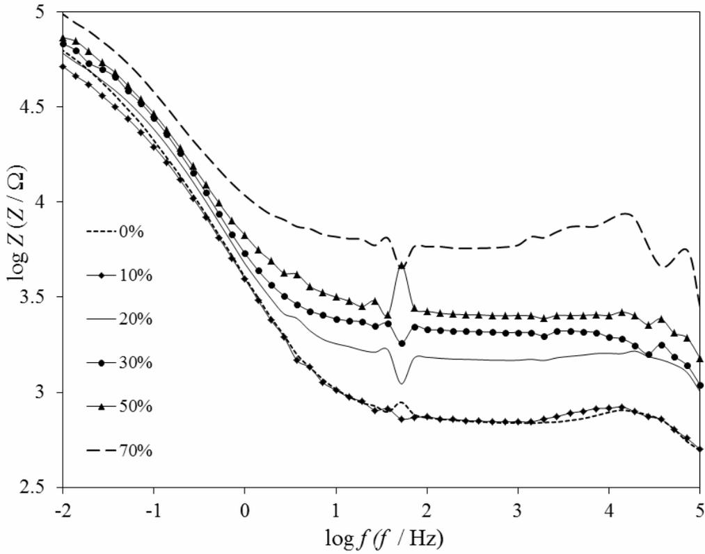
Fig. 3 – Bode diagrams of duplex steel alloy electrode in 100 ppm NaCl and ethylene glycol-water solution at different concentrations of ethylene glycol.
