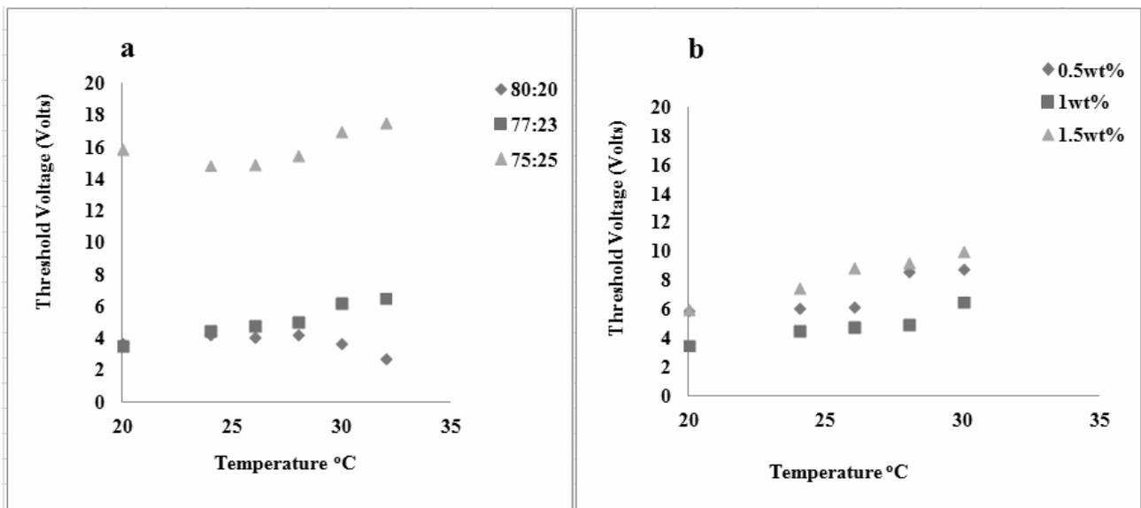
Fig. 3 – Electro-optical properties the threshold voltage of D-PDLC at various LC and dye compositions against varying the curing temperatures.
