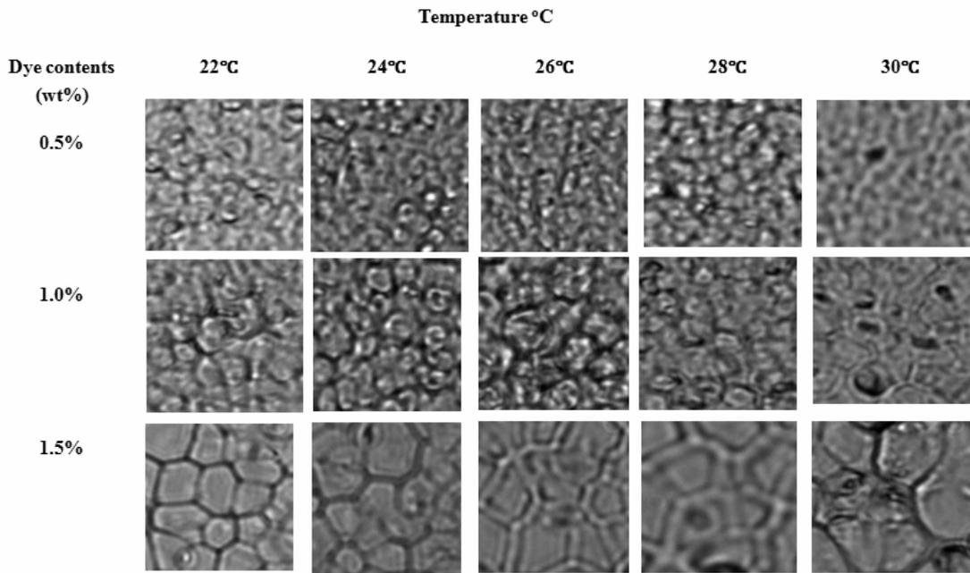
Fig. 2 – The POM images of dye doped PDLC fabricated with 77:23 wt% of LC/monomer while S428 compositions are remained as 0.5 wt%, 1 wt% and 1.5 wt% respectively.
