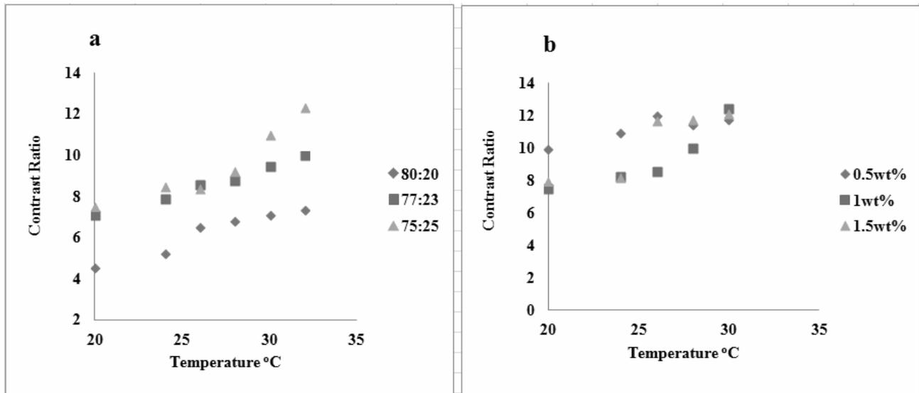
Fig. 4 – Electro-optical contrast of D-PDLC at various LC and dye concentrations against the varying temperatures.
