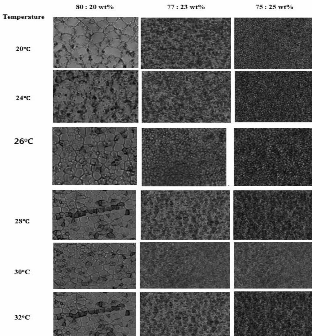
Fig. 1 – The surface morphologies of dye doped PDLC having 1 wt% of S428 dye with LC/monomer compositions as 80:20 wt%, 77:23 wt% and 75:25 wt% respectively.
