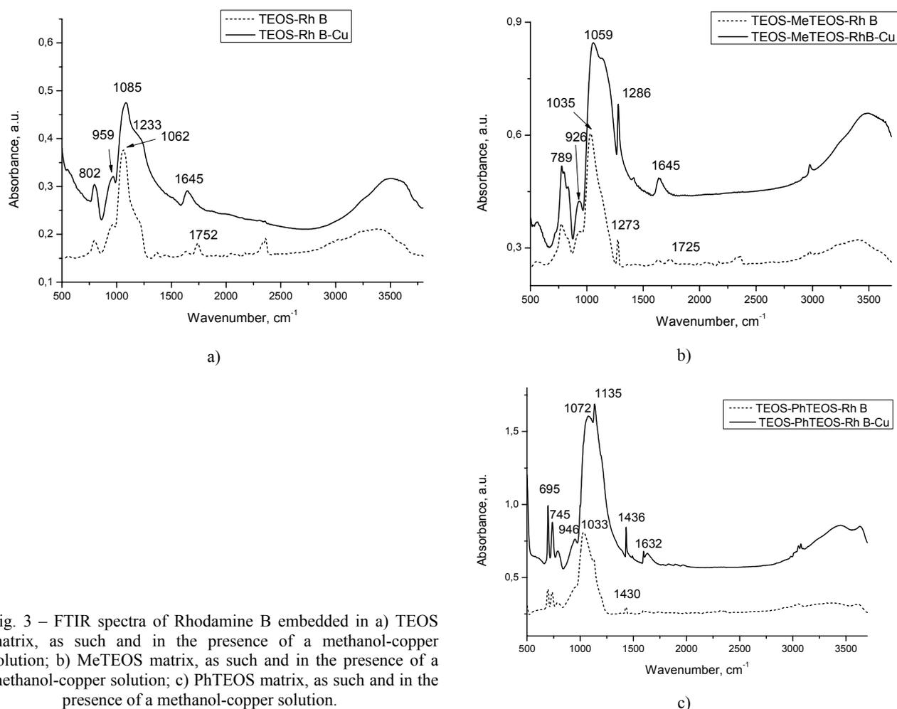
Fig. 3 – FTIR spectra of Rhodamine B embedded in a) TEOS matrix, as such and in the presence of a methanol-copper solution; b) MeTEOS matrix, as such and in the presence of a methanol-copper solution; c) PhTEOS matrix, as such and in the presence of a methanol-copper solution.
