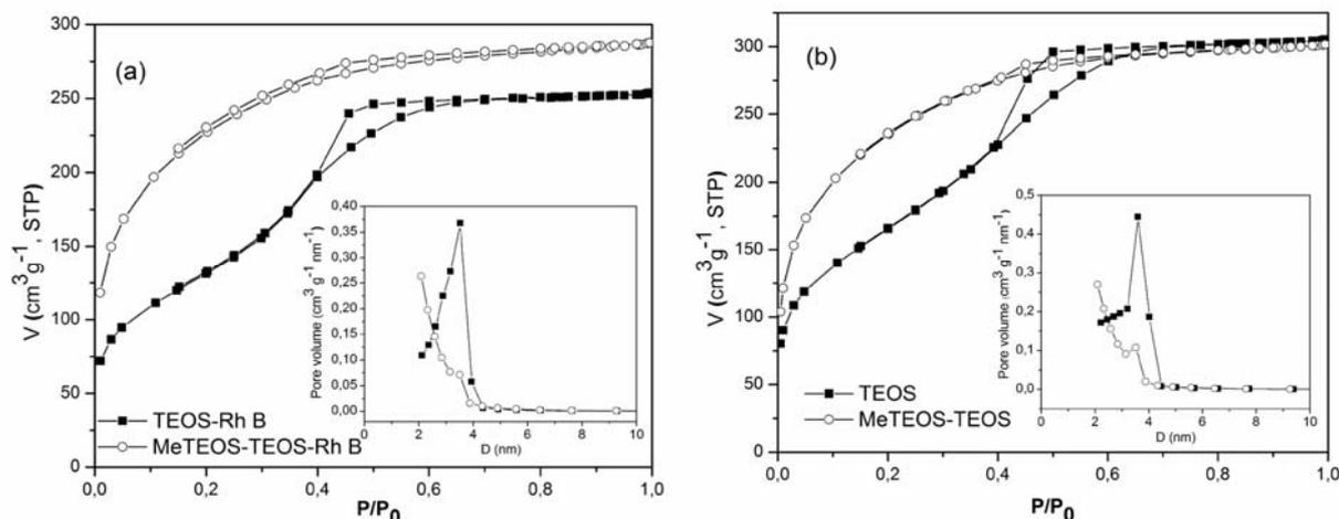
Fig. 2 –  $\text{N}_2$  adsorption-desorption isotherms of (a) TEOS-RhB, MeTEOS-TEOS-RhB; (b) TEOS, MeTEOS-TEOS (inset – the corresponding PSD graphs).
