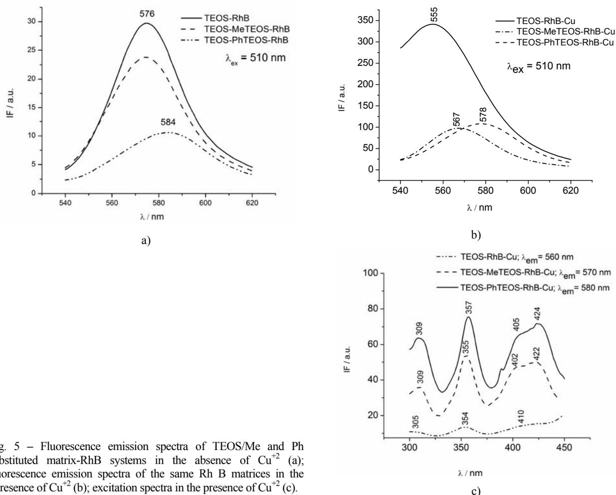
Fig. 5 – Fluorescence emission spectra of TEOS/Me and Ph substituted matrix-RhB systems in the absence of  $\text{Cu}^{+2}$  (a); fluorescence emission spectra of the same Rh B matrices in the presence of  $\text{Cu}^{+2}$  (b); excitation spectra in the presence of  $\text{Cu}^{+2}$  (c).
