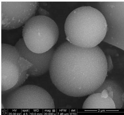
Fig. 4 – Micrograph of the composite TEOS-PhTEOS-Rh B-Cu powder.
