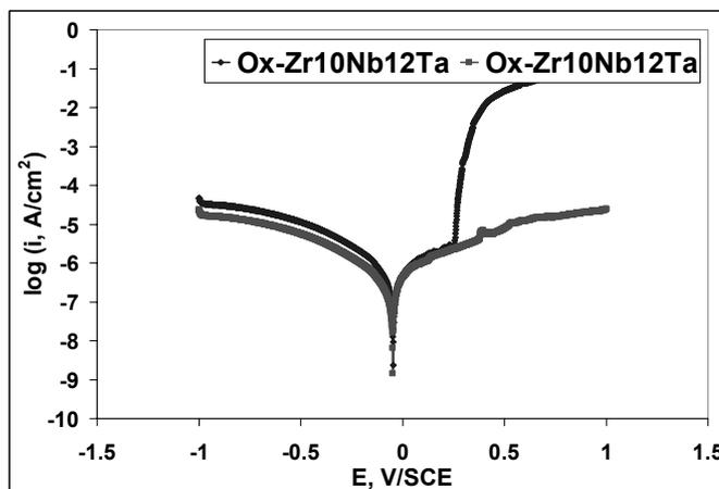
Fig. 2 – Potentiodynamic polarization curves for oxidized ZrNbTa ternary alloys.
