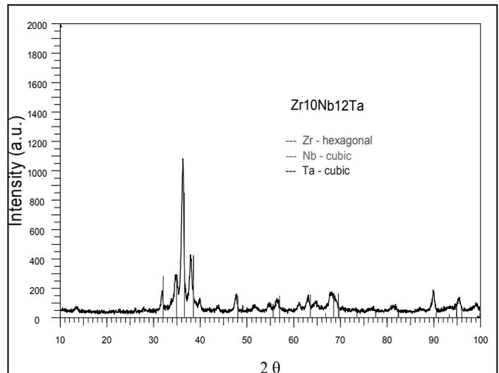
Fig. 8 – XRD pattern of Zr<sub>10</sub>Nb<sub>12</sub>Ta sample.
