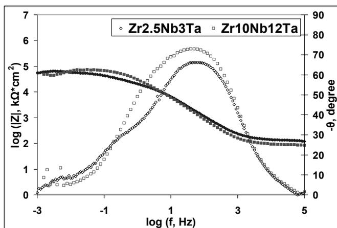
Fig. 5 – Bode diagrams for ZrNbTa ternary alloys.
