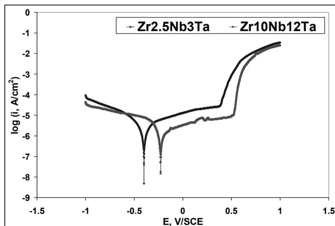
Fig. 1 – Potentiodynamic polarization curves for ZrNbTa ternary alloys.
