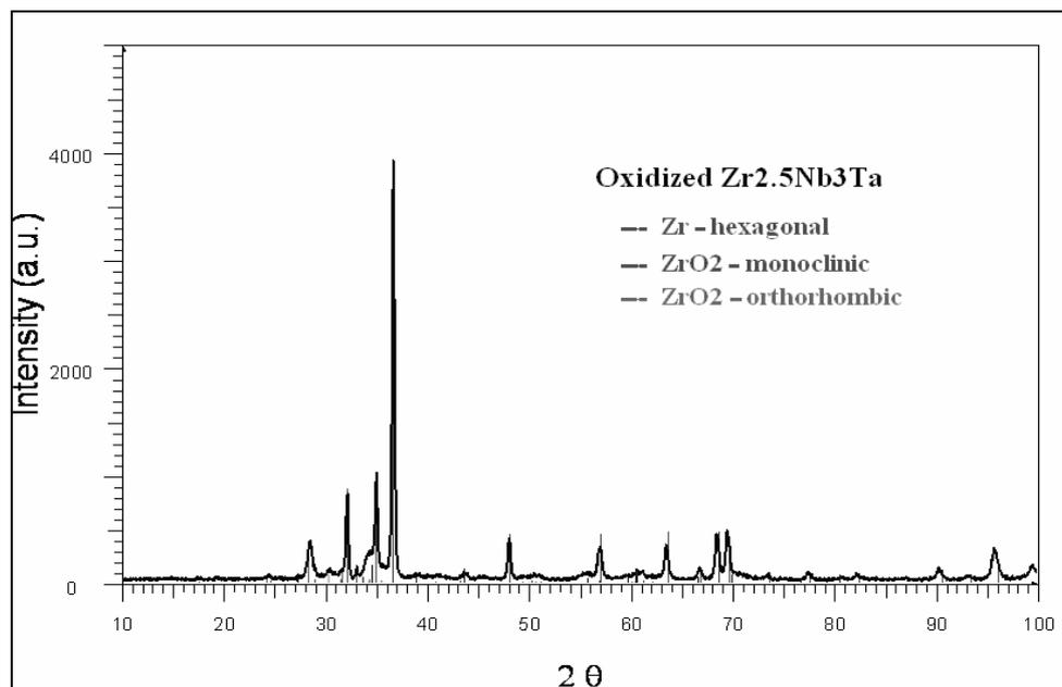
Fig. 9 – XRD pattern of Ox-Zr<sub>2.5</sub>Nb<sub>3</sub>Ta sample.
