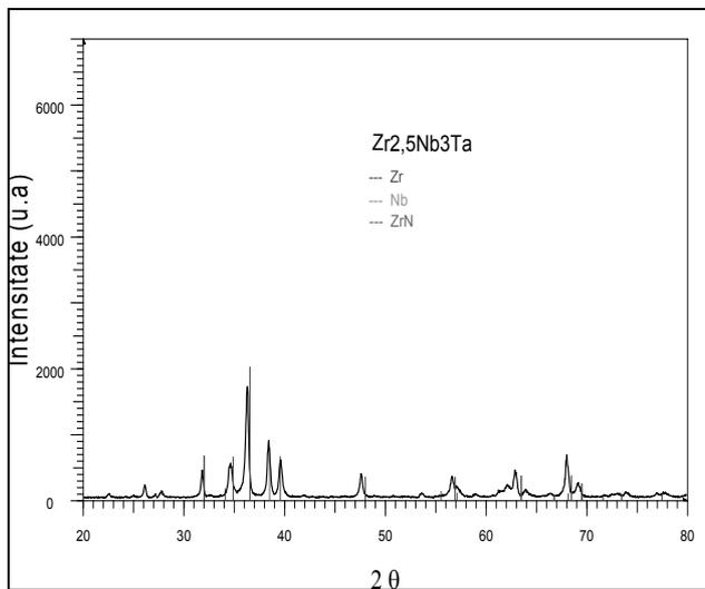
Fig. 7 – XRD pattern of Zr<sub>2.5</sub>Nb<sub>3</sub>Ta sample.
