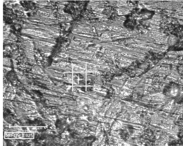
Fig. 13 – Vickers microhardness of Ox-Zr<sub>2.5</sub>Nb<sub>3</sub>Ta sample.
