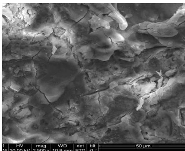
Fig. 11 – SEM micrograph of Ox-Zr<sub>10</sub>Nb<sub>12</sub>Ta sample.
