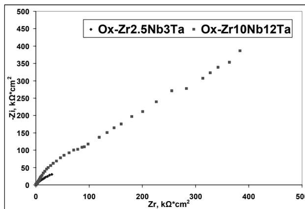
Fig. 4 – Nyquist diagrams for oxidized ZrNbTa ternary alloys.
