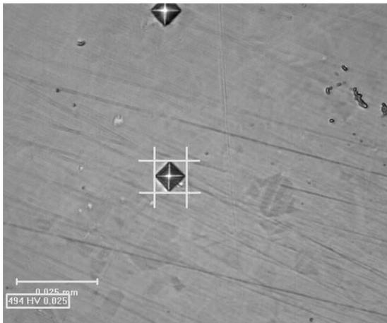
Fig. 14 – Vickers microhardness of Ox-Zr<sub>10</sub>Nb<sub>12</sub>Ta sample.
