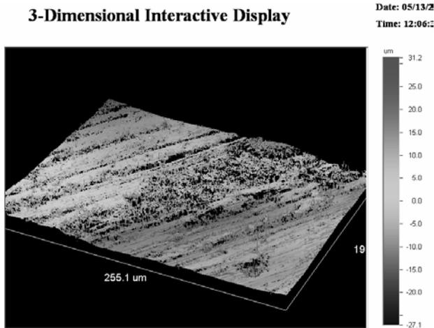
Fig. 16 – 3D profile of Ox-Zr<sub>2.5</sub>Nb<sub>3</sub>Ta sample.
