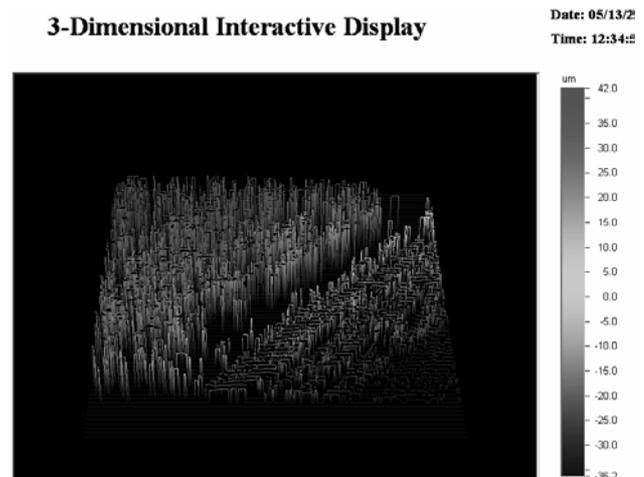
Fig. 17 – 3D profile of Ox-Zr<sub>10</sub>Nb<sub>12</sub>Ta sample.
