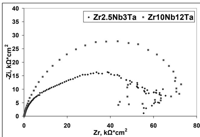
Fig. 3 – Nyquist diagrams for ZrNbTa ternary alloys.
