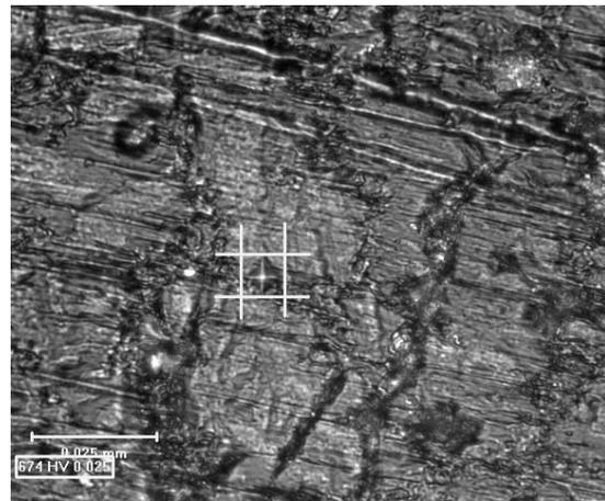
Fig. 15 – Vickers microhardness of Ox-Zr<sub>10</sub>Nb<sub>12</sub>Ta sample.
