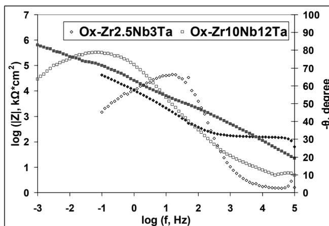
Fig. 6 – Bode diagrams for oxidized ZrNbTa ternary alloys.
