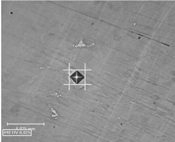
Fig. 12 – Vickers microhardness of Zr<sub>2.5</sub>Nb<sub>3</sub>Ta sample.
