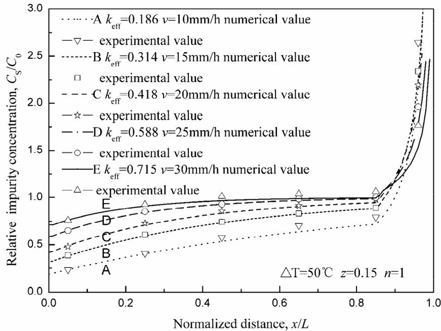
Fig. 5 – The comparison of zone melting rate between experimental and numerical value.
