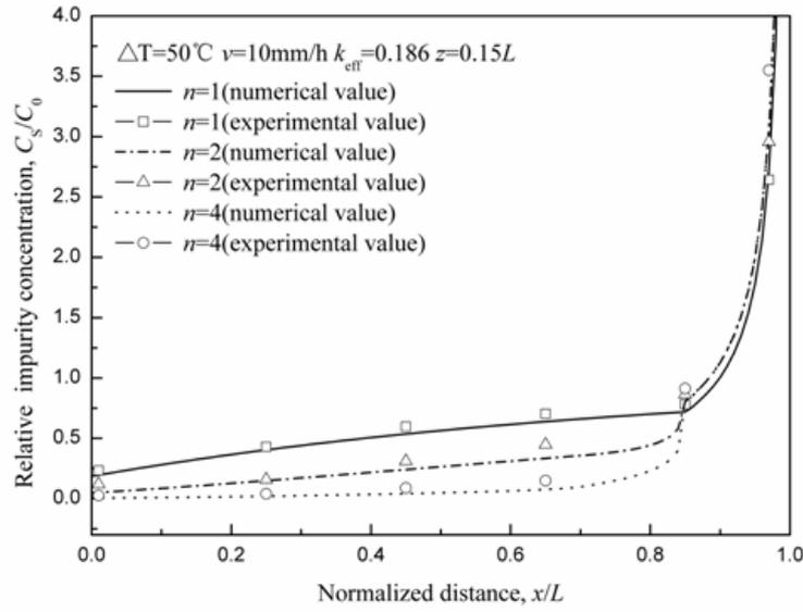
Fig. 6 – The comparison of zone passing times between experimental and numerical value.
