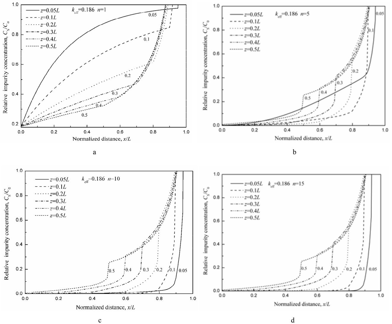
Fig. 7 – Concentration distribution of impurity 2, 6-TDI with different molten zone lengths. Zone melting passing times: a,  $n = 1$ ; b,  $n = 5$ ; c,  $n = 10$ ; d,  $n = 15$ .
