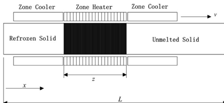
Fig. 3 – Schematic diagram of the principle of zone melting.
