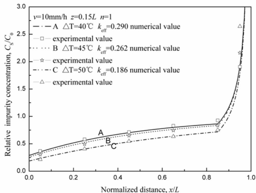
Fig. 4 – The comparison of temperature difference between experimental and numerical value.
