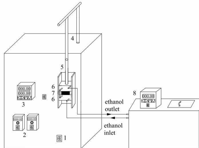
Fig. 2 – Schematic diagram of experimental apparatus of zone melting
