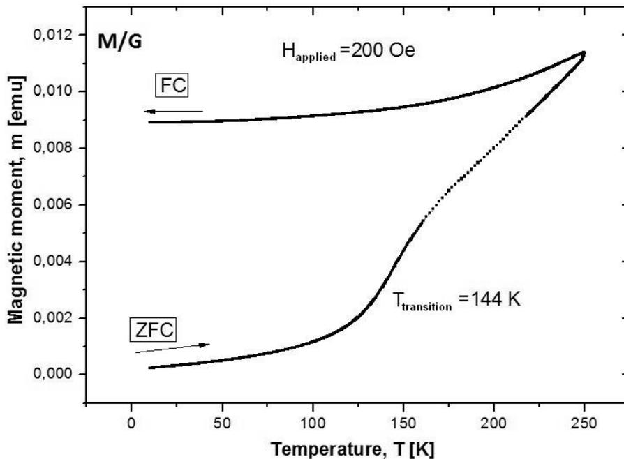
Fig. 5 – Thermomagnetic curves (temperature dependence of magnetization measured using standard zero field cooling (ZFC) and field cooling (FC) procedure) for M/G.
