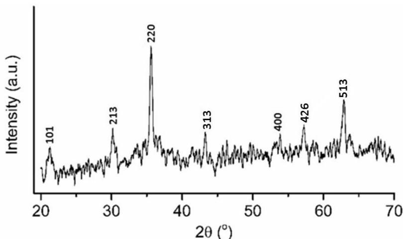
Fig. 3 – Diffraction pattern of M/G composite.
