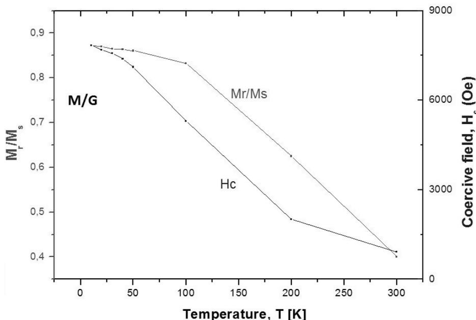
Fig. 6 – Dependence of remanent magnetization/saturation magnetization ratio ( $M_r/M_s$ ) and of coercive field on temperature for M/G composite sample.
