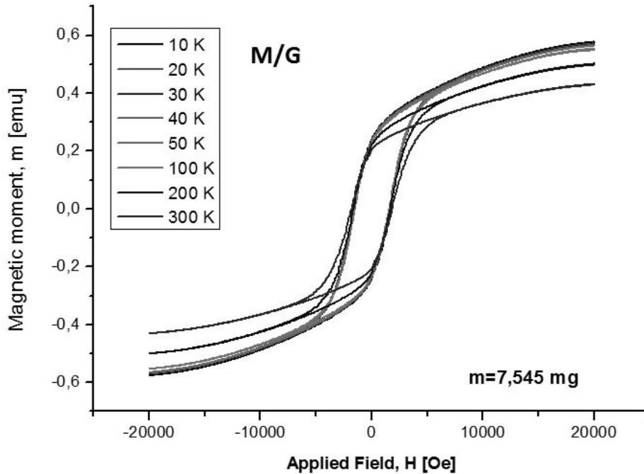
Fig. 4 – Evolution of the magnetic hysteresis curves for M/G composites as a function of temperature.
