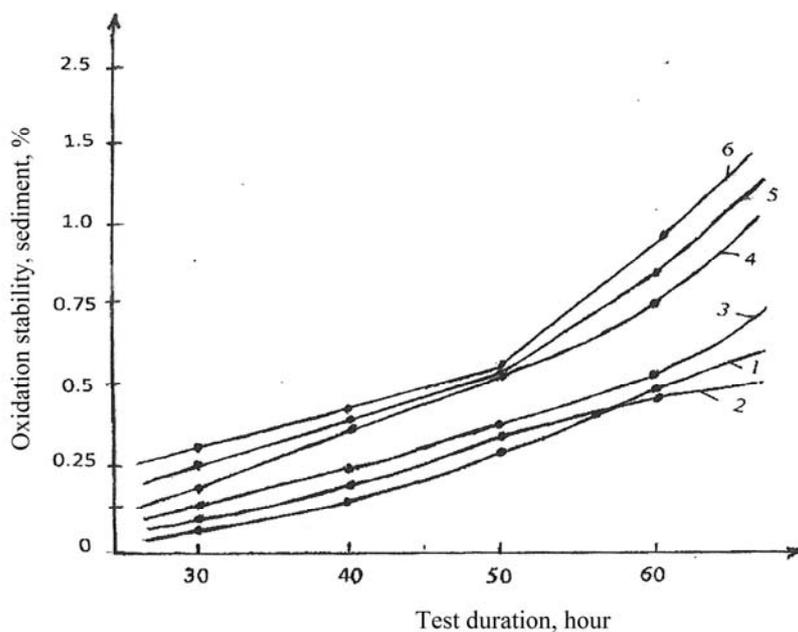
Fig. 5 – Dependence of the resistance of M-14G<sub>2</sub> oil to oxidation with 5% additive on oxidation test duration
