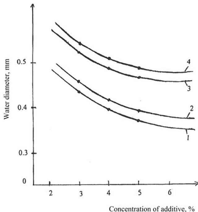
Fig. 4 – Dependence of wear resistance of M-8 oil on 3.5% concentration of the additive:
