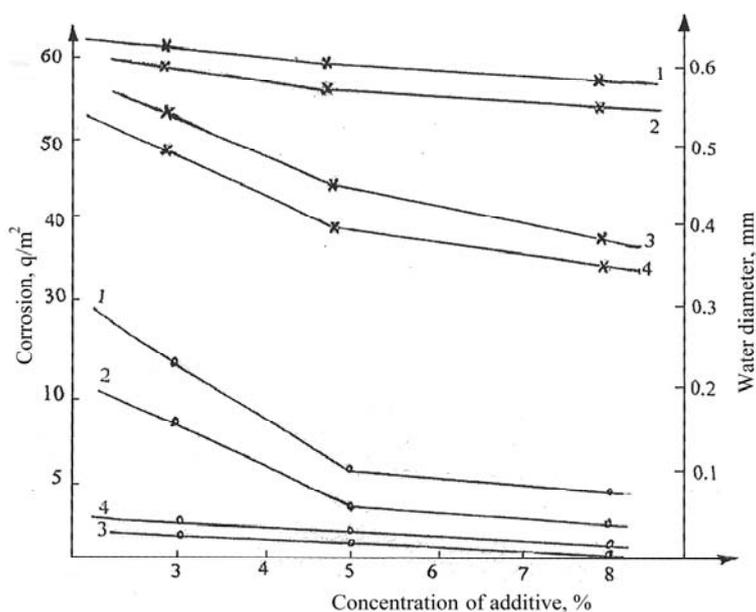
Fig. 3 – Dependence of wear and corrosion resistance of the additives on their concentration in M-8 oil 1-IXP-109, 2-IXP-115, 3-AKI-208, 4-AKI-209. --x---x---wear resistance ; ---o---o--- corrosion resistance.
