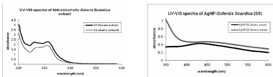
Fig. 3 – UV-VIS spectra of a) *Sideritis Scardica* extract and b) silver nanoparticle AgNP-SS samples.
