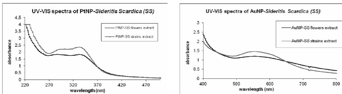
Fig. 4 – UV-VIS spectra of a) platinum nanoparticles PtNP-SS and b) gold nanoparticles AuNP-SS samples.
