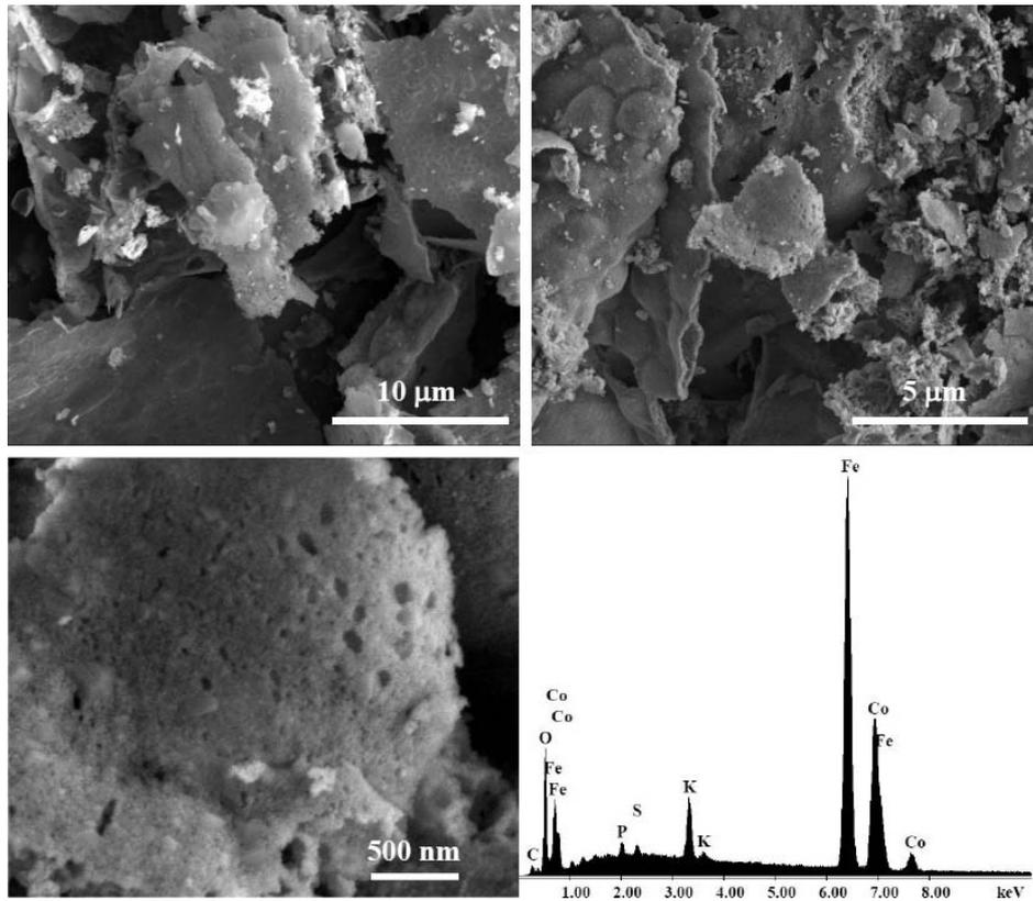
Fig. 3 – SEM micrographs, at different magnifications, and EDX spectrum of the sample **G-800** obtained by self-combustion using ginger root extract and calcined at 800 °C/1h.
