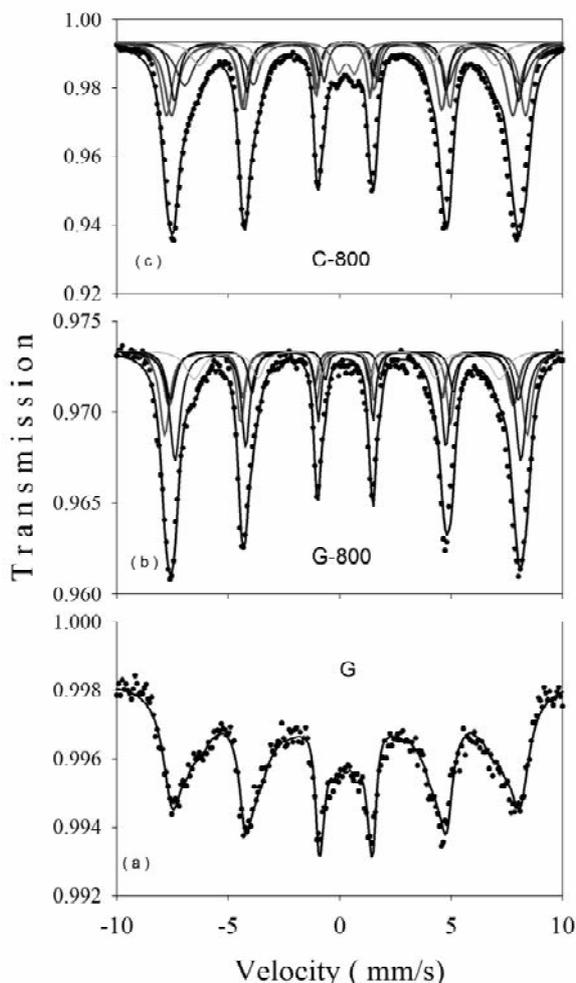
Fig. 5 – Mössbauer spectra of the synthesized cobalt ferrite samples: (a) G, (b) G-800, (c) C-800. Continuous lines represent the fit with experimental points.
