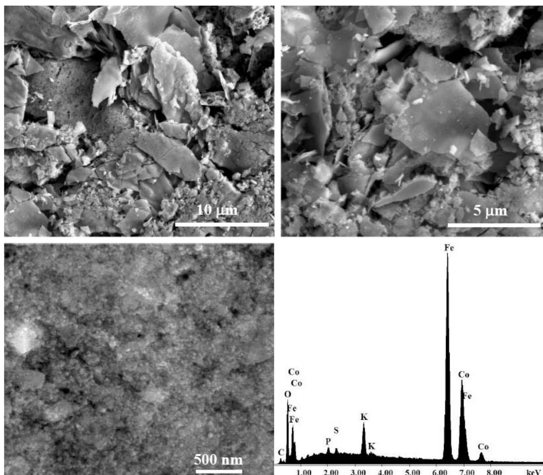
Fig. 2 – SEM micrographs, at different magnifications, and EDX spectrum of the sample **G** obtained by self-combustion using ginger root extract.
