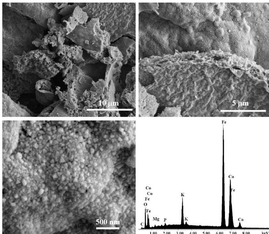
Fig. 4 – SEM micrographs, at different magnifications, and EDX spectrum of the sample **C-800** obtained by self-combustion using cardamom seeds extract, calcined at 800 °C/1h.
