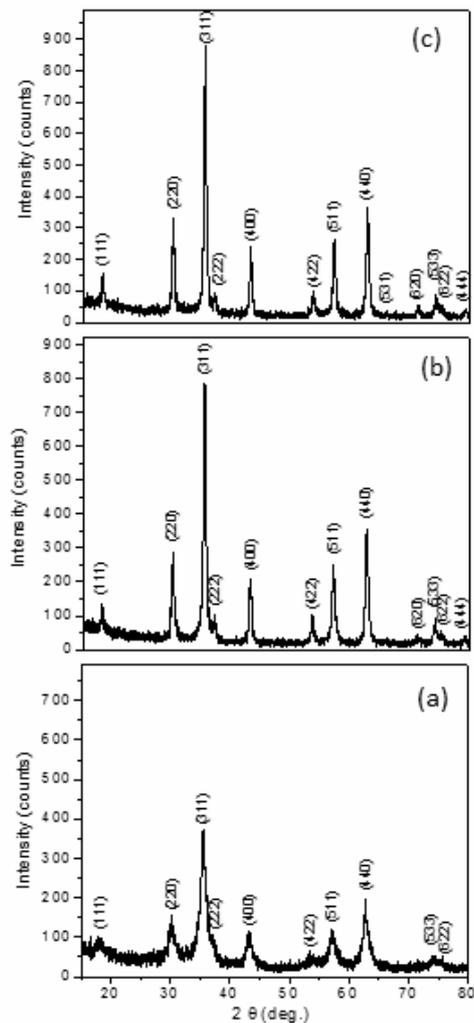
Fig. 1 – X-ray diffraction of the cobalt ferrites obtained by self-combustion using ginger root/cardamom seed extracts: (a) G, (b) G-800, (c) C-800.
