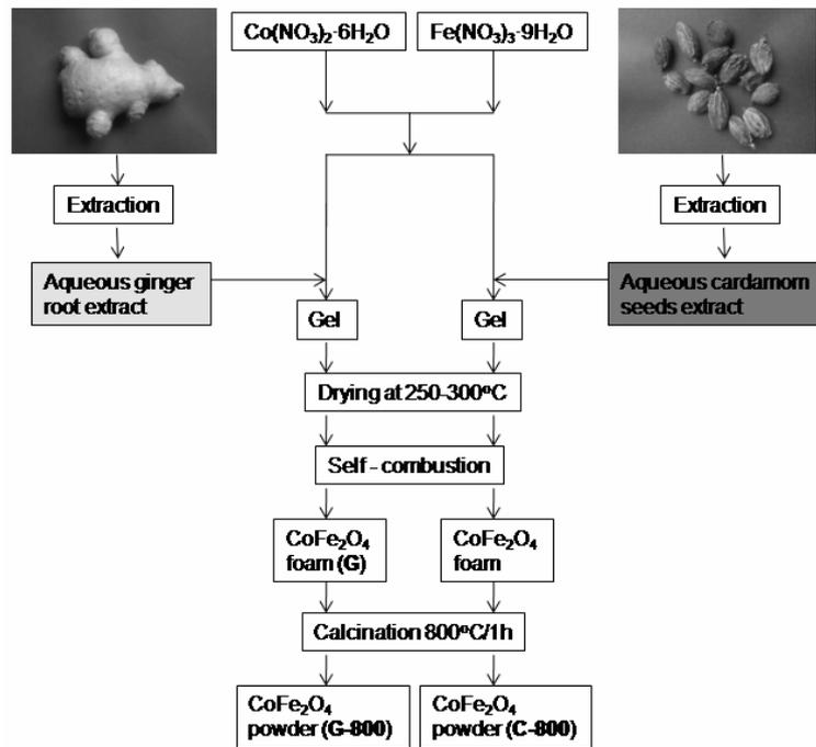
Scheme 1 – Overall description for the preparation of  $\text{CoFe}_2\text{O}_4$  through green synthesis method.
