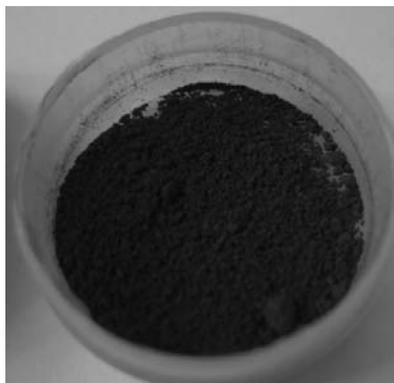
Fig. 1 – NiFe<sub>2</sub>O<sub>4</sub>/kaolinite composite heat treated up to 500°C.
