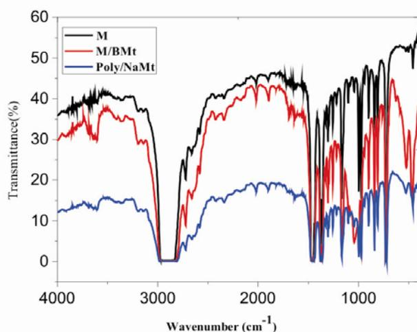
Fig. 4 – Variation of IR transmittance (%) of M, M/BMt and Poly/ NaMt.
