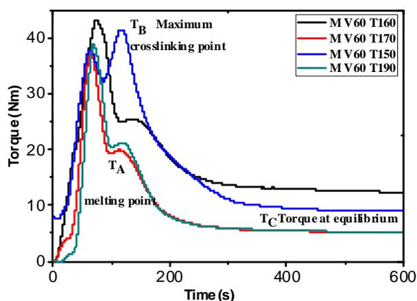
Fig. 2 – Variation of the torque *versus* time for (PP/HDPE/MAH) at different temperatures.
