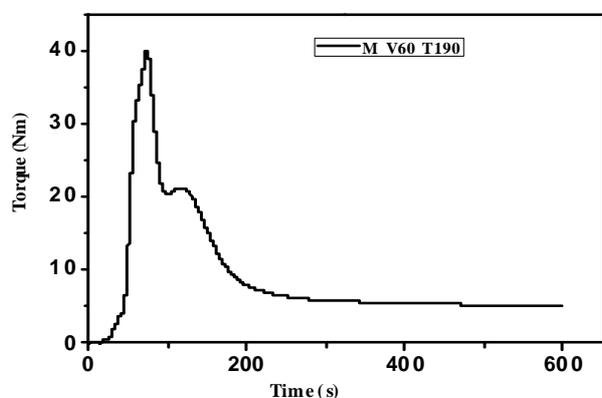
Fig. 1 – Variation of the torque *versus* time for PP/HDPE/MAH at (60 rpm and 190°C).
