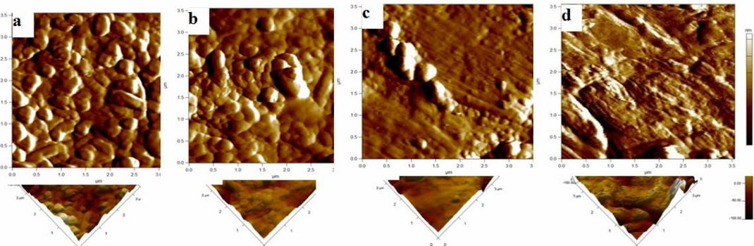
Fig. 7 – AFM topographic images of: a) M, b) Poly/NaMt, c) M/BMt, d) M/BMt/TiO<sub>2</sub>.
