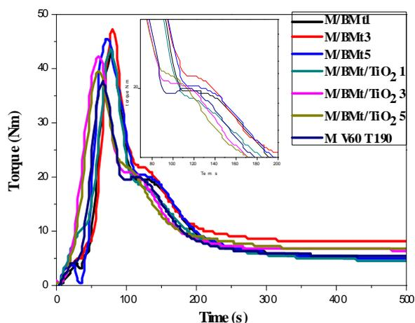
Fig. 3 – Variation of the torque *versus* time for (M, M/BMt 1, 3, 5 M/BMt/TiO<sub>2</sub> 1, 3, 5) at 180 °C.
