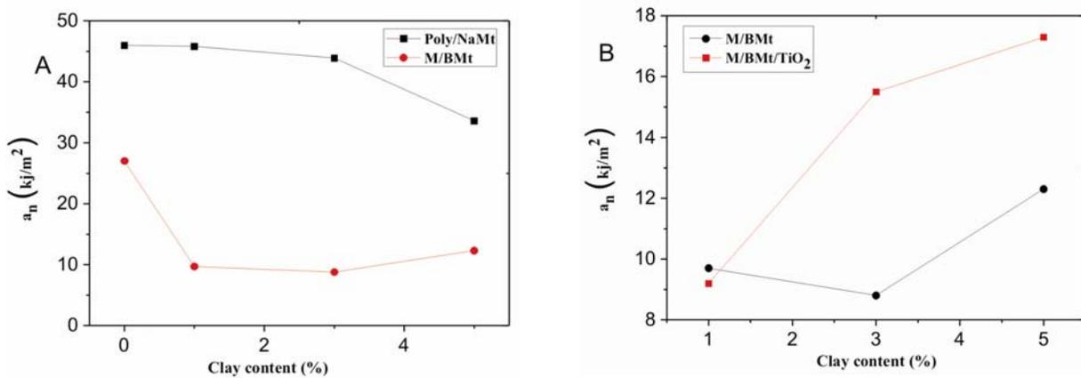
Fig. 9 – Impact strength for Poly/NaMt, M/BMt and M/BMt/TiO<sub>2</sub>.
