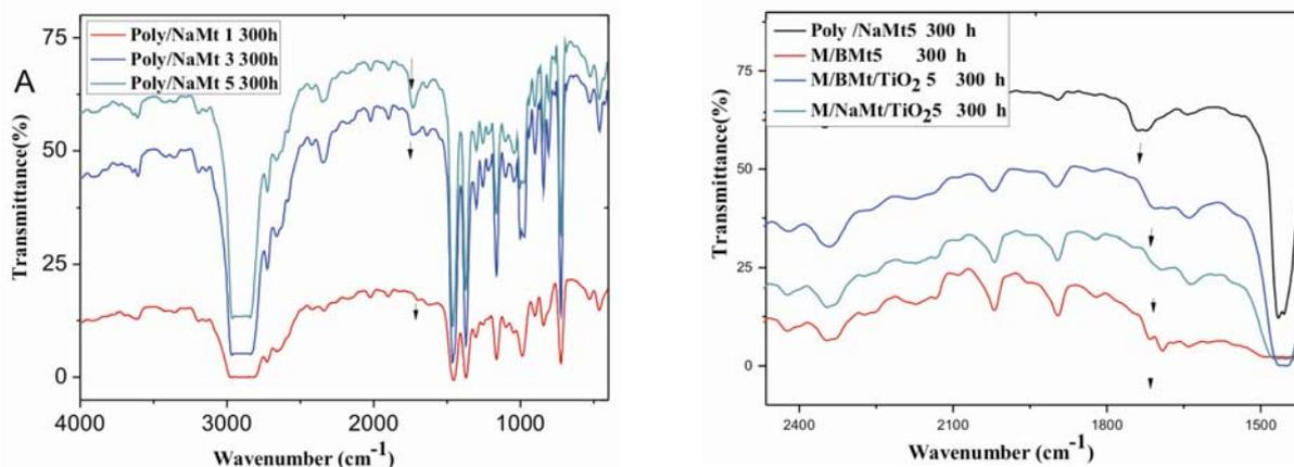
Fig. 10 – FTIR spectra for UV-irradiated; a: (poly/NaMt 1, 3, 5), b: (Poly/NaMt 5), (M/BMt 5) and (M/BMt/TiO<sub>2</sub> 5).
