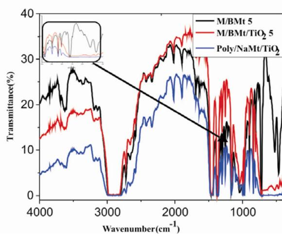
Fig. 5 – Variation of IR transmittance of M/BMt, M/BMt/TiO<sub>2</sub> 5 and Poly/NaMt/TiO<sub>2</sub> 5.
