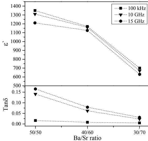
Fig. 5 – Room-temperature dielectric permittivity and losses of approximately 240 nm-thick BST 50/50, 40/60 and 30/70 thin films measured at 100 kHz, 10 GHz and 15 GHz. Lines are guides to the eye.
