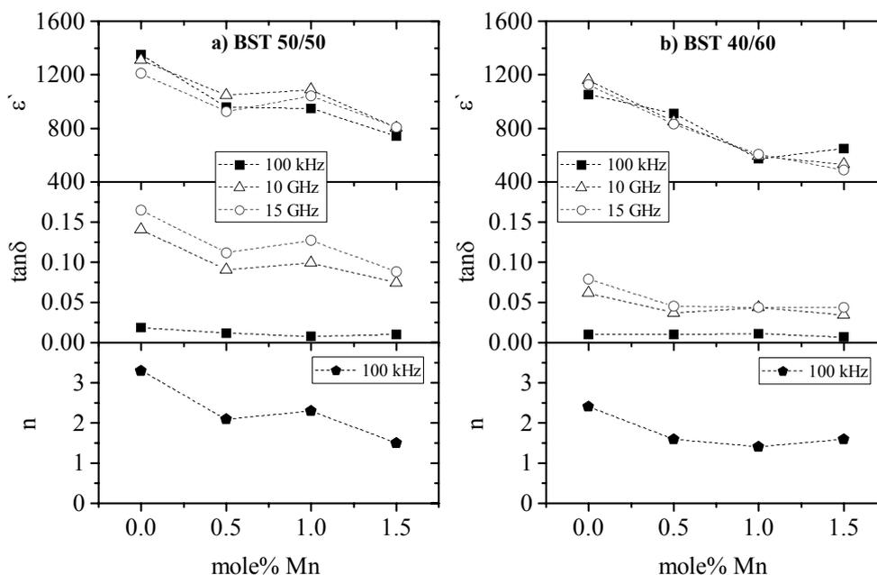
Fig. 9 – Dielectric permittivity ( $\epsilon'$ ), dielectric losses ( $\tan\delta$ ) and tunability ( $n$ ) of undoped and doped a) BST 50/50 and b) BST 40/60 films, measured at 100 kHz, 10 GHz and 15 GHz. Tunability is expressed as the ratio of permittivities at 0 and 40 V.
