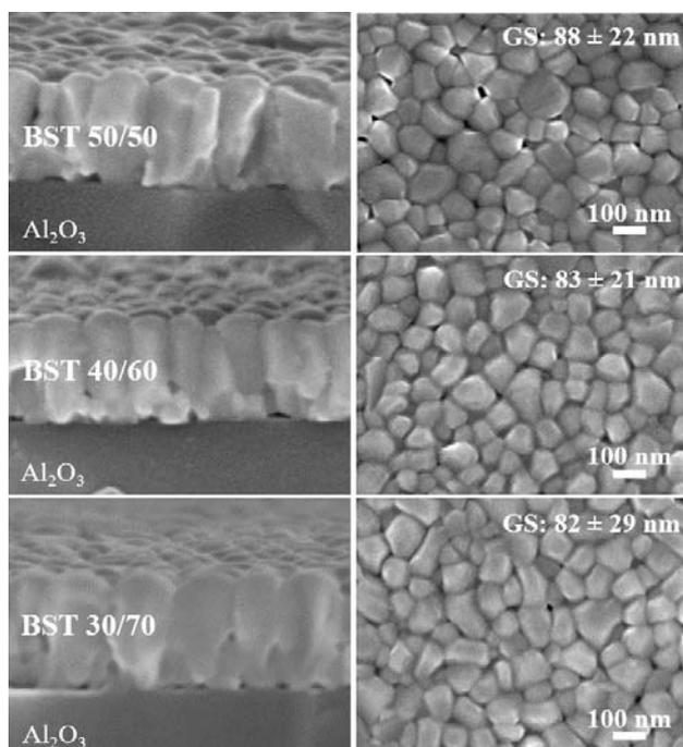
Fig. 4 – FE-SEM micrographs of the cross-section and plane-view microstructures with average grain sizes (GS) of approximately 240 nm-thick BST 50/50, 40/60 and 30/70 thin films on alumina substrates.
