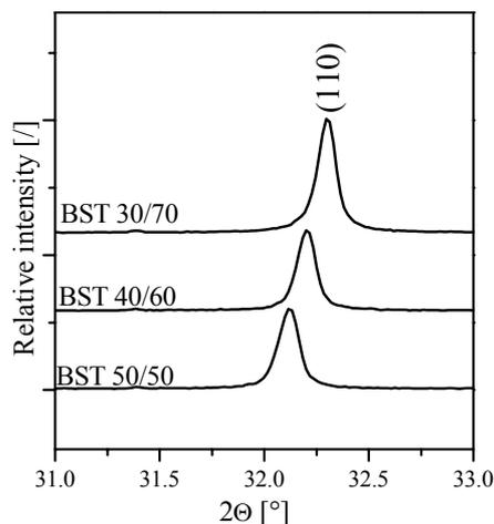
Fig. 3 – XRD patterns of BST films with different Ba/Sr molar ratios in a narrow  $2\theta$  range showing (110) peaks of the perovskite phase.
