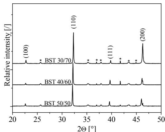
Fig. 2 – XRD patterns of BST 50/50, BST 40/60 and BST 30/70 thin films on alumina substrates. The peaks of alumina (JCPDS 01-081-226) were subtracted and are denoted by \*. The main reflections of the perovskite structure are indexed according to the reference for BST 50/50 (JCPDS 00-039-1395).
