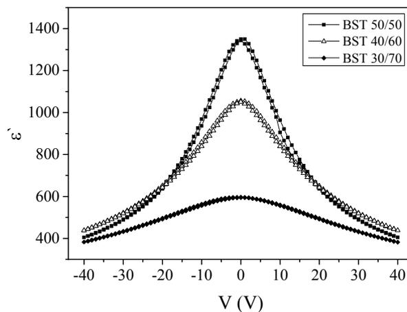
Fig. 6 – Voltage dependence of the dielectric permittivity measured at 100 kHz for BST 50/50, 40/60 and 30/70 thin films.
