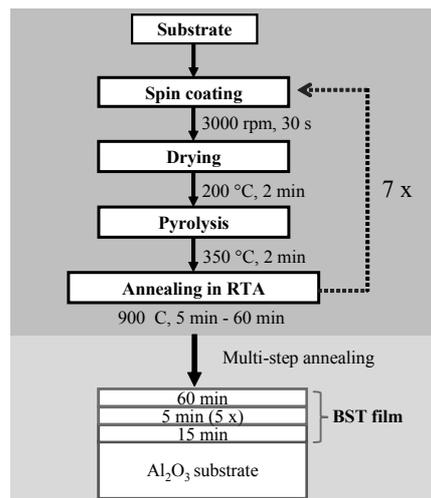
Fig. 1 – Schematic presentation of the thin-film deposition by multi-step annealing.
