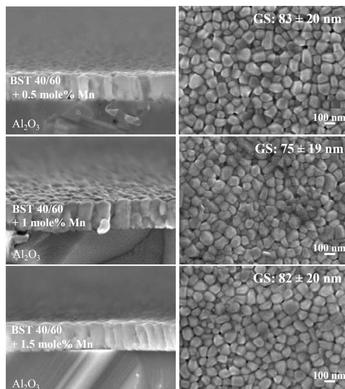
Fig. 8 – FE-SEM micrographs of the cross-section and plane-view microstructures of BST 40/60 thin films with 0 (already shown in Fig. 4), 0.5, 1.0 and 1.5 mole % Mn prepared on alumina substrates.
