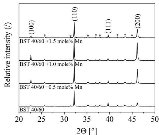
Fig. 7 – XRD patterns of BST 40/60 thin films with 0, 0.5, 1.0 and 1.5 mole % of Mn prepared on alumina substrates. \* - diffraction peaks of alumina substrate.
