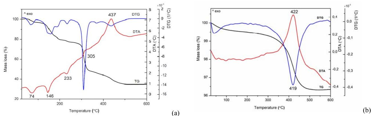
Fig. 1 – ATD, DTG and TG curves for the ZnO powders: as-prepared powder (a) and thermally treated at 400 °C (b).
