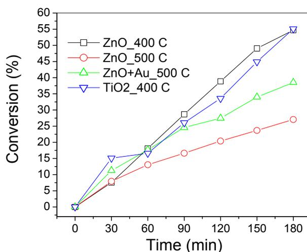
Fig. 8 – Comparative dye conversion under simulated solar light irradiation in the presence of the investigated powders.
