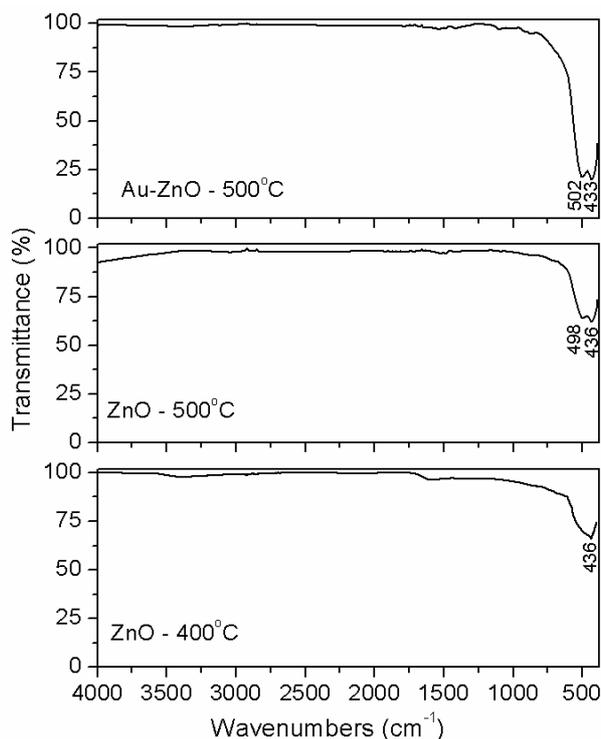
Fig. 2 – FTIR Spectra of ZnO and ZnO-Au powders.
