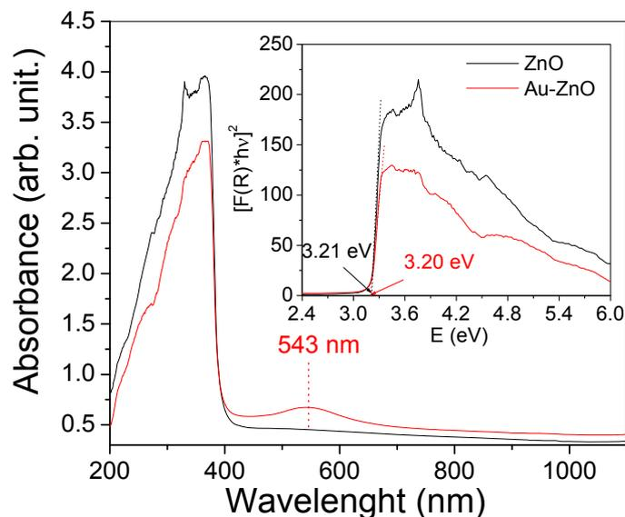
Fig. 5 – UV-VIS absorption spectra of the pristine and Au-modified ZnO powders thermally treated at 500 °C. Inset: The Kubelka-Munk plot of the same samples.
