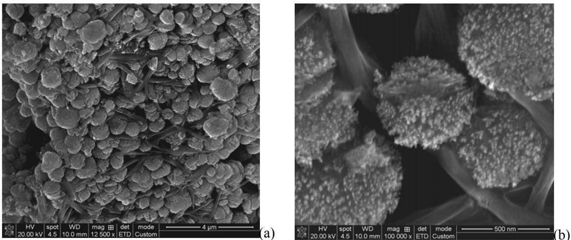
Fig. 4 – Morphology of ZnO powders treated at 400 °C at two different magnification scales: 12.5 k (a) and 100 k (b).
