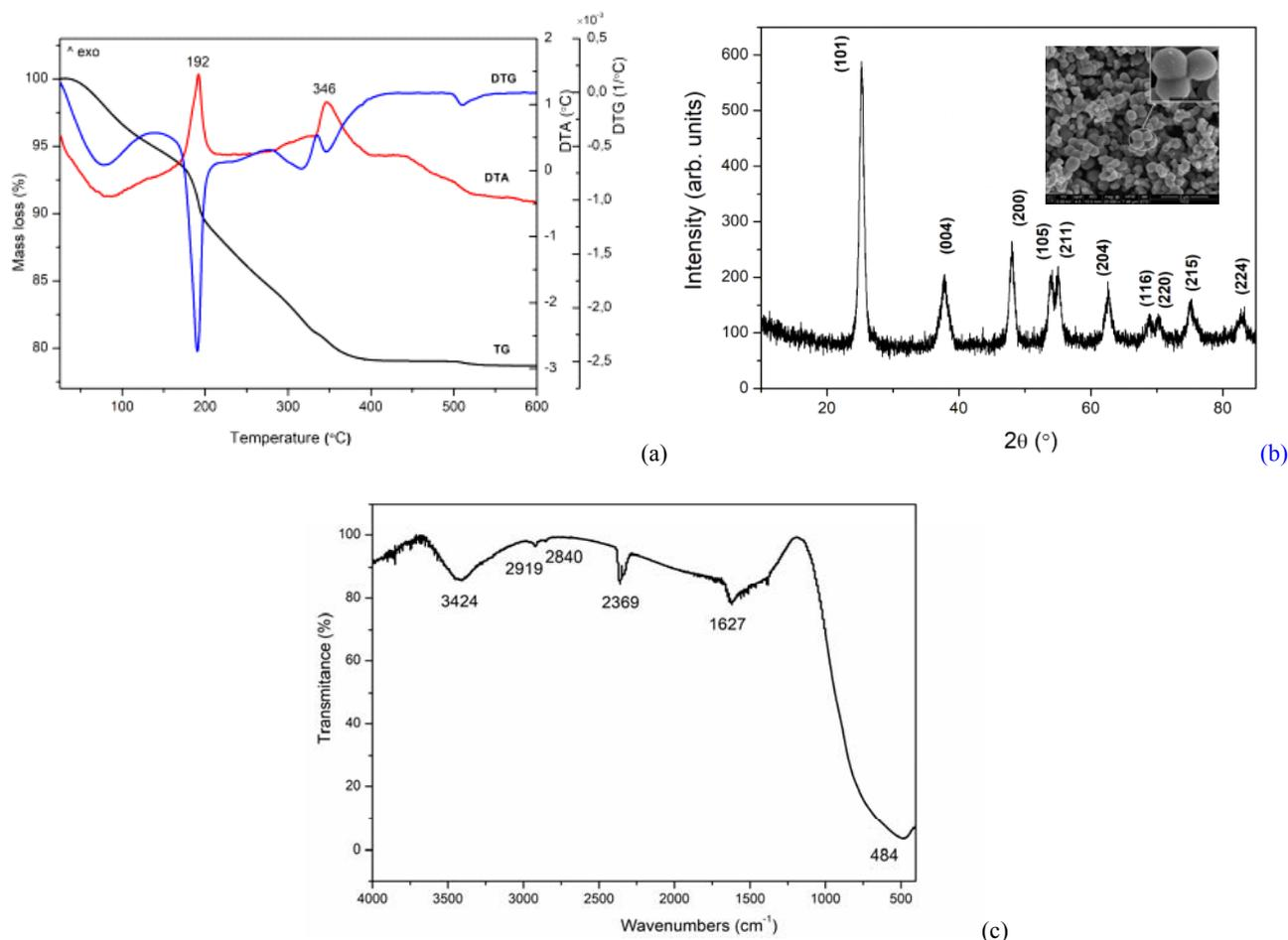
Fig. 6 – (a) ATD, DTG and TG curves for the TiO<sub>2</sub> gel (b) X-ray diffraction patterns of TiO<sub>2</sub> powder in the angular range of 2θ between 5 ° and 85 °; Inset: SEM images of the TiO<sub>2</sub> powder with anatase phase; the inset shows in detail the spherical shape of the constituent particles which have the tendency of merging (c) FT-IR spectra of the gel thermally treated at 400°C for 1 hour.
