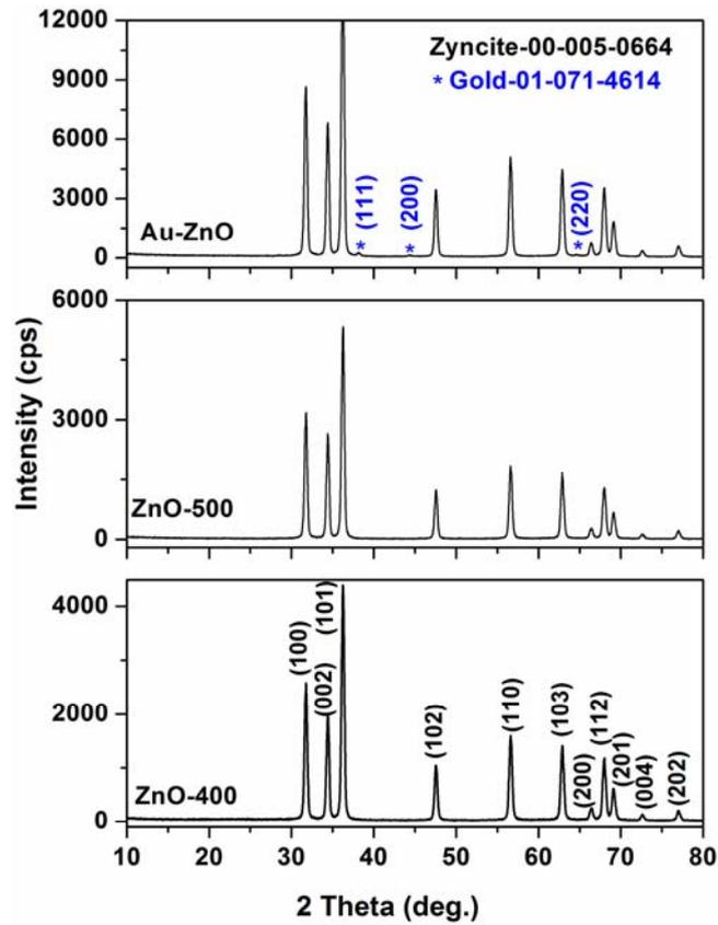
Fig. 3 – XRD patterns of the obtained samples.
