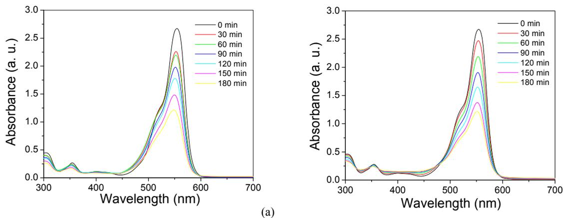
Fig. 7 – The photocatalytic activity of undoped TiO<sub>2</sub>-(a) and ZnO-(b), both calcined at 400 °C, tested in the RhB degradation reaction, followed by the absorbance decrease over time.
