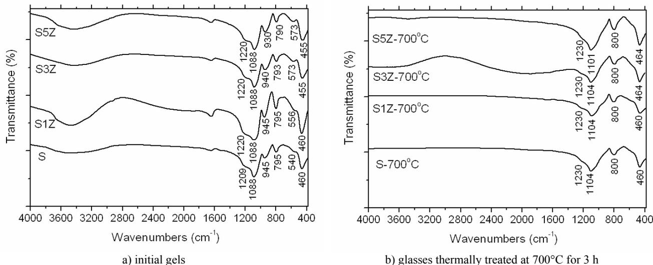
Fig. 2 – FTIR spectra of initial gels and thermally treated glasses.
