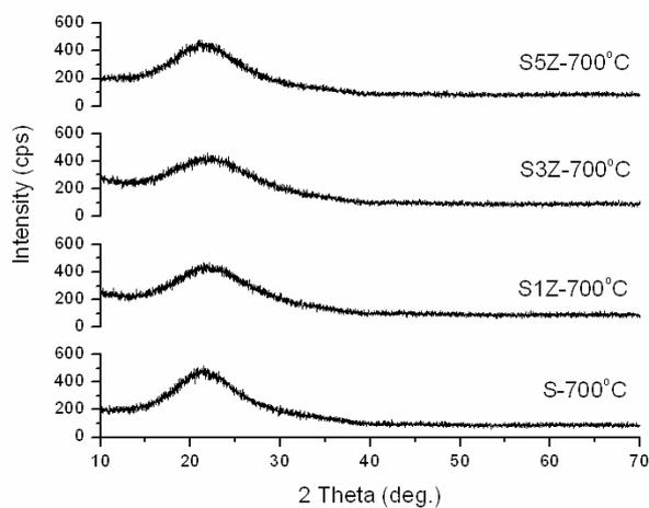
Fig. 3 –XRD patterns of the glasses treated at 700°C for 3h.
