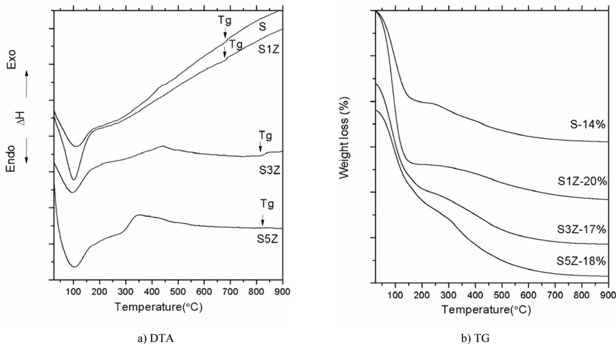
Fig. 1 – DTA/TG curves of initial gels.
