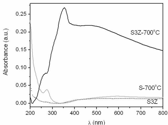
Fig. 4 – UV-VIS absorption spectra of the S3Z gel and S-700°C and S3Z-700°C glasses.
