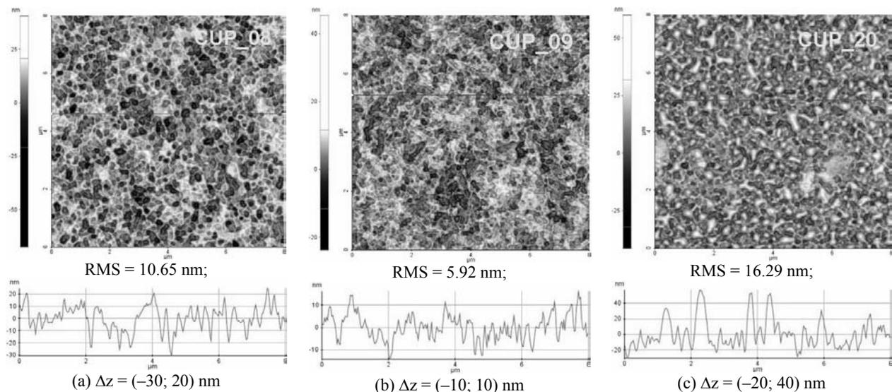
Fig. 3 – Two-dimensional characteristic AFM images together with arbitrary surface profiles (line scans).
