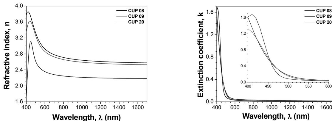
Fig. 7 – Dispersion of the refractive index ( $n$ ) and absorption coefficient ( $k$ ) of the  $\text{Cu}_2\text{O-Sr}$  films in the VIS-NIR spectral range.
