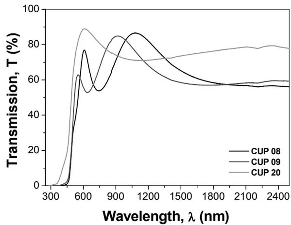
Fig. 11 – UV-VIS-NIR transmission spectra of the  $\text{Cu}_2\text{O-Sr}$  films.
