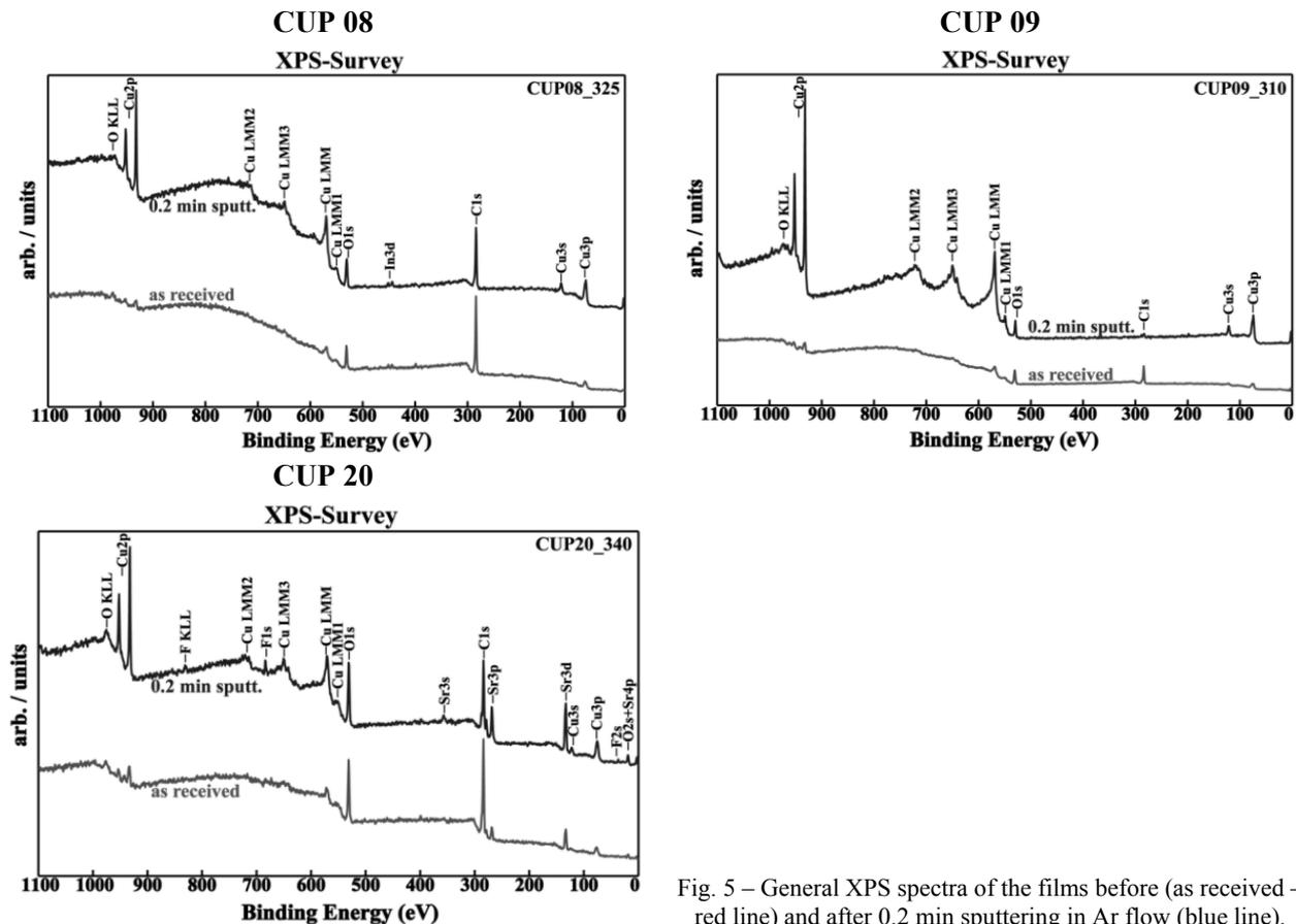
Fig. 5 – General XPS spectra of the films before (as received – red line) and after 0.2 min sputtering in Ar flow (blue line).
