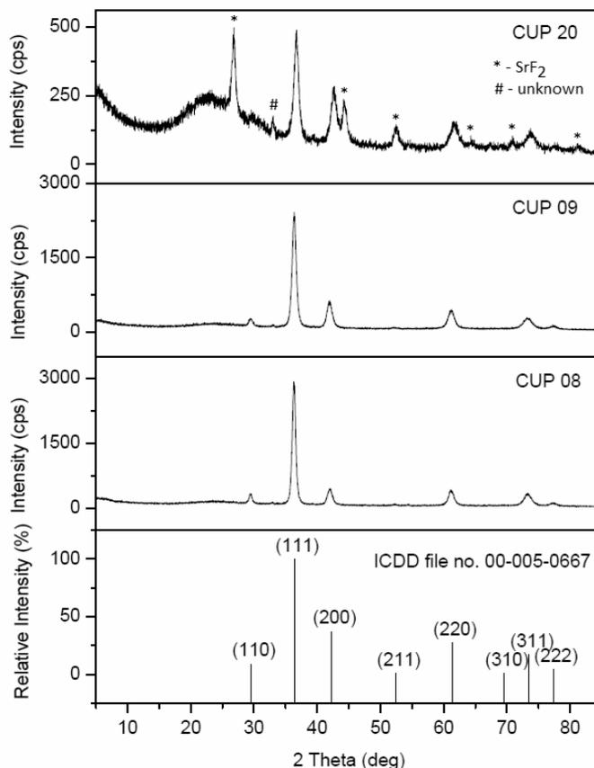
Fig. 1 – X-ray diffractograms of the Sr doped  $\text{Cu}_2\text{O}$  films compared with  $\text{Cu}_2\text{O}$  pattern (ICDD file no. 00-005-0667).
