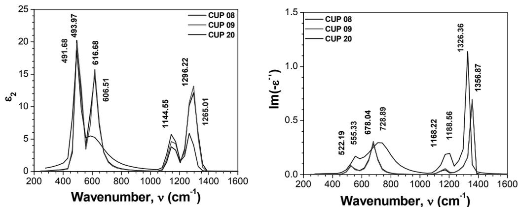
Fig. 9 – The imaginary part of dielectric function ( $\epsilon_2$ ) and dielectric loss function ( $\text{Im}-\epsilon^{-1}$ ) of  $\text{Cu}_2\text{O-Sr}$  films.
