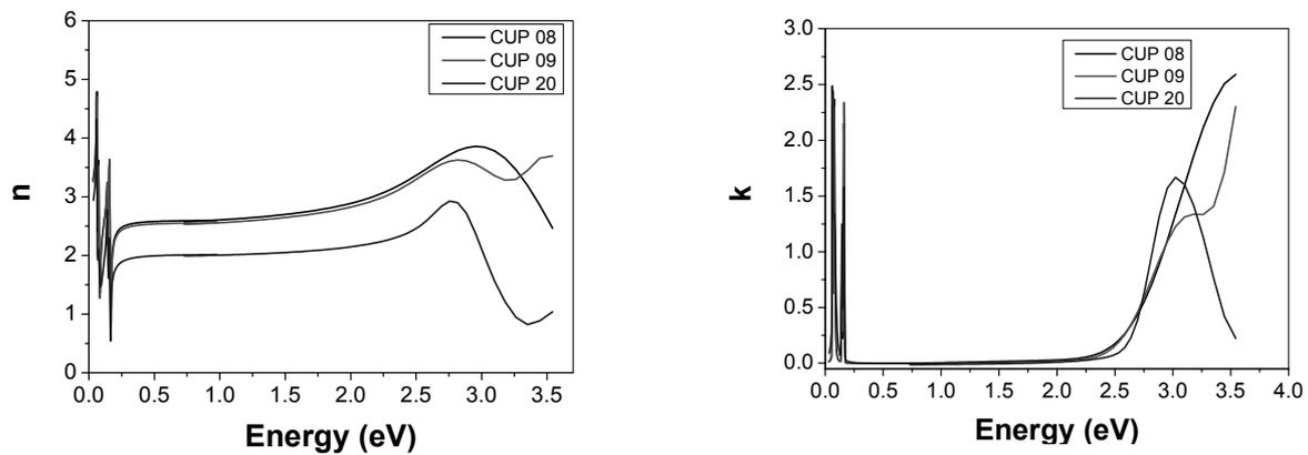
Fig. 10 – Dispersion of the refractive index ( $n$ ) and absorption coefficient ( $k$ ) of the  $\text{Cu}_2\text{O-Sr}$  films over a wide spectral range (0.7-3.5eV).
