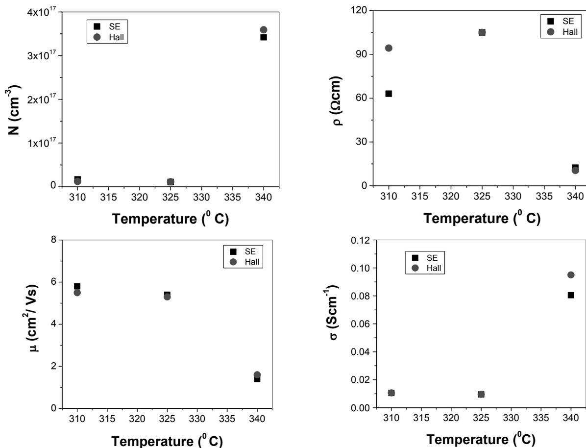
Fig. 8 – Comparison of the electrical parameters as obtained by SE and Hall methods.
