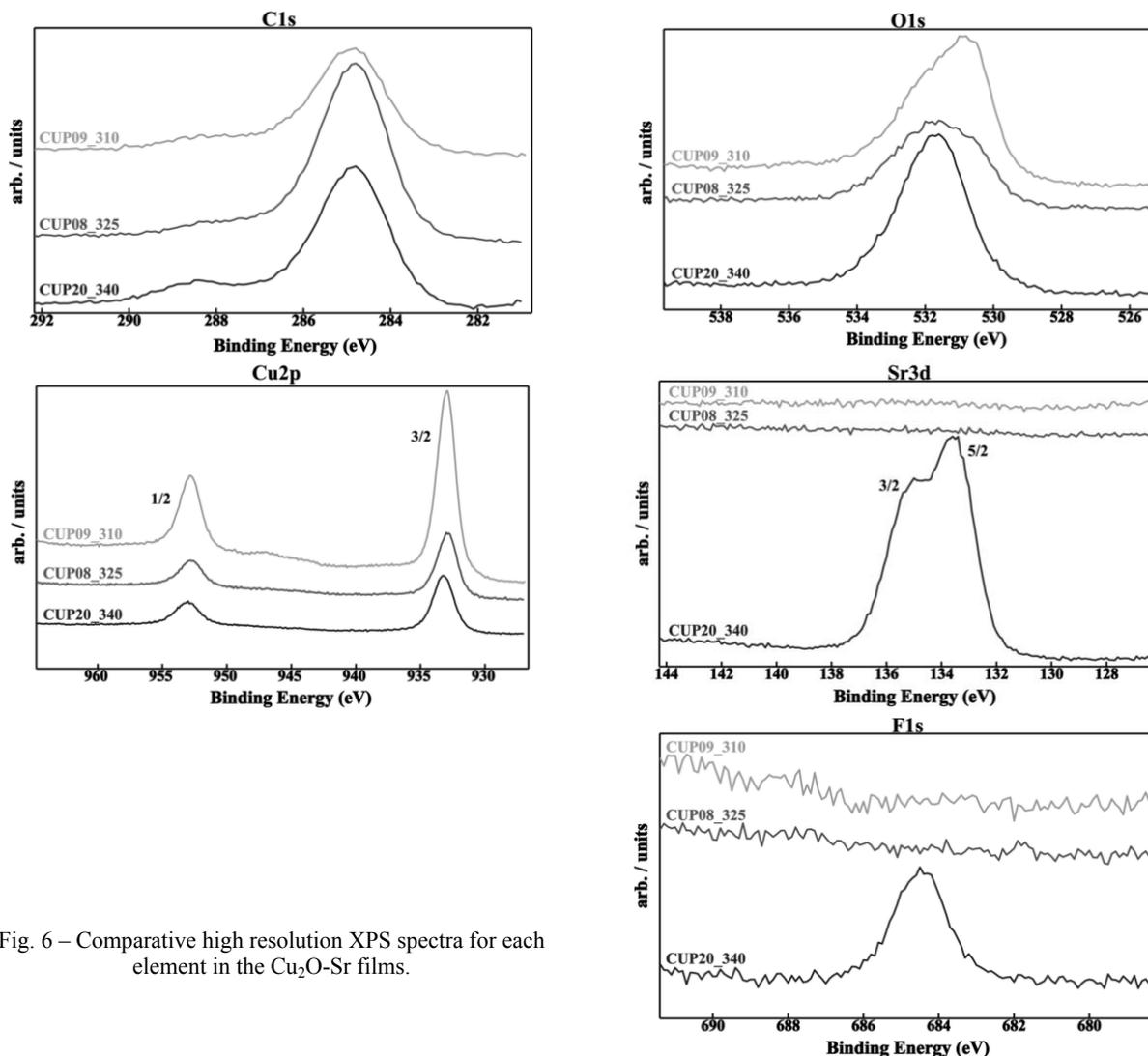
Fig. 6 – Comparative high resolution XPS spectra for each element in the  $\text{Cu}_2\text{O}$ -Sr films.
