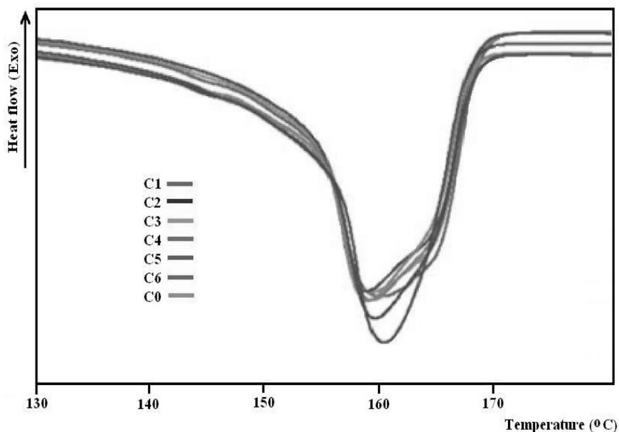
Fig. 3 – DSC scans on heating of the neat PP-g-MA (C0) and PP-g-MA – silica composites (C1-C6).
