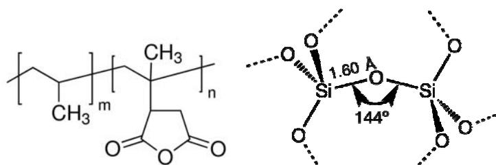
Fig. 1 – Chemical structure of maleated polypropylene (left) and silica (right).
