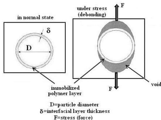
Fig. 7 – The theoretic model that correlates the interfacial adhesion and the voids formation under stress in nanocomposites filled with spherical particles (adapted after ref. 44).
