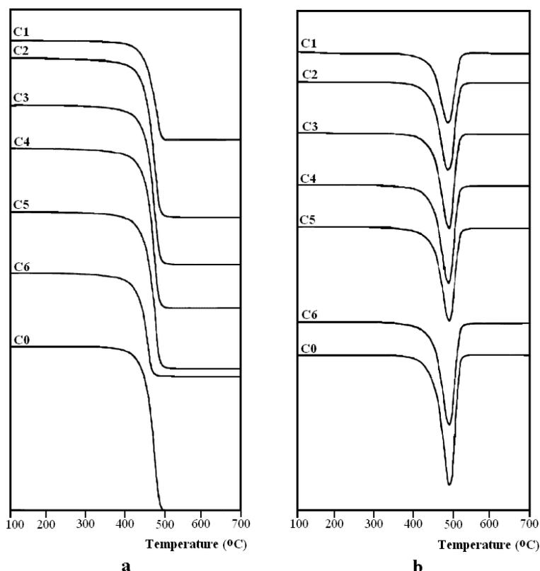
Fig. 5 – Thermal stability of the neat PP-g-MA (C0) and PP-g-MA – silica composites (C1-C6): a – TG data; b – DTG data.
