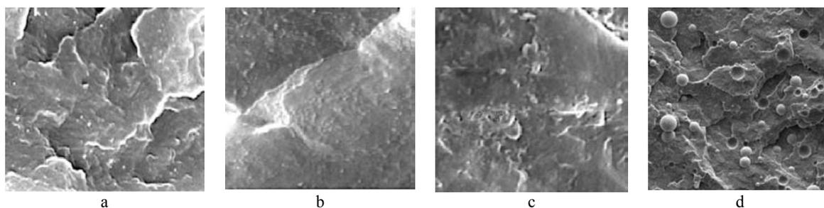
Fig. 2 – SEM micrographs: a – C1 (50 nm); b – C2 (200 nm); c – C3 (400 nm); d – C4 (2 μm).
