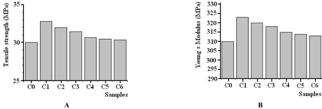
Fig. 6 – Tensile strength (A) and Young’s modulus (B) of the neat PP-g-MA (C0) and PP-g-MA – silica composites (C1-C6).
