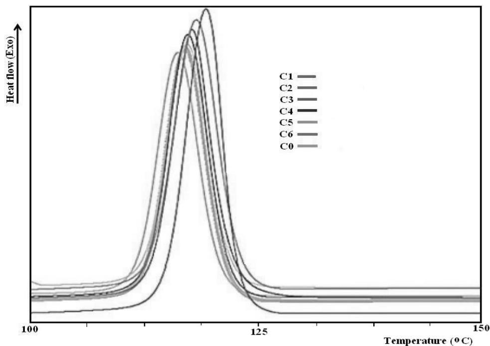
Fig. 4 – DSC scans on cooling of the neat PP-g-MA (C0) and PP-g-MA – silica composites (C1-C6).
