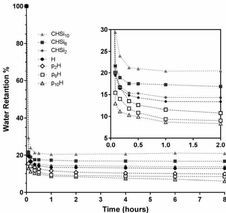
Fig. 5 – Water retention in hydrogels as function of time.
