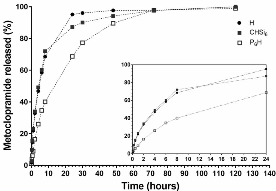
Fig. 7 – Release kinetics of Met from poly(NIPAAm-co-HEAAm) hydrogels in standard phosphate buffer solution of pH=7.4 at 37 °C. For comparison, the release profile of Met from SiMs was represented.
