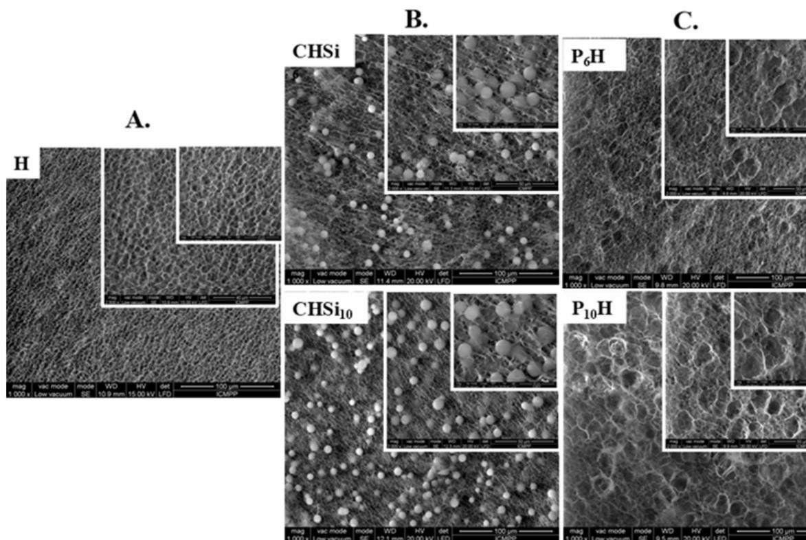
Fig. 2 – Scanning electron micrographs of conventional hydrogel (A), silica-incorporated composite hydrogels (B) and porous hydrogel after removal of SiMs (C).
