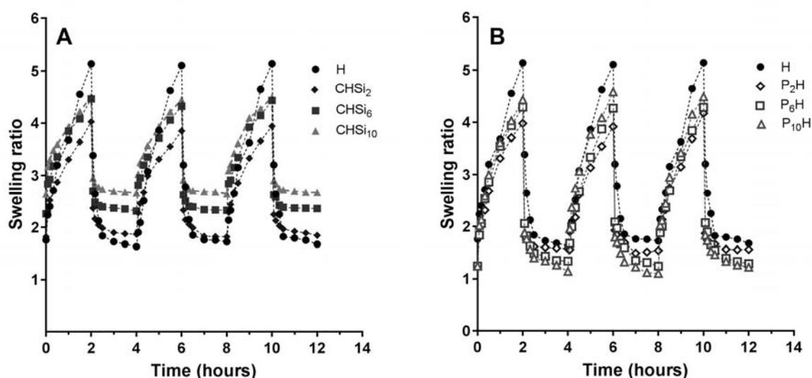
Fig. 6 – Cycles of the swelling/deswelling processes of the composite (A) and porous (B) hydrogels in comparison with conventional one (sample H).
