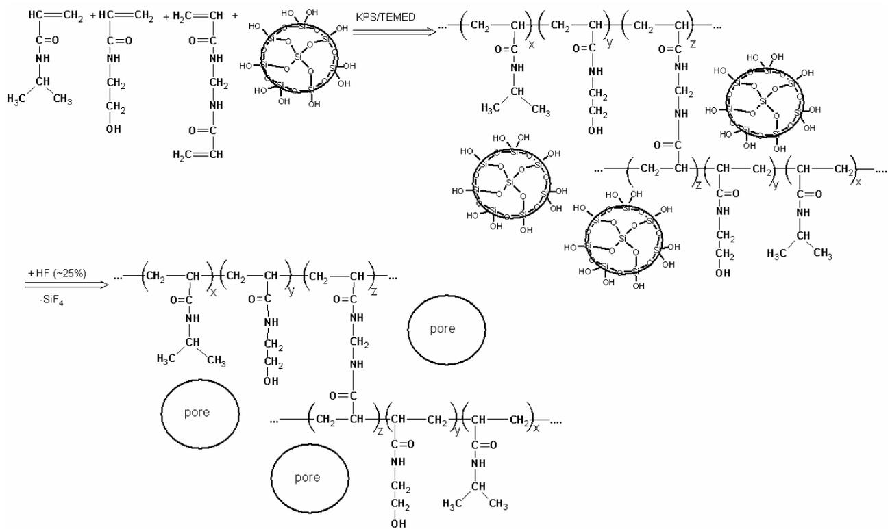
Fig. 1 – Schematic representation of the synthesis steps of porous hydrogels.
