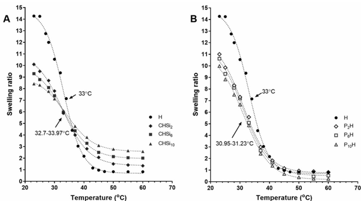
Fig. 3 – Swelling ratios of hydrogels as function of temperature.
