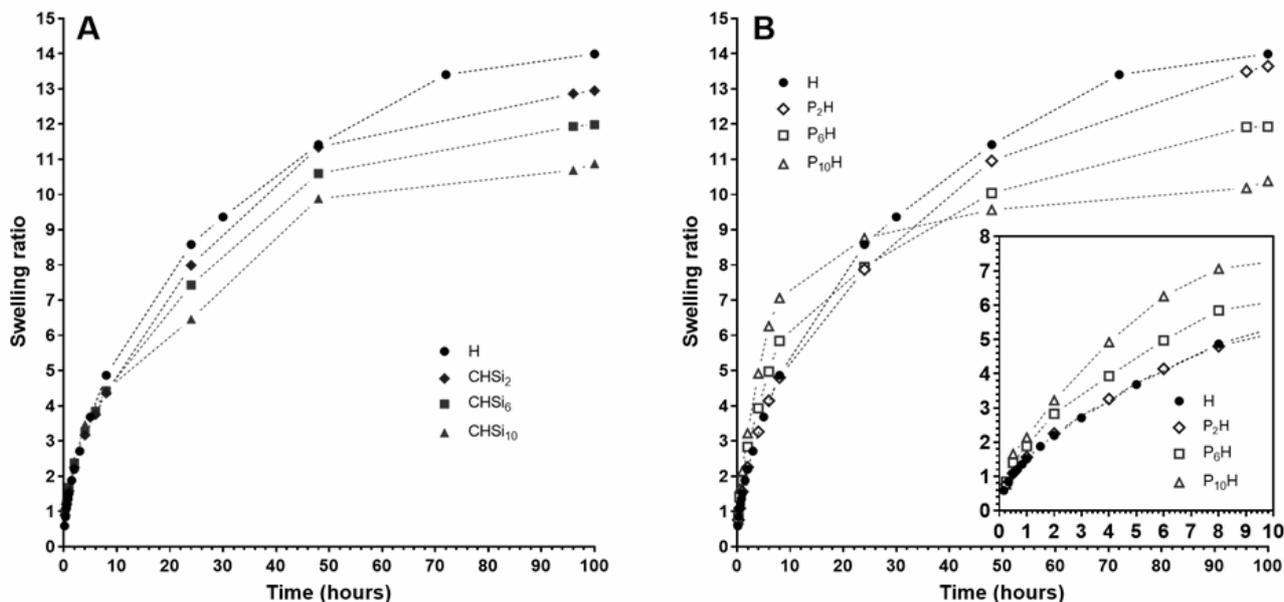
Fig. 4 – Swelling kinetic curves of composite (A) and porous (B) hydrogels in comparison with conventional one (sample H) in phosphate buffer solution at pH=7.4 at 25 °C.
