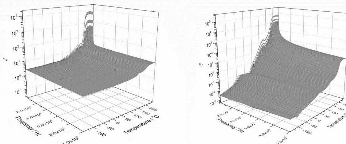
Fig. 9 – Dielectric permittivity of Ch (a) and PItAU\_Ch as a function of temperature and frequency.
