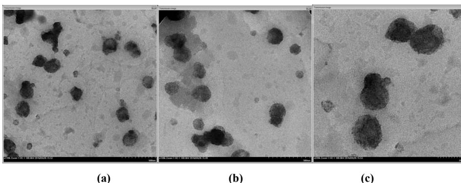
Fig. 4 – TEM images for PItAU/Ch samples synthesised in ratio of 4/1 (a), 2/1(b), and (c) 1/1.
