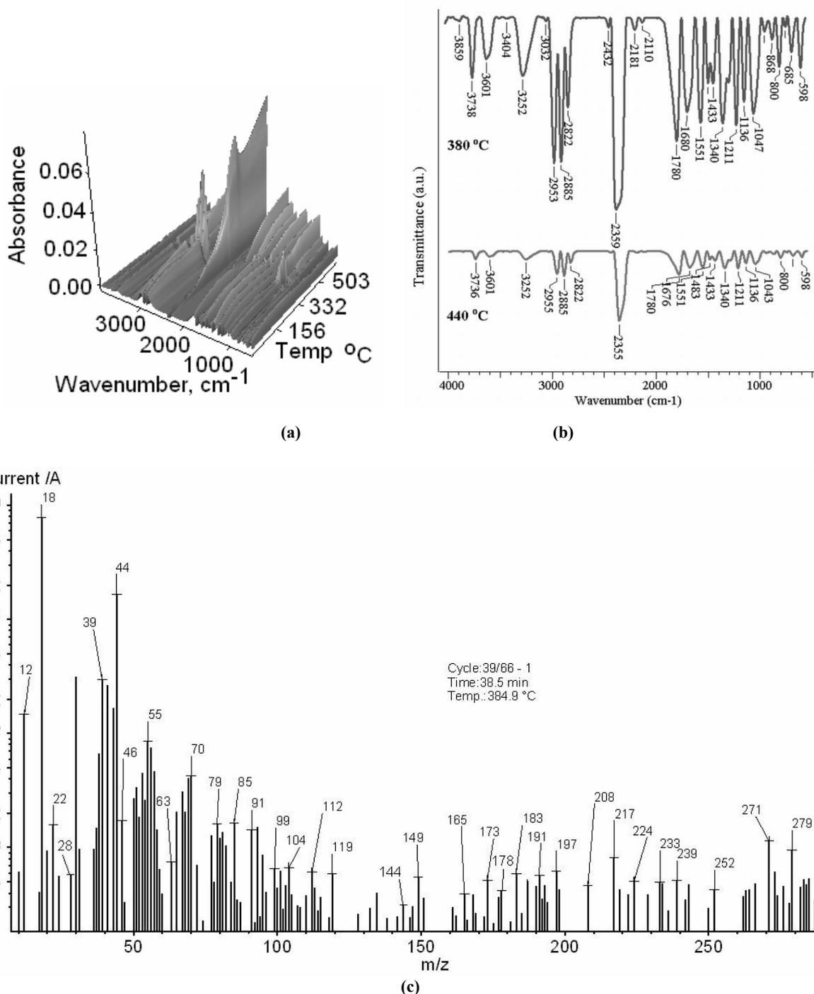
Fig. 3 – FTIR 3D spectrum of the PItAU\_Ch sample (a), FTIR 2D spectra of the evolved gases from the thermal decomposition of the PItAU\_Ch sample at 380 $^{\circ}\text{C}$  and 440 $^{\circ}\text{C}$  (b), and MS graphic of the evolved gases at the temperature of 385 $^{\circ}\text{C}$ .
