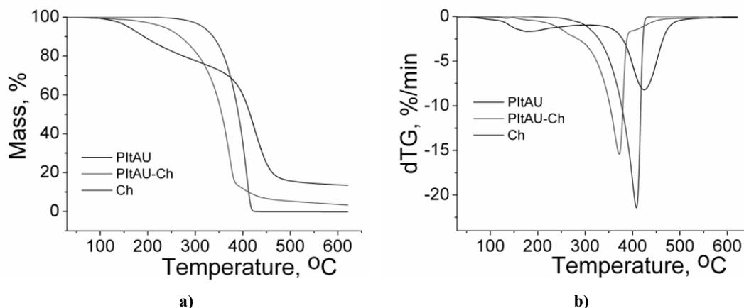
Fig. 2 – TG (a) and dTG (b) curves of the studied samples.
