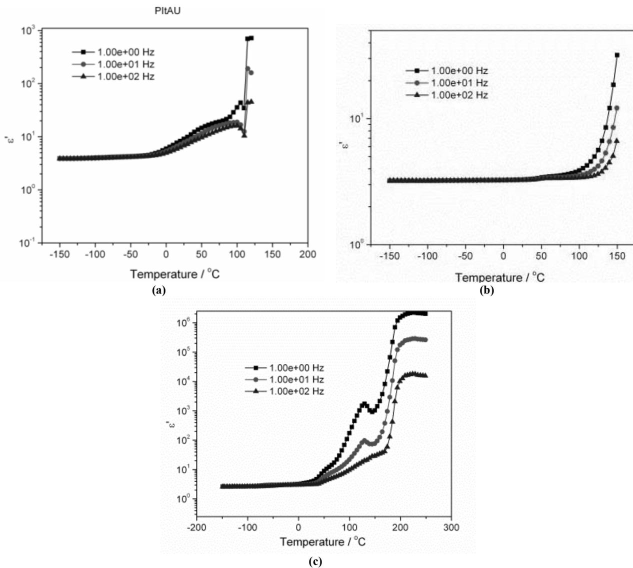
Fig. 7 – Logarithmic plot of the dielectric constant ( $\epsilon'$ ) for PItAU (a), Ch (b) and PItAU\_Ch (1:1) (c) as a function of temperature and specified frequencies.
