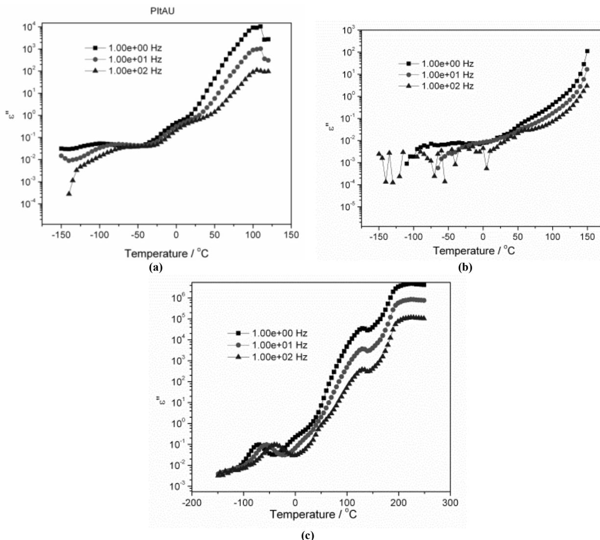
Fig. 8 – Logarithmic plot of the dielectric loss ( $\epsilon''$ ) of PItAU (a), Ch (b) and PItAU\_Ch in ratio of 1/1 (c) as a function of temperature and specified frequencies.
