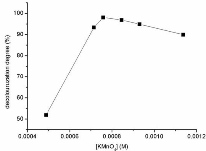
Fig. 4 – Inhibitory effect of permanganate for concentrations above 7.6 mM (Initial conditions: 0.008 g/L  $\beta$ CuPcS4, pH 11 and 56°C).
