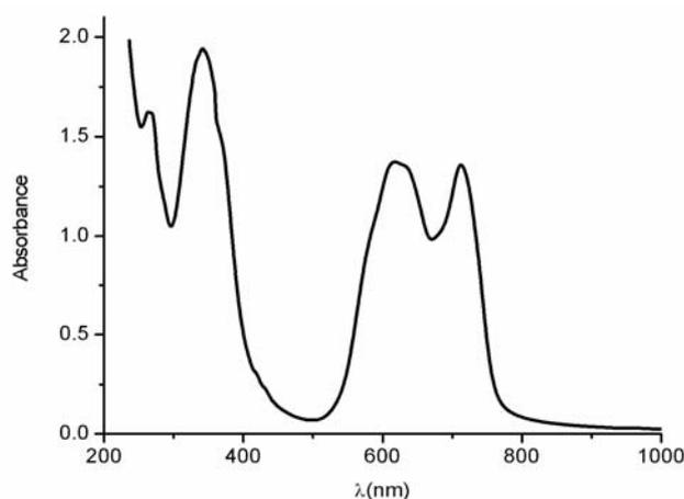
Fig. 1 – UV-VIS spectral features of  $\beta$ CuPcS4 in conditions similar to DNA Chelex extraction (0.008g/L phthalocyanine in 0.01% APG, pH 11 at 56°C).
