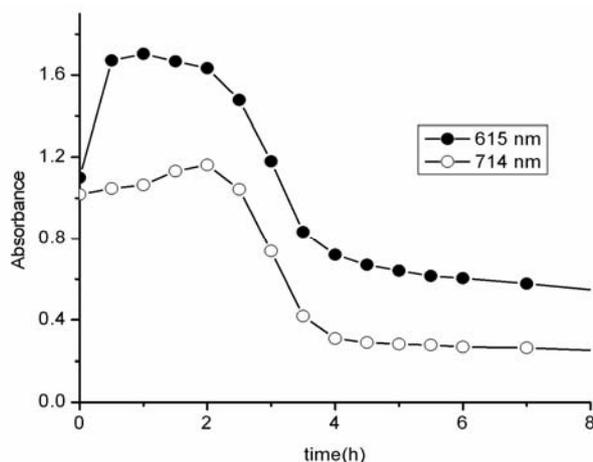
Fig. 2 – Typical absorbance changes at characteristic wavelengths during the permanganate assisted oxidation of  $\beta\text{CuPcS4}$  in alkaline medium (initial concentrations: 0.008 g/L  $\beta\text{CuPcS4}$ , 7.6 mM potassium permanganate at pH 11 and  $56^\circ\text{C}$ ).
