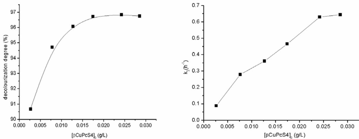
Fig. 5 – Increase of the decolourization degree (left) and degradation rate (right) over the initial concentration  $\beta$ CuPcS4 (Initial conditions: 7.6 mM permanganate, pH 11 and 56°C).
