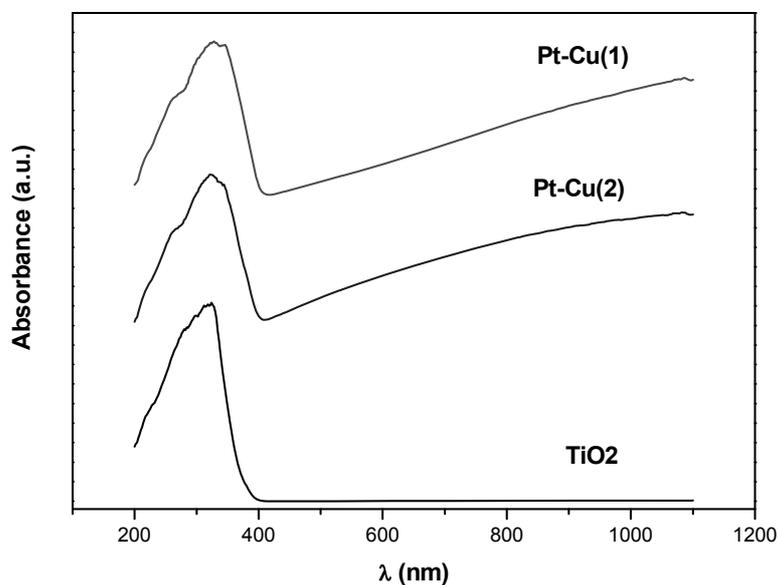
Fig. 4 – UV/vis spectra for calcined Pt-Cu(1), Pt-Cu(2) and TiO<sub>2</sub> (P25).
