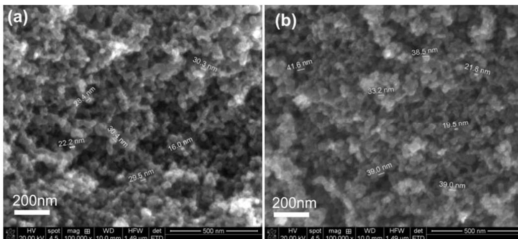
Fig. 2 – SEM images for (a) – Pt-Cu(1) and (b) – Pt-Cu(2) catalysts.
