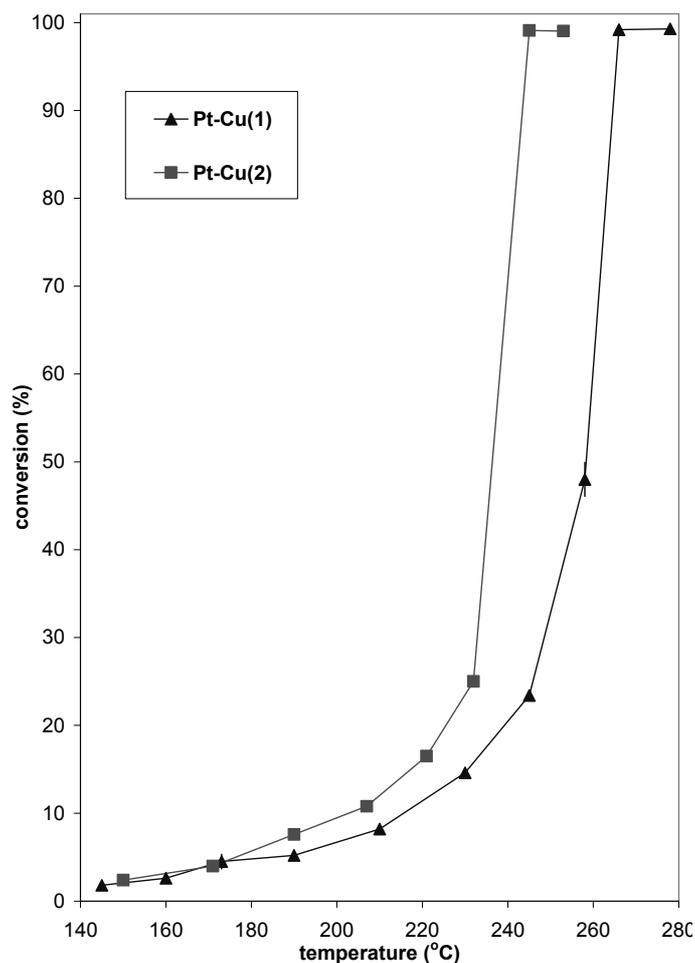
Fig. 5 – Conversion of CO over Pt-Cu/TiO<sub>2</sub> catalysts.
