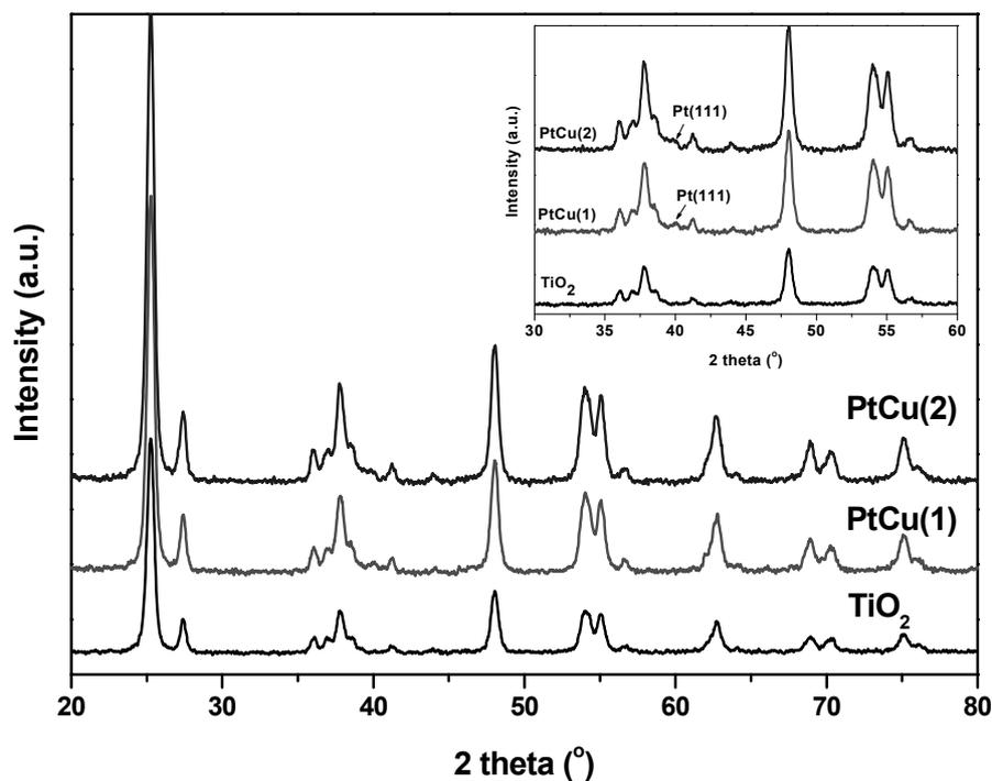
Fig. 1 – X-ray diffraction patterns of Pt-Cu(1) and Pt-Cu(2) catalysts.
