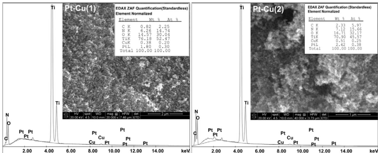
Fig. 3 – SEM-EDX Images for Pt-Cu(1) and Pt-Cu(2).
