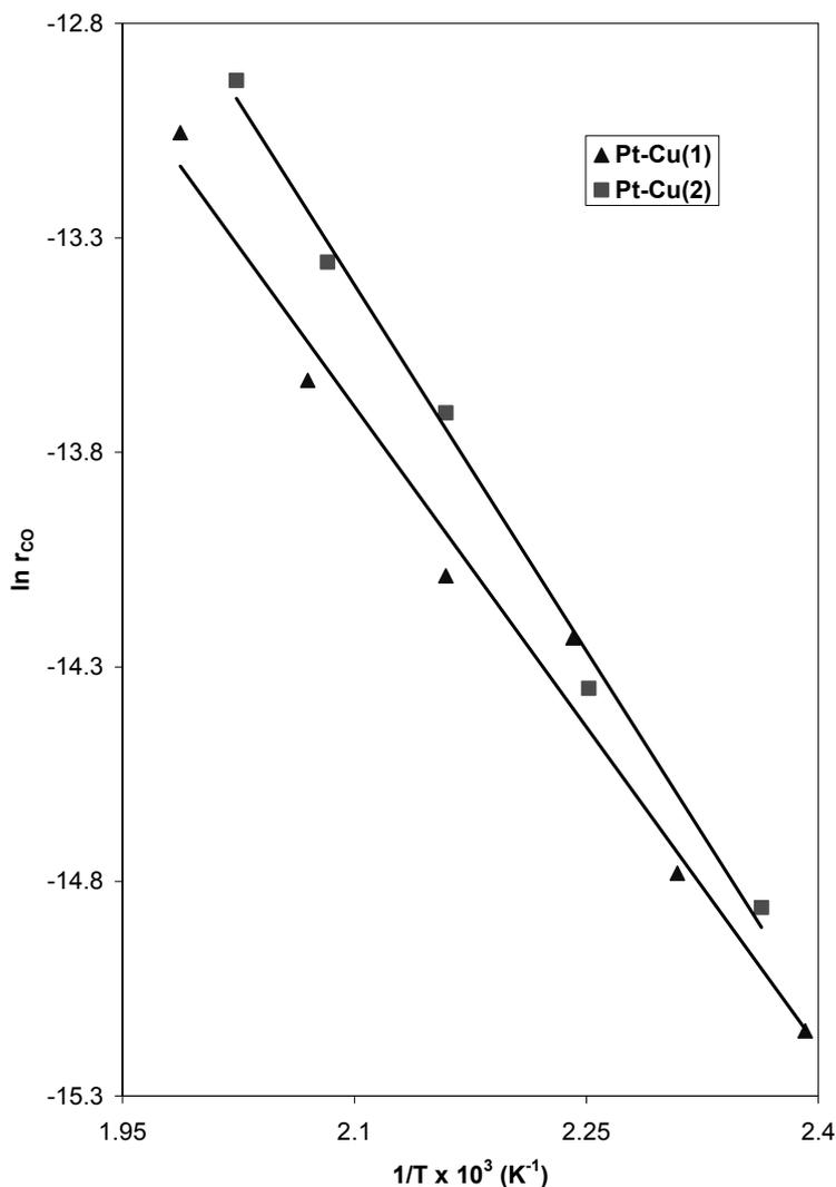
Fig. 6 – Logarithmic reaction rate of CO oxidation (measured in  $\text{mol s}^{-1} \text{g}_{\text{cat}}^{-1}$ ) over Pt-Cu catalysts vs. of reciprocal temperature.
