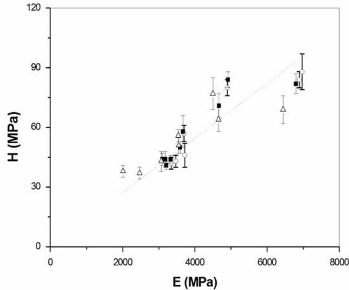
Fig. 9 – Relationship between Young's modulus  $E$  and microhardness  $H$  for the PP/PET compatibilized blends.
