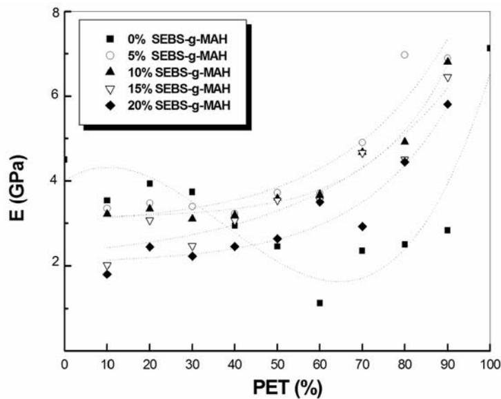
Fig. 4 – Young's modulus  $E$  of PP/PET blends, pure and compatibilized with SEBS-g-MAH, as a function of the PET content.
