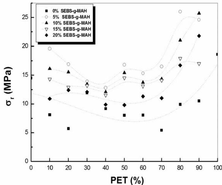
Fig. 5 – Tensile stress at break  $\sigma_r$  of PP/PET blends, pure and compatibilized with SEBS-g-MAH, as a function of the PET content.
