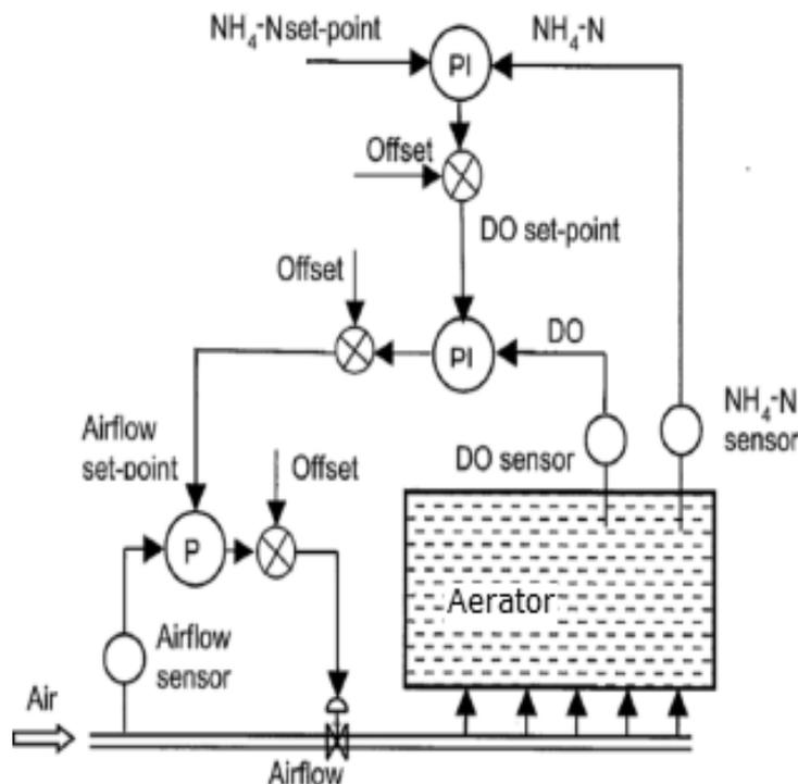
Fig. 3 – Control of aeration with ammonium measurement<sup>11</sup>.
