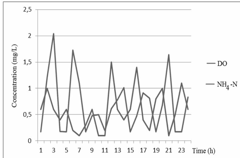
Fig. 4 – DO and NH<sub>4</sub>-N cycle profiles during monitoring of the nitrification process.
