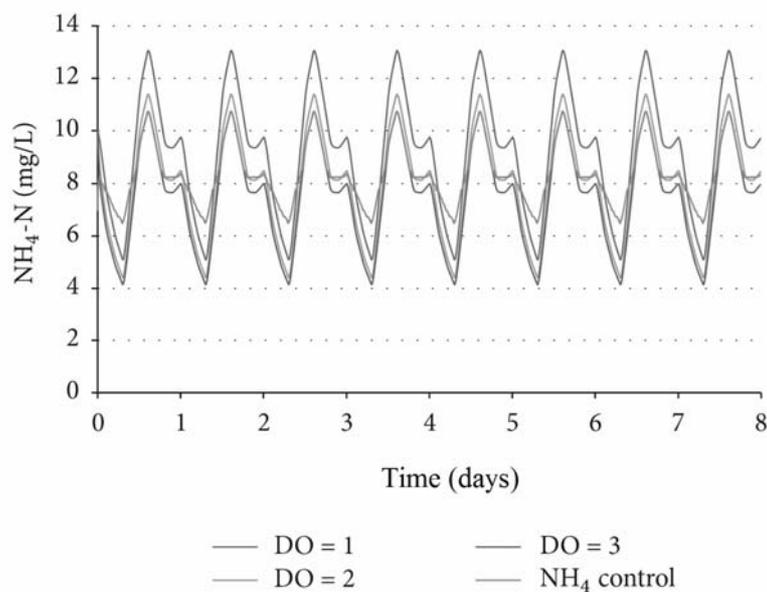
Fig. 2 – Nitrification process for high concentrations of ammonium<sup>11</sup>.
