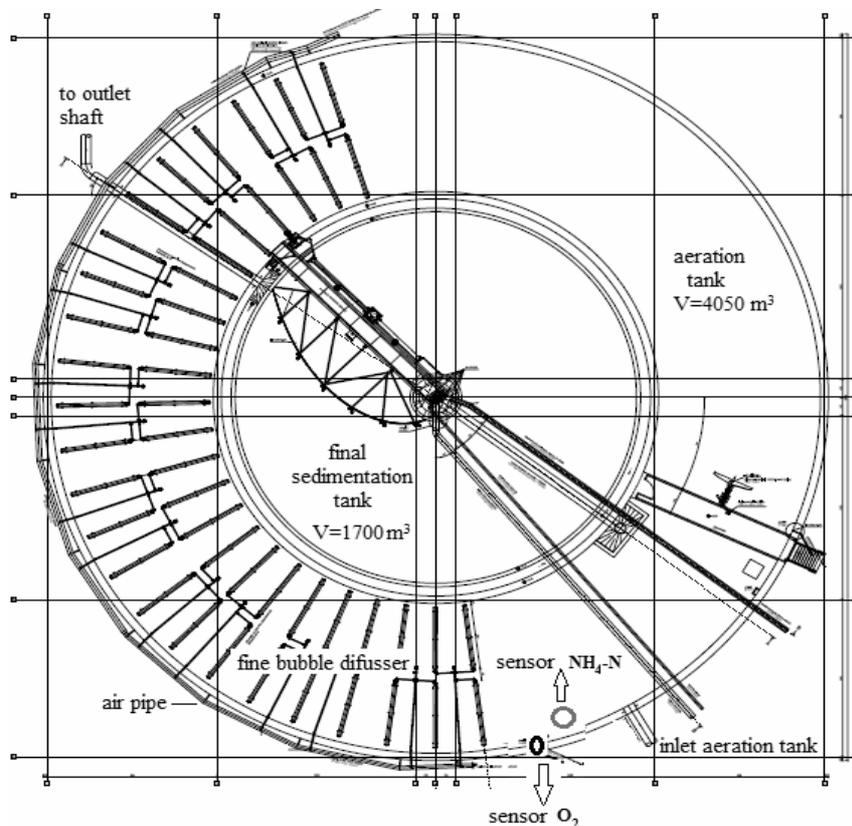
Fig. 5 – Sensor location of  $\text{NH}_4\text{-N}$  and oxygen for measurements in the aeration tank.
