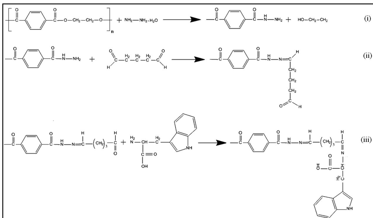
Fig. 4 – Scheme of reactions occurring during PET surface modification: (i) reaction of PET surface with hydrazine hydrate, (ii) reaction of PET-H surface with glutaraldehyde and (iii) reaction of PET-G surface with tryptophan.
