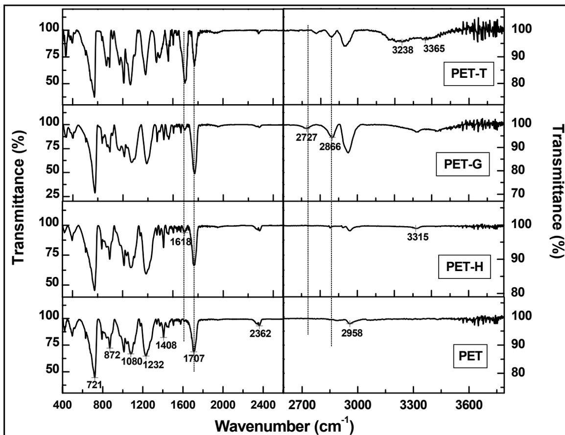
Fig. 2 – FTIR spectra of PET films (PET, PET-H, PET-G and PET-T).
