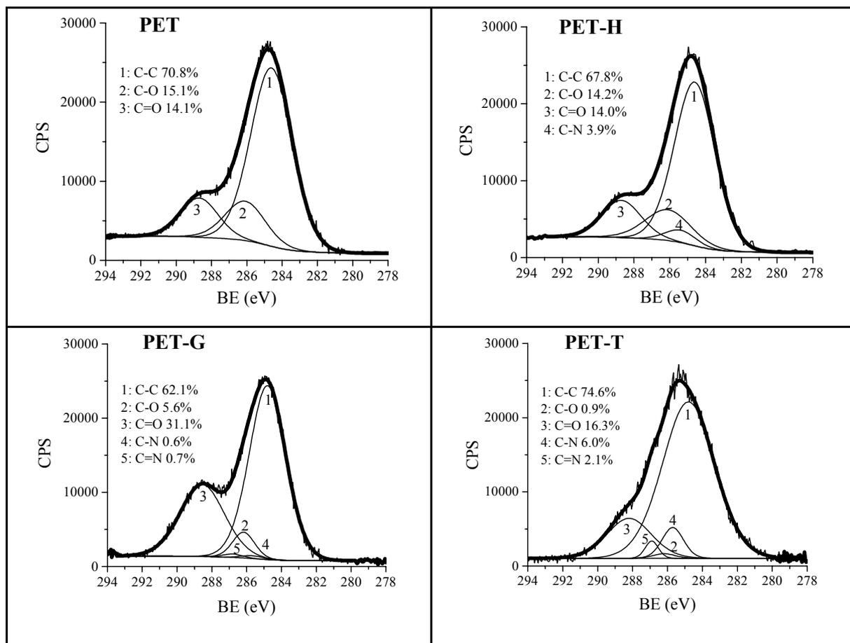
Fig. 3 – C1s XPS spectra of samples surfaces (PET, PET-H, PET-G and PET-T).
