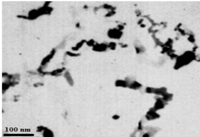
Fig. 4 – TEM micrograph of silica nanowires.
