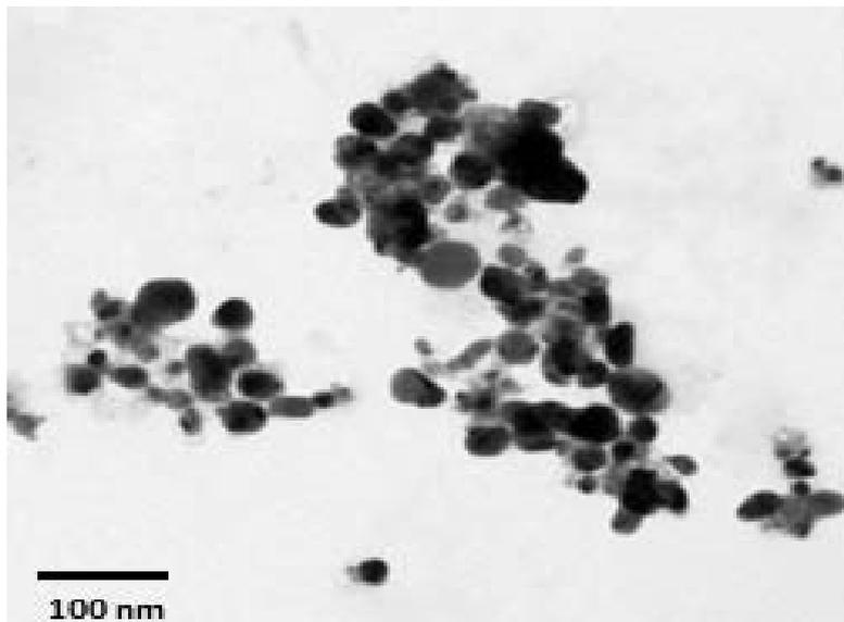
Fig. 3 – TEM micrograph of silica nanoparticles.
