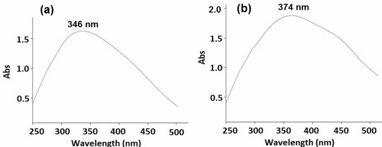
Fig. 1a – UV-Visible spectrum of silica nanoparticles, b: UV-Visible spectrum of silica nanowires.
