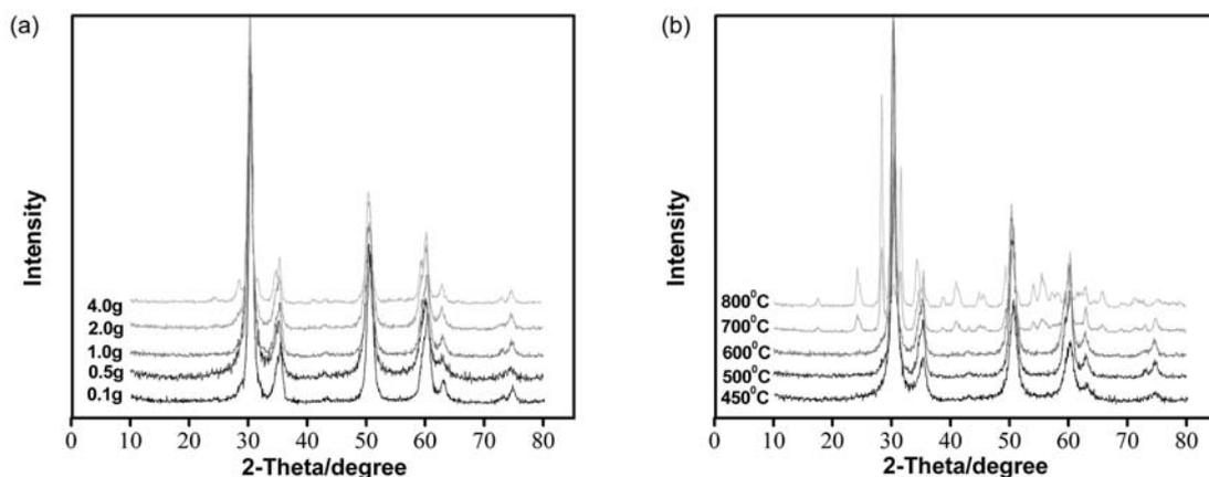
Fig. 2 – XRD characterization of  $ZrO_2$ -NiO. (a) XRD patterns of  $ZrO_2$ -NiO at different adding quality of  $Ni(NO_3)_2$ . (b) XRD patterns of  $ZrO_2$ -NiO prepared at different calcination temperatures.
