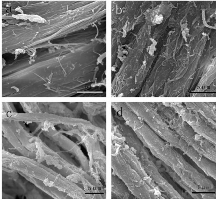
Fig. 1 – SEM images (a) pure collagen fiber (CF); (b) collagen fibers react with Zr and Ni ions; (c) fibrous  $ZrO_2$ -NiO calcined at 550 °C; (d)  $SO_4^{2-}/ZrO_2$ -NiO.
