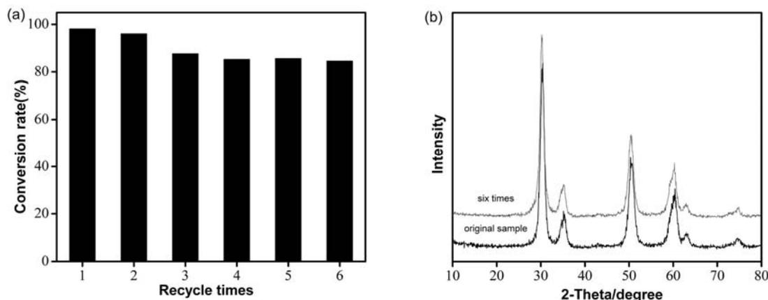
Fig. 5 – Reusability of the catalyst. (a) Reusability of the  $\text{SO}_4^{2-}/\text{ZrO}_2\text{-NiO}$  catalyst. (b) XRD patterns of  $\text{SO}_4^{2-}/\text{ZrO}_2\text{-NiO}$  after six times cycles.
