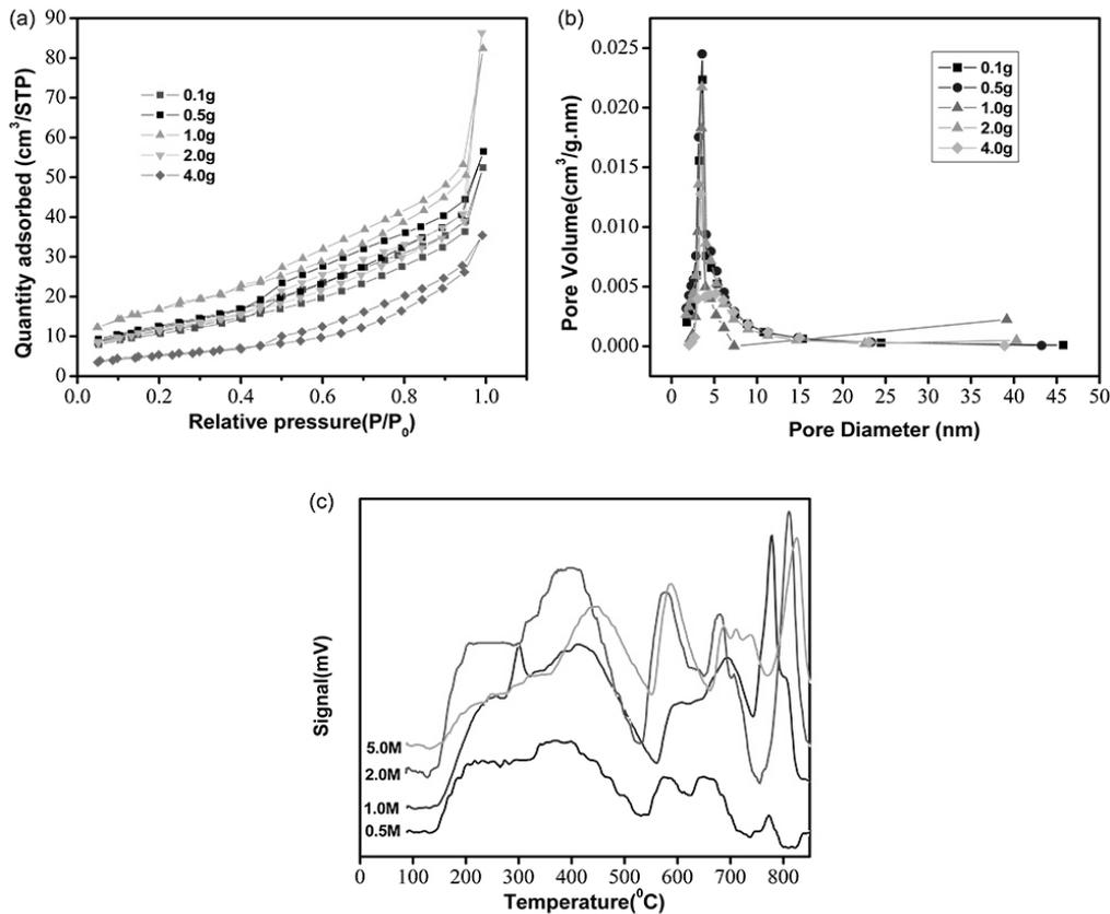
Fig. 3 – (a) N<sub>2</sub> adsorption-desorption isotherms of ZrO<sub>2</sub>-NiO prepared at different adding quality of Ni(NO<sub>3</sub>)<sub>2</sub>: 0.1g, 0.5g, 1.0g, 2.0g, 4.0g. (b) Pore size distribution curves of ZrO<sub>2</sub>-NiO prepared at different adding quality of Ni(NO<sub>3</sub>)<sub>2</sub>: 0.1g, 0.5g, 1.0g, 2.0g, 4.0g. (c) NH<sub>3</sub> – TPD curves of SO<sub>4</sub><sup>2-</sup>/ZrO<sub>2</sub>-NiO prepared at different acid concentration.
