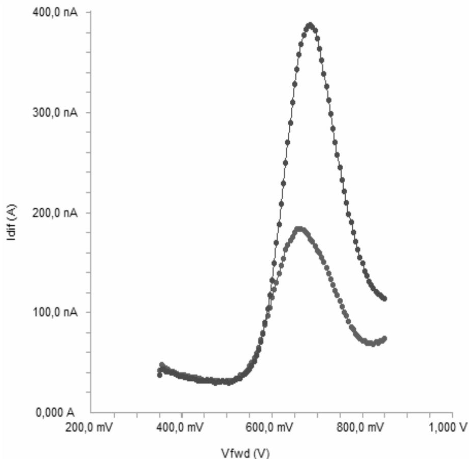
Fig. 10 – Thyromazol tablet DPV 2 for different two concentrations (10 and 25  $\mu\text{g/mL}$ ).
