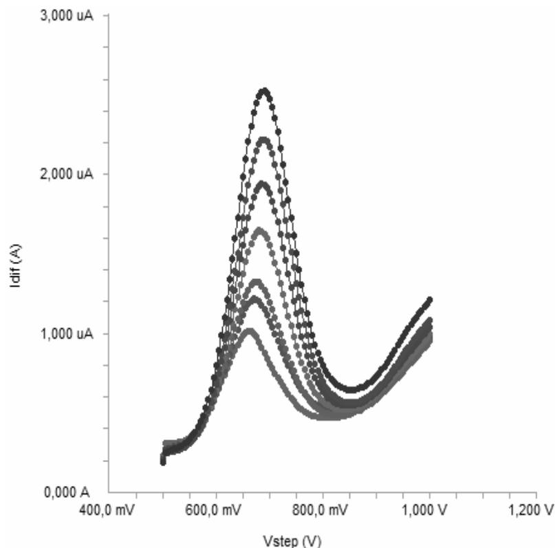
Fig. 7 – Square wave voltammograms (SWV) for different concentrations of methimazole at Bi<sub>2</sub>O<sub>3</sub>/Au electrode in 1 mM K<sub>3</sub>[Fe(CN)<sub>6</sub>]. Methimazole concentration; 5, 7.5, 10, 15, 20, 25 and 30 µg/mL (down to up).
