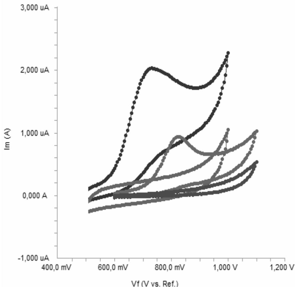
Fig. 5 – Cyclic voltammogram (CV) for the oxidation of 30  $\mu\text{g}/\text{mL}$  methimazole in 1 mM  $\text{K}_3[\text{Fe}(\text{CN})_6]$  containing 0.1 KCl at Au (111) electrode, scan rate: 0.1 V/s.
