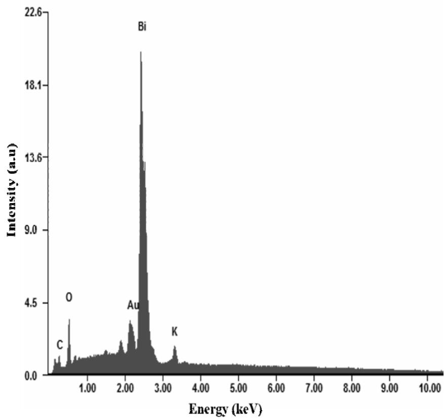
Fig. 4 – EDS spectrum of the electrodeposited  $\text{Bi}_2\text{O}_3$  nanostructures on a Au electrode at + 300 mV for 15 min.
