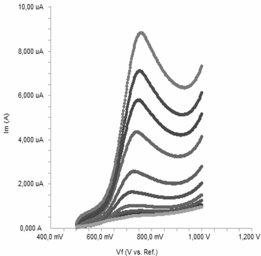
Fig. 6 – Linear sweep voltammograms (LSV) for the oxidation of 30 µg/mL methimazole in 1 mM K<sub>3</sub>[Fe(CN)<sub>6</sub>] on Bi<sub>2</sub>O<sub>3</sub>/Au electrode as a function of scan rate; from inner to outer, 5, 10, 25, 50, 100, 200, 400, 600, 800, 1000 mV/s.
