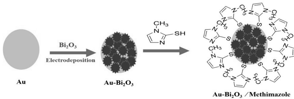
Scheme 1 – Schematic illustration of the electrochemically patterned Bi<sub>2</sub>O<sub>3</sub> biosensor on Au.
