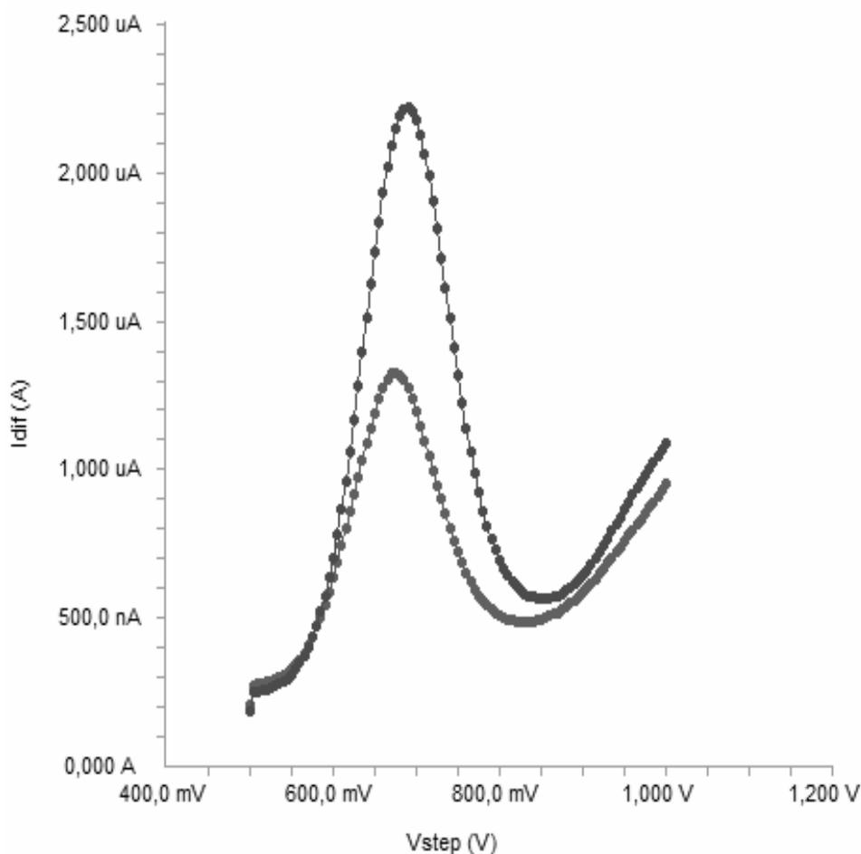
Fig. 9 – Thyromazol tablet SWV 2 for different two concentrations 10 and 25  $\mu\text{g/mL}$ .
