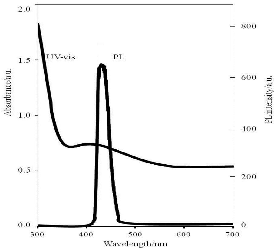
Fig. 3 – PL spectrum and UV-visible absorption spectrum of the electrodeposited  $\text{Bi}_2\text{O}_3$  nanostructures on ITO/quartz substrates.
