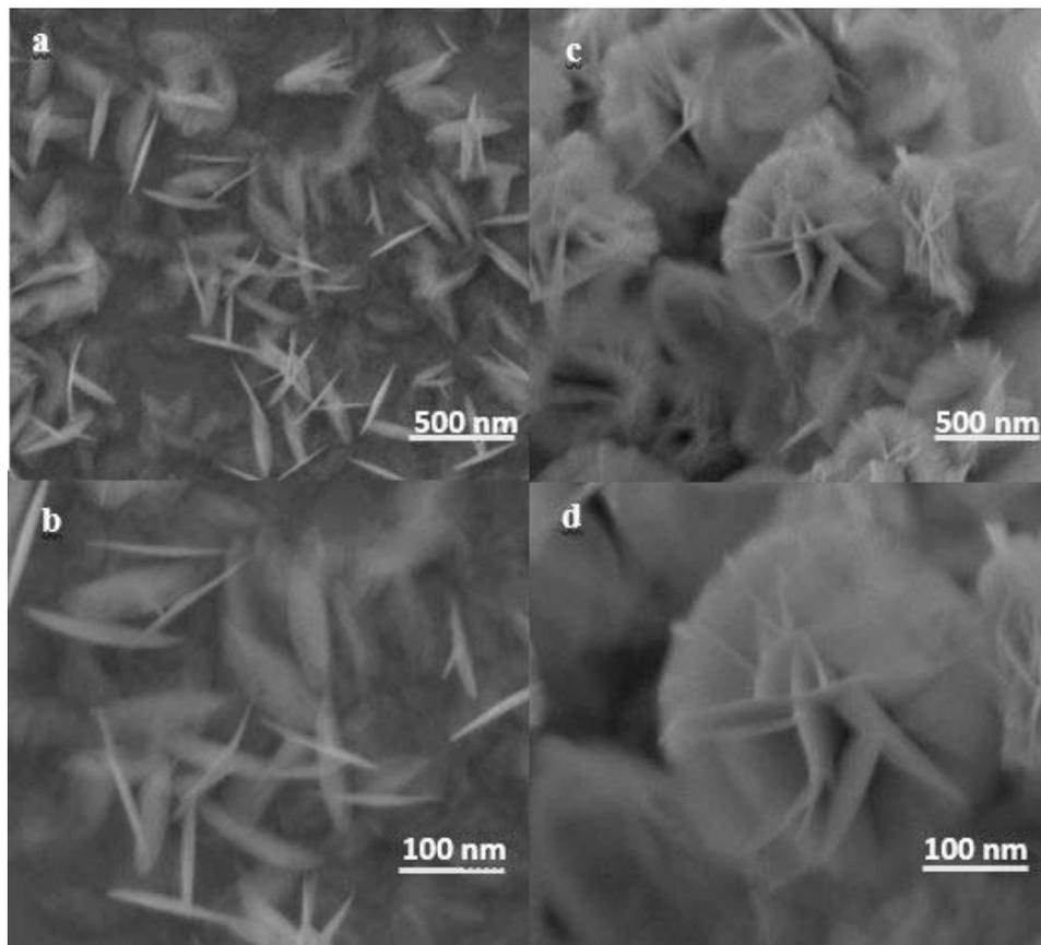
Fig. 2 – SEM images of the electrodeposited Bi<sub>2</sub>O<sub>3</sub> nanostructures on Au (111) electrodes (+ 300 mV) for 5 min (a-b) and 15 min (c-d).
