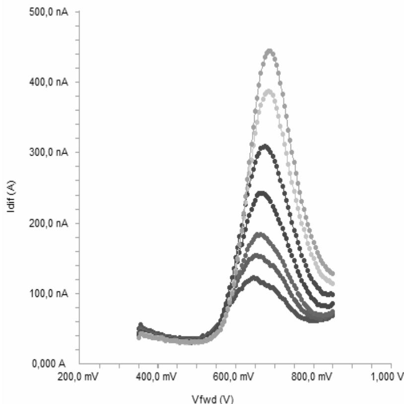
Fig. 8 – Differential pulse voltammograms (DPV) for different concentrations of at Bi<sub>2</sub>O<sub>3</sub>/Au electrode in 1mM K<sub>3</sub>[Fe(CN)<sub>6</sub>]. Methimazole concentration; 5, 7.5, 10, 15, 20, 25 and 30 µg/mL (down to up).
