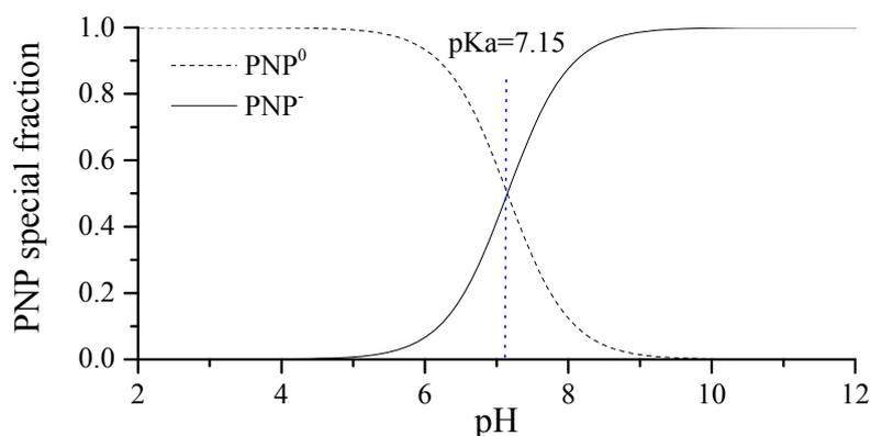
Fig. 8 – The distribution coefficient of PNP.
