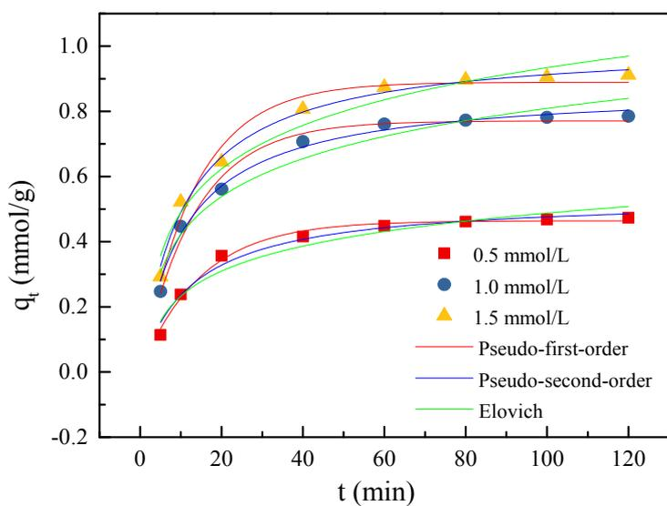
Fig. 10 – Kinetic models at different initial *p*-nitrophenol concentrations.
