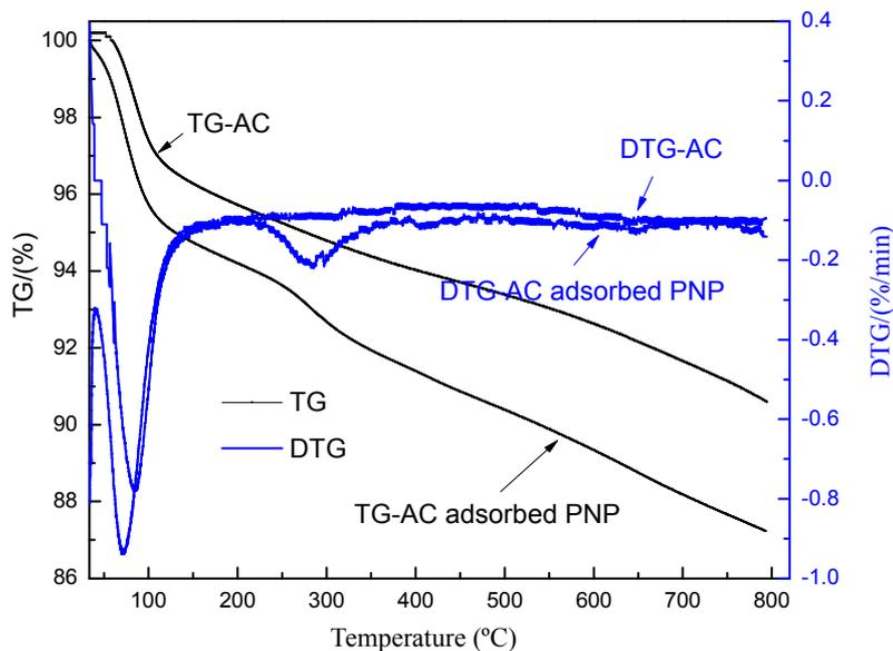
Fig. 4 – TG-DTG curves of AC before and after PNP adsorption.
