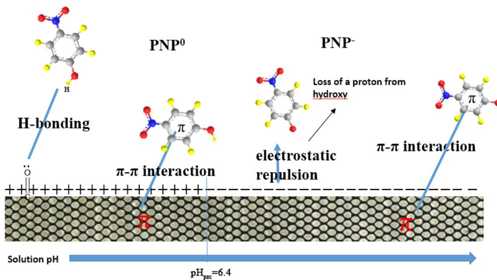
Fig. 9 – The contact model of PNP adsorption on AC at different pH.
