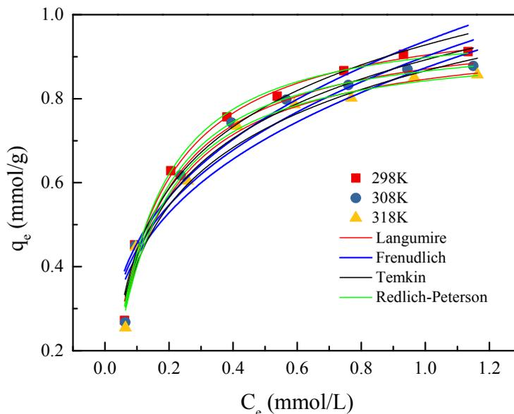
Fig. 14 – The isotherm models at different temperature.
