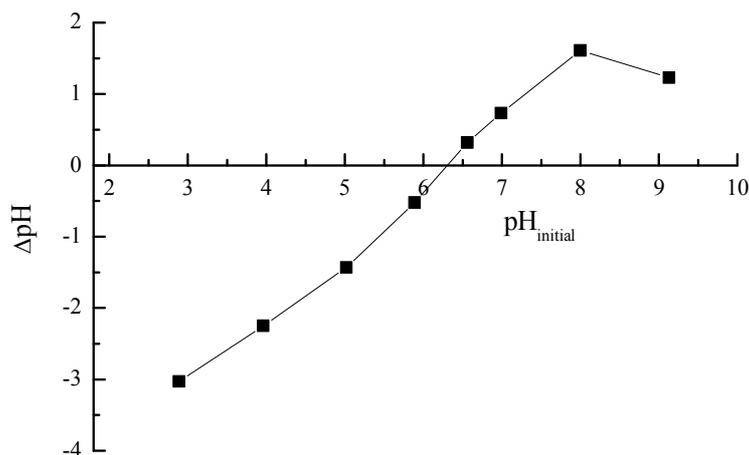
Fig. 5 – The point of zero charge of AC.
