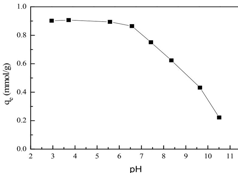
Fig. 7 – Effect of pH on the adsorption capacity of PNP ( $C_0=1.0$  mmol/L; adsorbent concentration=0.5g/L;  $t=60$ min;  $T=298$ K).
