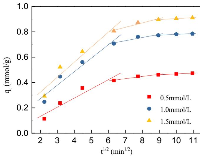
Fig. 12 – Intra-particle diffusion model at different initial concentrations.
