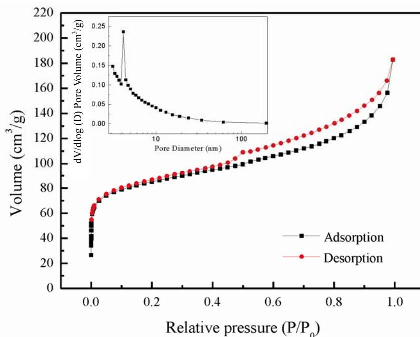
Fig. 1 – Nitrogen adsorption/desorption isotherms and pore size distribution of AC.
