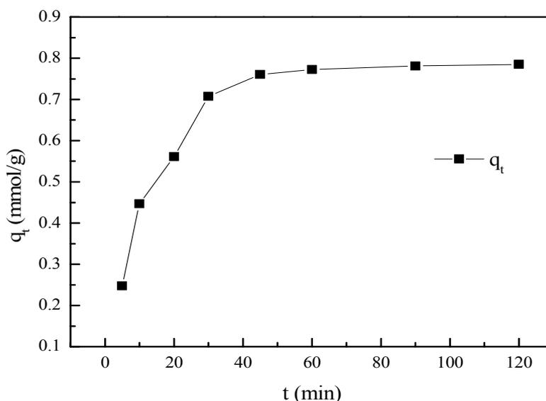
Fig. 6 – Effect of contact time on the adsorption capacity of AC ( $C_0=1.0$  mmol/L; adsorbent concentration=1g/L; initial pH=6.57;  $T=298K$ ).
