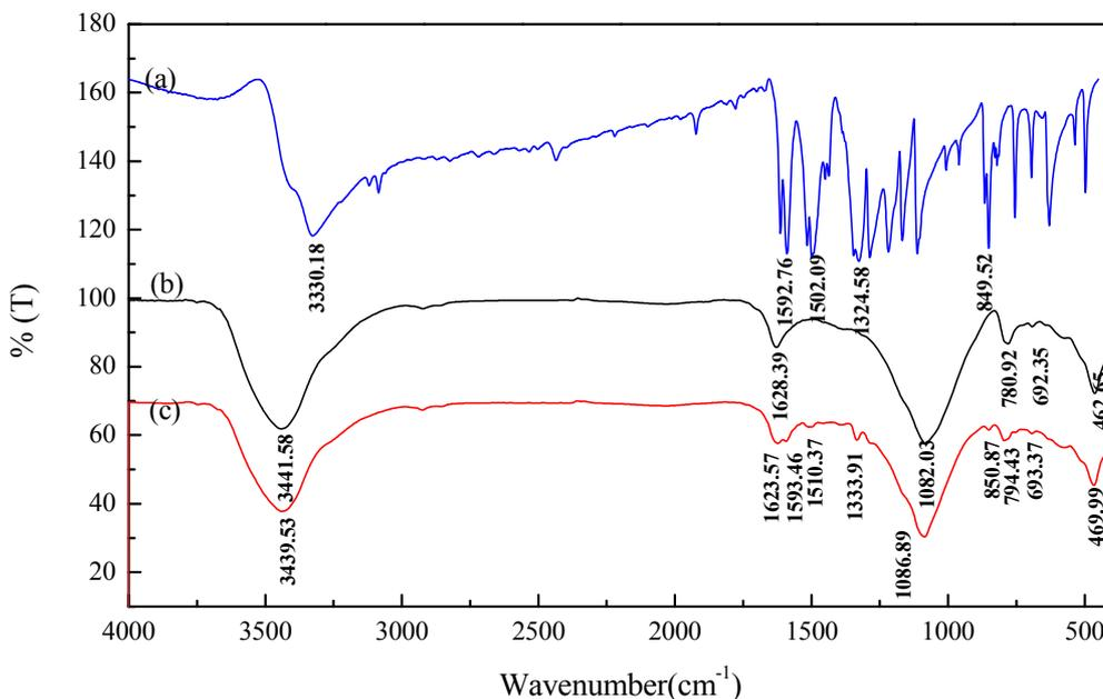
Fig. 3 – FTIR spectra of PNP(a), activated carbon(b) and activated carbon with adsorbed PNP (c).
