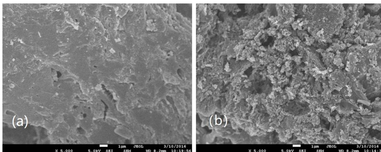
Fig. 2 – The SEM images of carbonized lignin (a) and AC (b).
