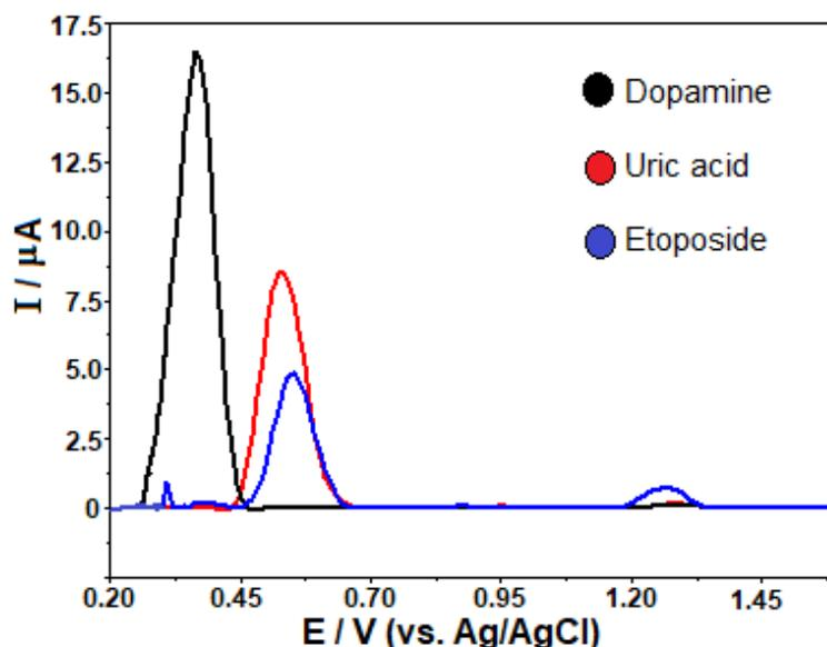
Fig. 4 – The SW stripping voltammograms demonstrating the effect of the presence of various interfering agents on  $0.025 \mu\text{g mL}^{-1}$  ETO (blue line) in Britton-Robinson buffer (pH 4.0). The studied interfering agents were:  $0.25 \mu\text{g mL}^{-1}$  dopamine (black line) and  $0.025 \mu\text{g mL}^{-1}$  uric acid (red line). Other operating conditions as indicated in Fig. 3.
