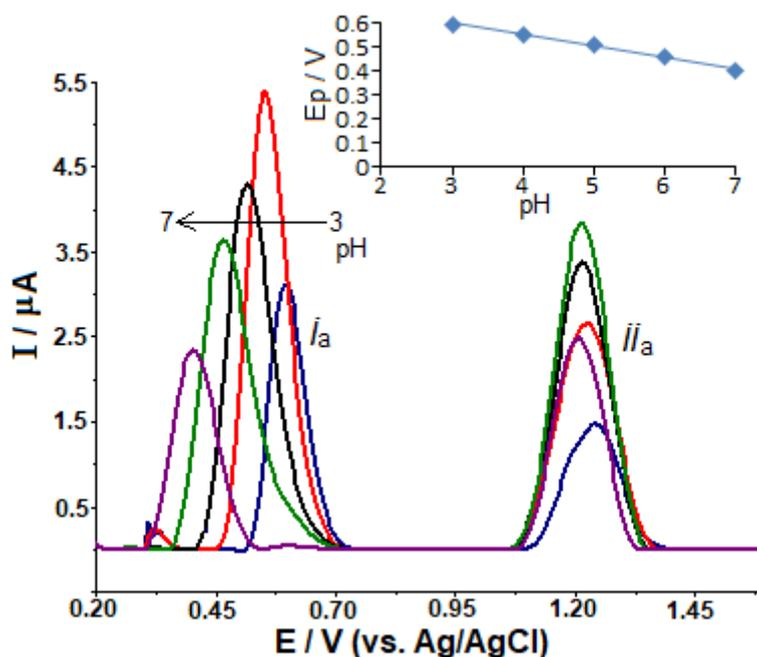
Fig. 2 – The SW stripping voltammograms of  $1 \mu\text{g mL}^{-1}$  ETO solutions in Britton-Robinson buffer pH 3–7 at GR/GCE.  $t_{\text{acc}} = 30$  s at open circuit condition; SWV parameters: frequency, 50 Hz; scan increment, 8 mV; pulse amplitude, 30 mV.
