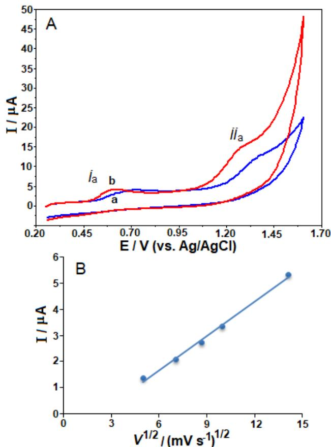
Fig. 1 – A) Cyclic voltammograms of bare GCE (a, blue line) and GR/GCE (b, red line) in Britton-Robinson buffer (pH 4.0) solution containing 100  $\mu\text{g mL}^{-1}$  ETO. Scan rate: 100 mV s<sup>-1</sup>. B) The plots of the peak current versus square root of scan rate.
