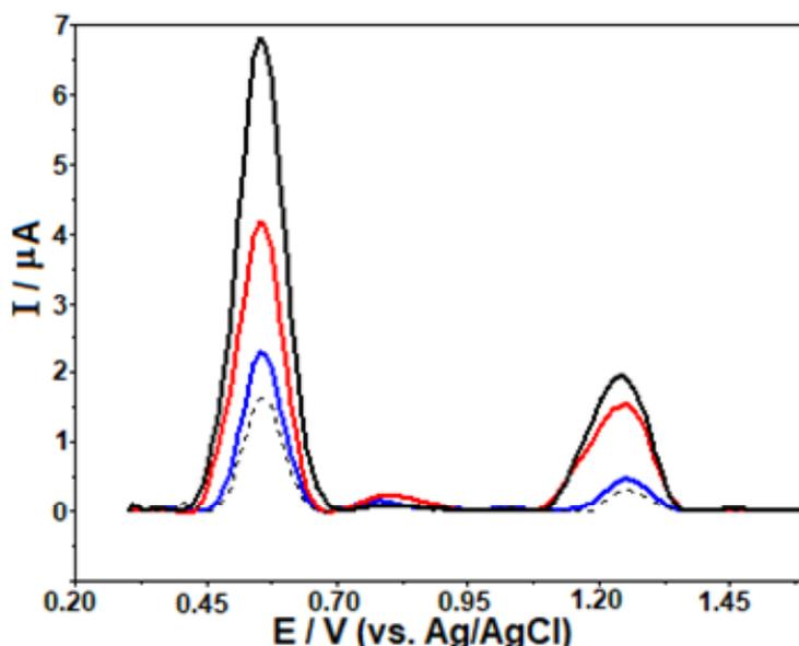
Fig. 5 – The SW stripping voltammograms obtained for the determination of ETO in the spiked sample. Dashed lines represent the diluted sample current. The sample spiked at a ETO levels of 0.025, 0.075 and 0.15. Other operating conditions as indicated in Figure 3.
