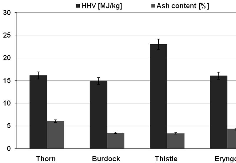
Fig. 2 –Variation of higher heating value (HHVf, MJ/Kg) versus ash content (%).
