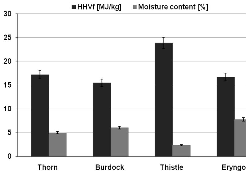
Fig. 3 – Variation of higher heating value (HHV, MJ/kg) versus moisture content (%).
