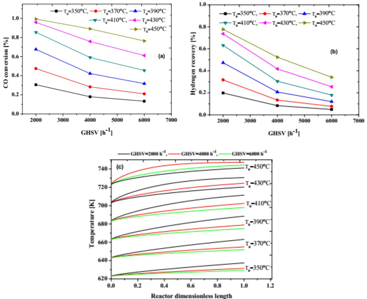
Fig. 5 – Reactor performance at different GHSV and at different inlet temperatures: (a): CO conversion, (b): hydrogen recovery, (c): axial temperature profiles. Conditions:  $P_0 = 1$  atm,  $F_I = 150$  mL/min, H<sub>2</sub>O/CO feed molar ratio = 1/1.
