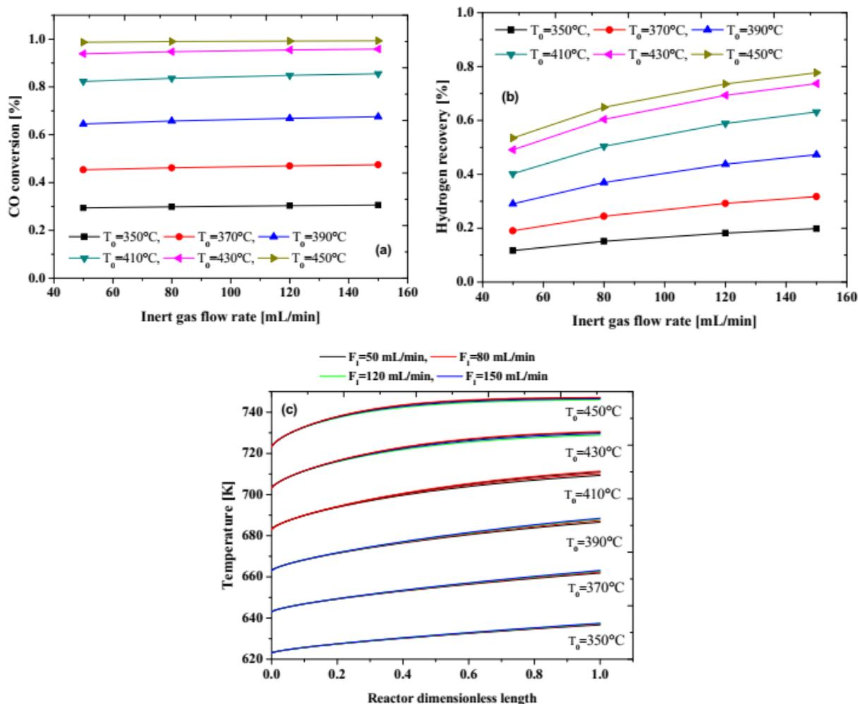
Fig. 4 – Reactor performance at different inert gas flow rates and for different inlet temperatures: (a): CO conversion, (b): hydrogen recovery, (c): axial temperature profiles. Conditions:  $P_0 = 1$  atm, H<sub>2</sub>O/CO feed molar ratio = 1/1, GHSV = 2000 h<sup>-1</sup>.
