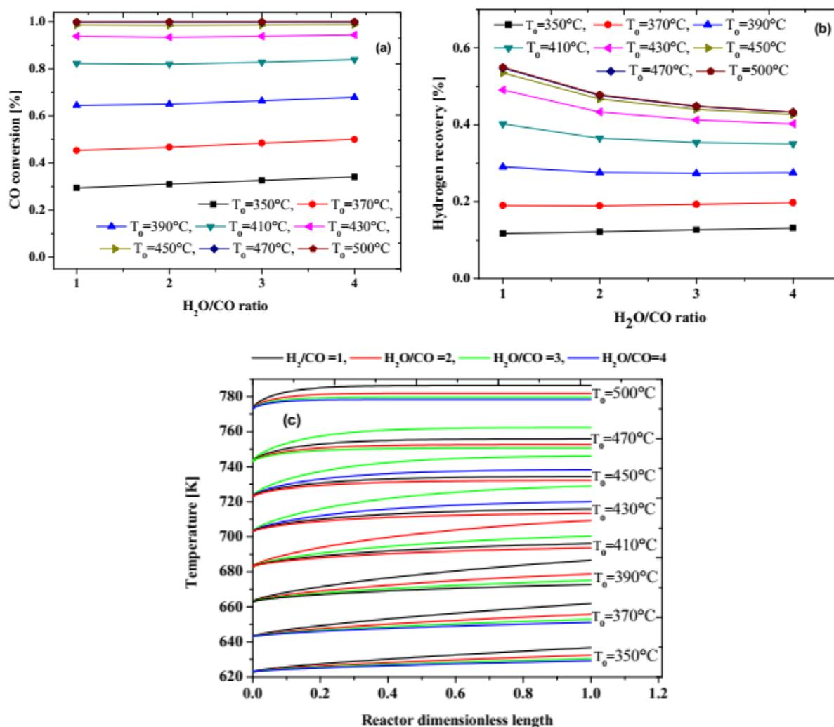
Fig. 2 – Reactor performance at different  $H_2O/CO$  molar ratio and different inlet temperatures: (a): CO conversion, (b):  $H_2$  recovery, (c): axial temperature profile. Conditions:  $P_0 = 1\text{atm}$ ,  $F_1 = 50\text{ mL/min}$ ,  $GHSV = 2000\text{h}^{-1}$ .
