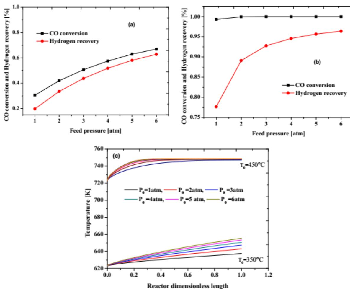
Fig. 6 – Reactor performance at different initial pressures and at different inlet temperatures: (a): CO conversion and hydrogen recovery at T<sub>0</sub> = 350°C, (b): CO conversion and hydrogen recovery at T<sub>0</sub> = 450°C, (c): axial temperature profiles at T<sub>0</sub> = 350°C and T<sub>0</sub> = 450°C. Conditions: H<sub>2</sub>O/CO feed molar ratio = 1/1, F<sub>l</sub> = 150 mL/min, GHSV = 2000 h<sup>-1</sup>.
