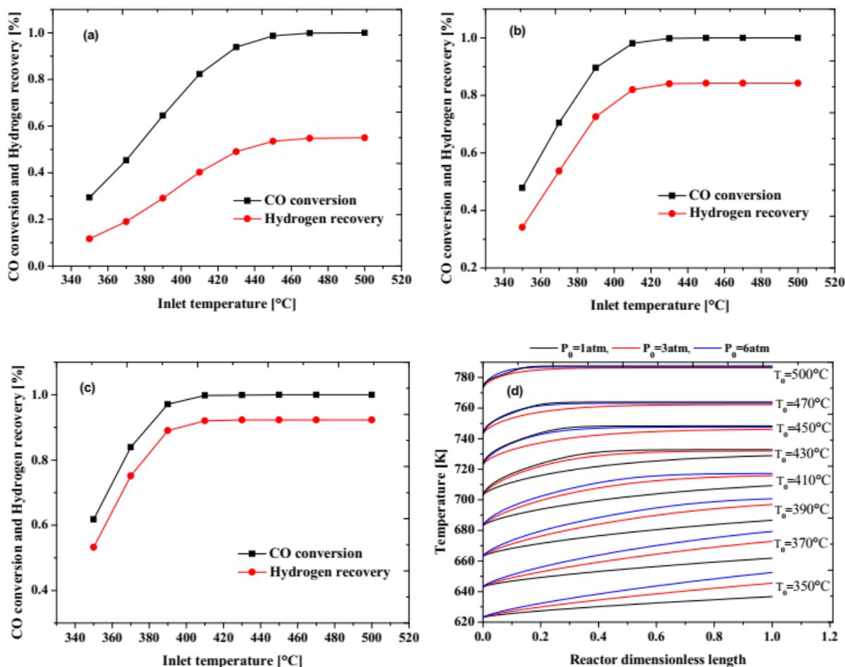
Fig. 3 – Reactor performance at different inlet temperature and at different initial total pressures: (a): CO conversion and hydrogen recovery for  $P_0=1\text{atm}$ , (b): CO conversion and hydrogen recovery for  $P_0=3\text{ atm}$ , (c): CO conversion and hydrogen recovery for  $P_0=6\text{atm}$ , (d): axial temperature profiles. Conditions:  $F_I = 50\text{ mL/min}$ ,  $\text{GHSV} = 2000\text{ h}^{-1}$ ,  $\text{H}_2\text{O}/\text{CO}$  feed molar ratio = 1/1.
