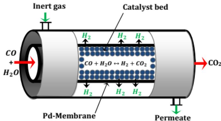
Fig. 1 – Schematic representation of Pd-Ag membrane reactor.
