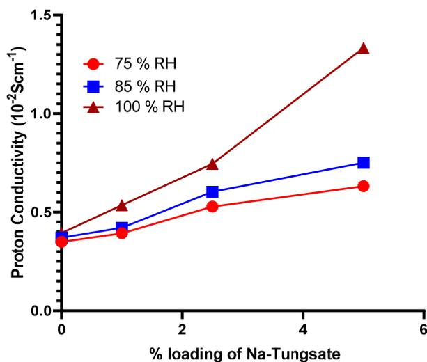
Fig. 6 – Proton conductivity curves for the different Na-Tungstate loaded membranes.
