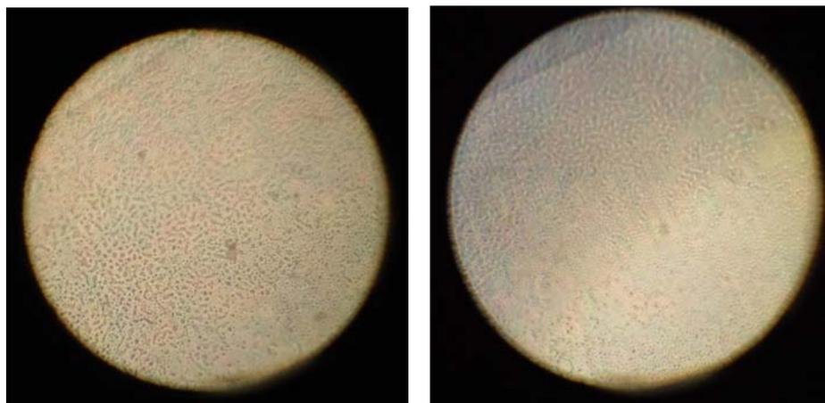
Fig. 4 – Optical microscopy of (a) plain PVA and (b) PVA loaded with ZnO (2.5 wt. %).
