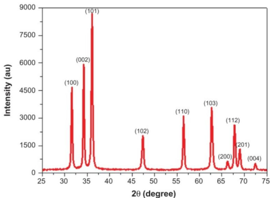
Fig. 3 – X-RD patterns of ZnO Nanoparticles.
