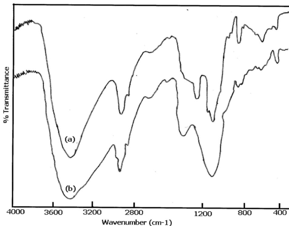
Fig. 2 – FTIR tracings of (a) Plain and (b) PVA-ZnO membranes.
