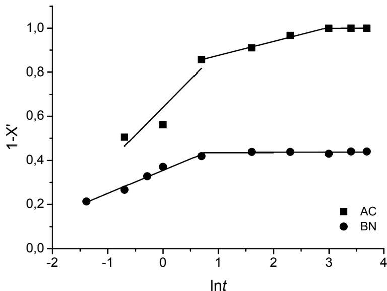
Fig. 6 – Elovich plots for the kinetic modelling of MBT adsorption.
