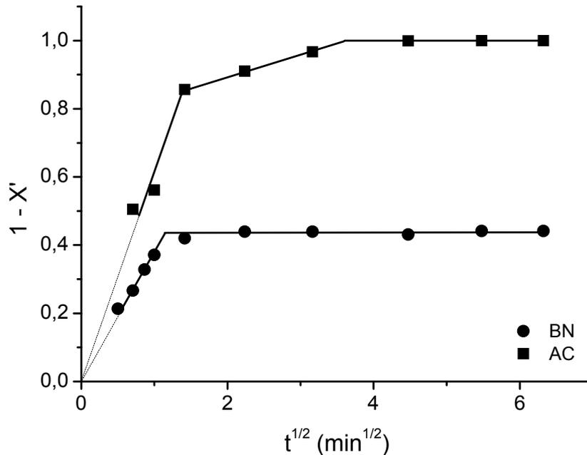
Fig. 3 – Weber and Morris plots for the kinetic modelling of MBT adsorption.
