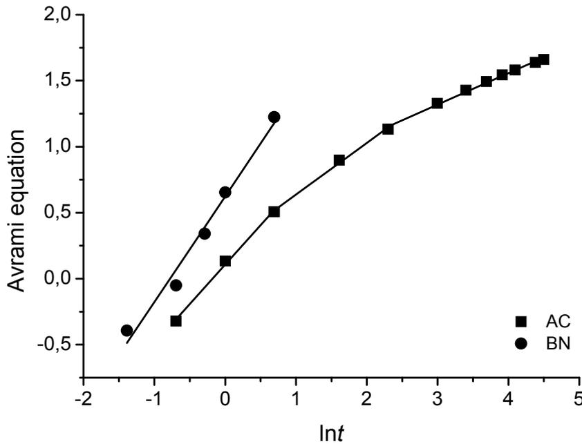
Fig. 7 – Avrami plots for the kinetic modelling of MBT adsorption.
