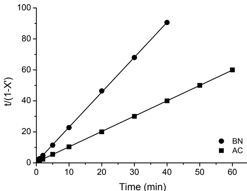
Fig. 8 – Pseudo-second order plots for the kinetic modelling of MBT adsorption.
