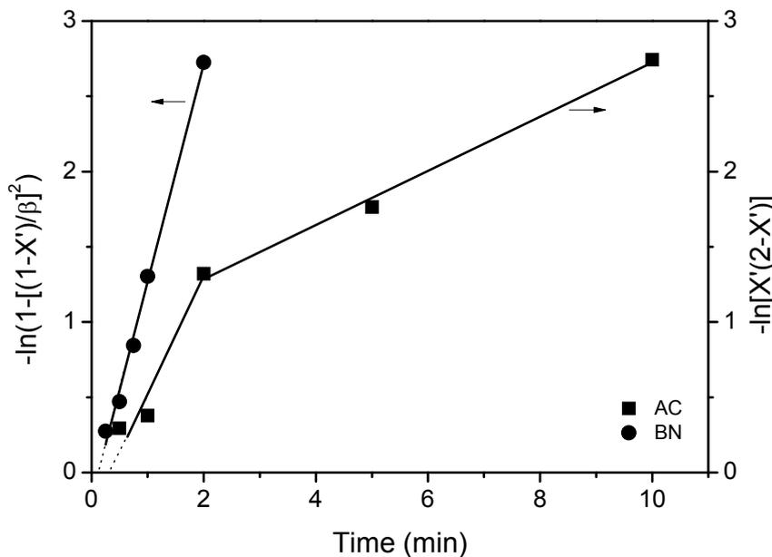
Fig. 5 – Urano and Tachikawa plots for the kinetic modelling of MBT adsorption.
