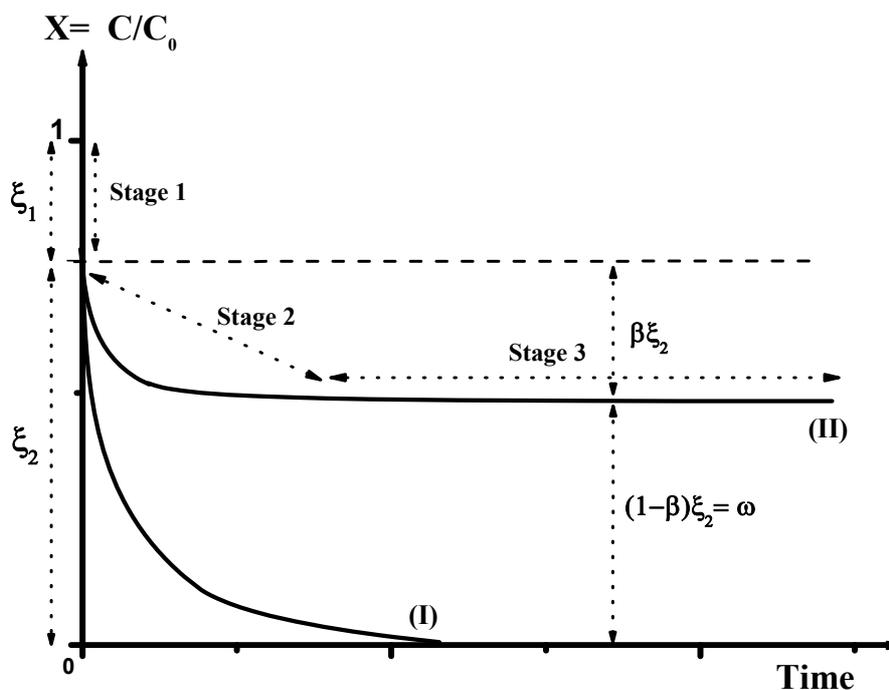
Fig. 1 – Evolution of the residual concentration fraction of a solute vs adsorption time (two and three stages models).
