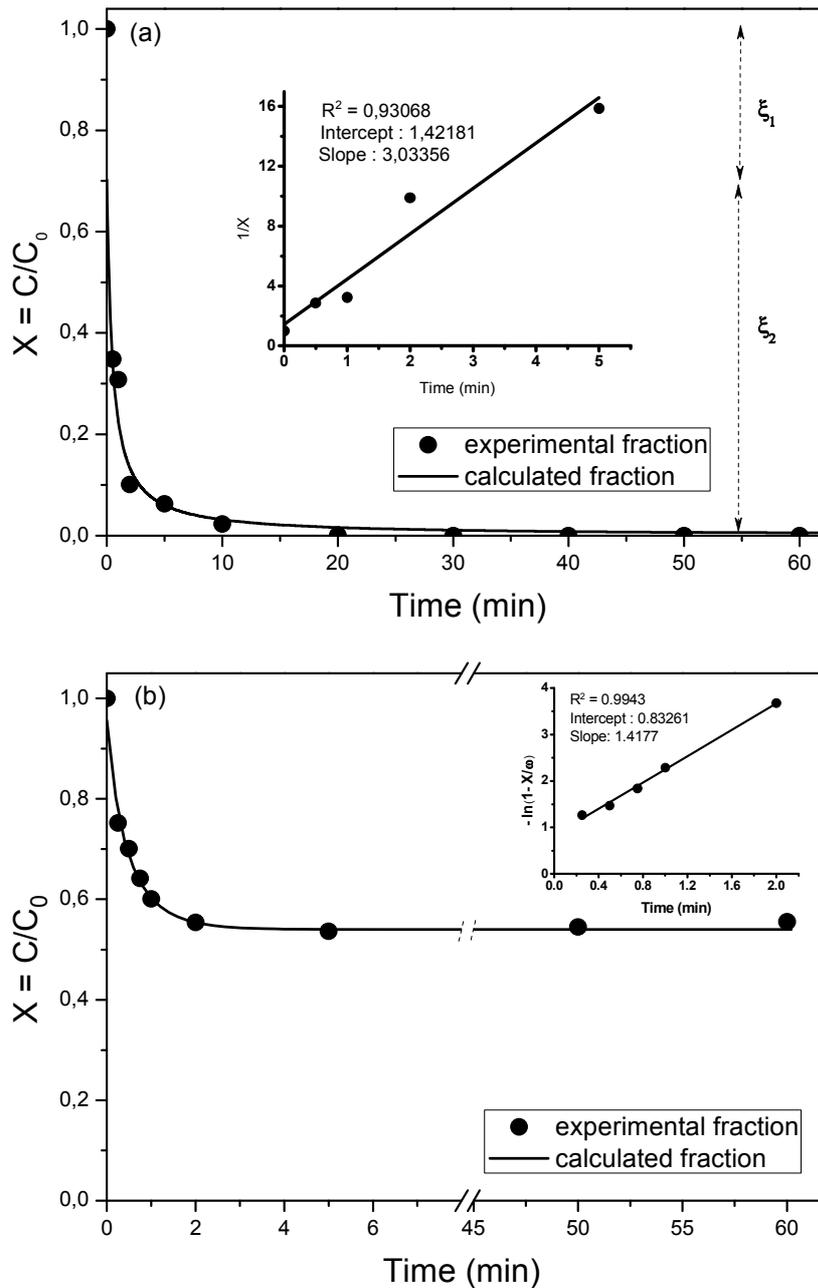
Fig. 2 – Evolution of the residual concentration fraction of MBT ( $C_0 = 20 \text{ mg.L}^{-1}$ ,  $m_{\text{ads}} = 0.5 \text{ g.L}^{-1}$ ,  $\text{pH} \approx 6.5$  et  $T = 20 \pm 1 \text{ }^\circ\text{C}$ ) vs adsorption time : (a) AC, (b) BN.
