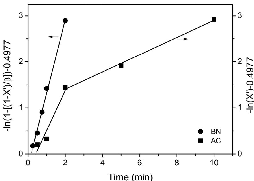
Fig. 4 – Boyd plots for the kinetic modelling of MBT adsorption.
