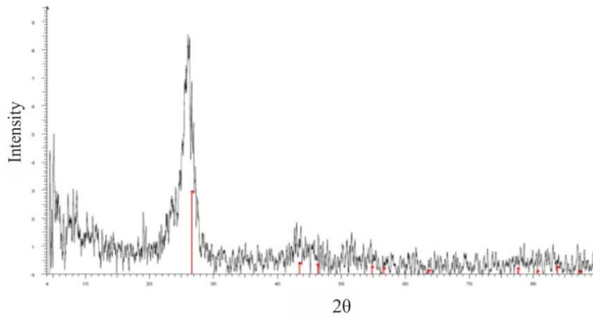
Fig. 3 – XRD images of the carbon nanotubes before the adsorption.
