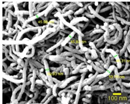
Fig. 8 – SEM of the carbon nanotubes after the adsorption  $\text{Ni}^{2+}$ .
