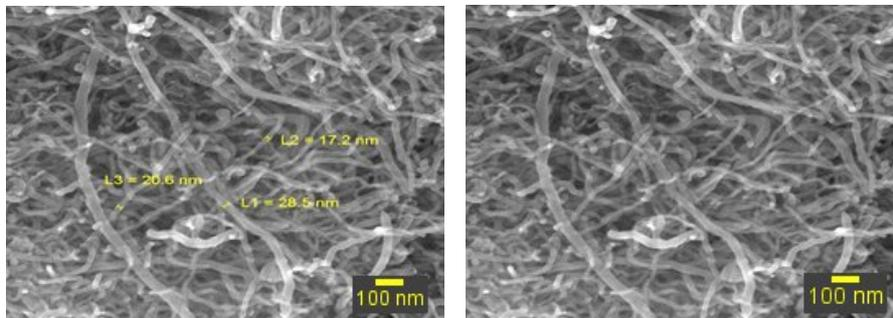
Fig. 6 – SEM correspond to the carbon nanotubes before the adsorption ligand.
