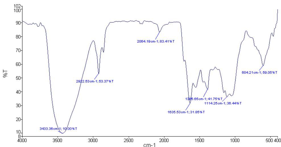
Fig. 1 – FT-IR spectrum of the adsorbent before the adsorption Ni (II).
