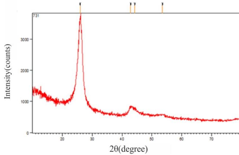
Fig. 5– XRD images of the adsorbent plus ligand after the adsorption.
