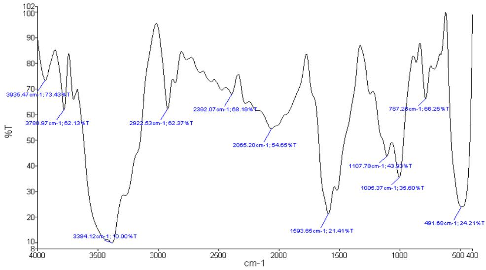
Fig. 2 – FT-IR spectrum of the adsorbent after the adsorption Ni (II).
