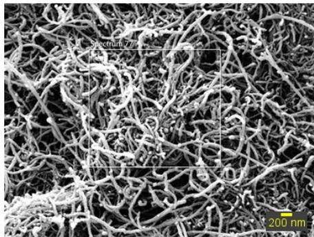
Fig. 7 – SEM image of carbon nanotubes added ligand before the adsorption  $\text{Ni}^{2+}$ .
