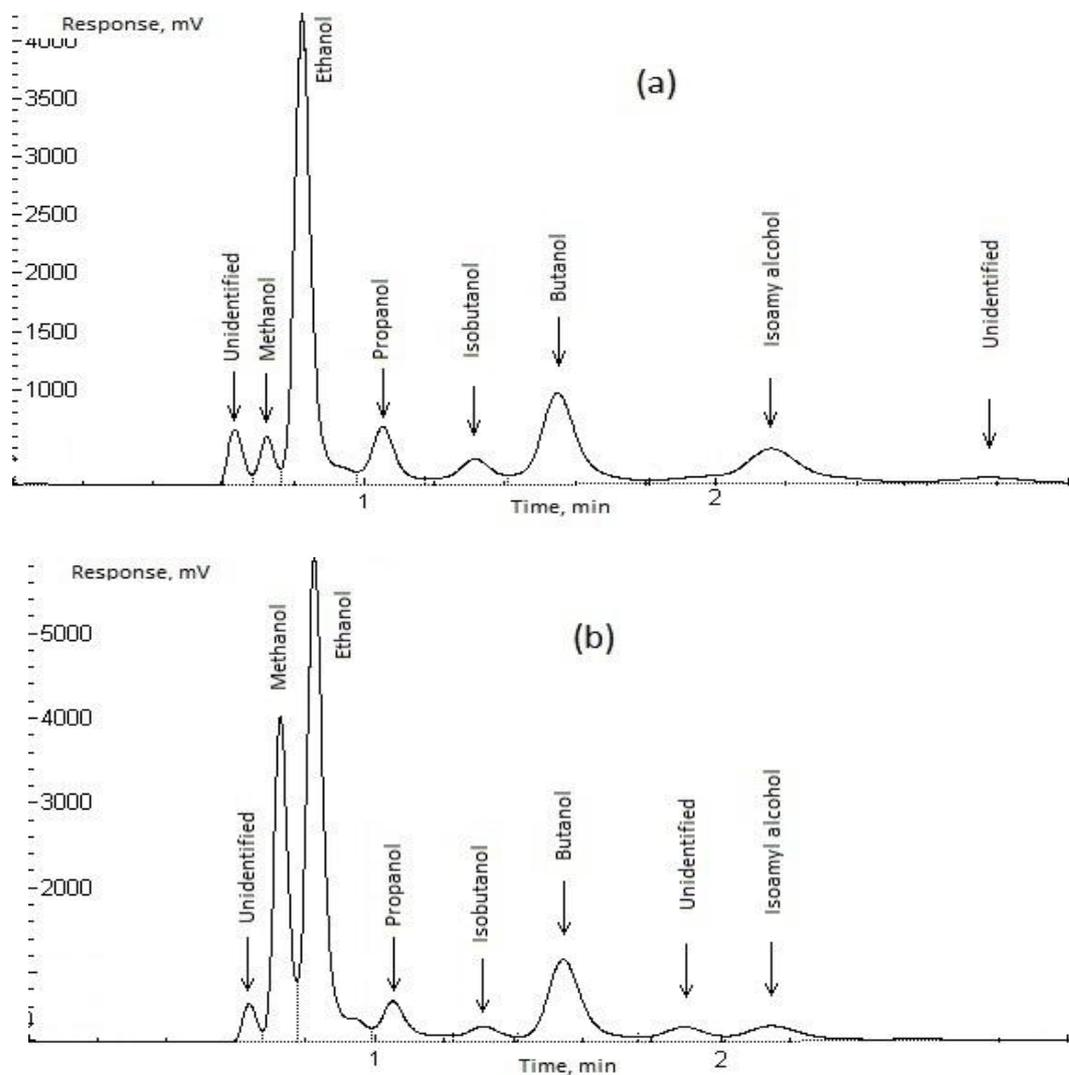
Fig. 2 – Chromatograms of the blood samples with a 0.2 % admixture of ‘646’ (a) and ‘647’ (b) MOS.
