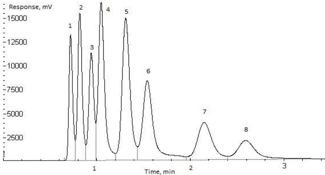
Fig. 1 – Typical GC image of eight homologous alcohols manifesting themselves through the corresponding nitrite esters: methanol (1), ethanol (2); isopropyl alcohol (3); propanol (4); isobutyl alcohol (5); butanol (6); isoamyl alcohol (7), and amyl alcohol (8).
