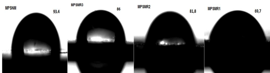
Fig. 7 – Angle contact of MPSNM, MPSMR1, MPSMR2 and MPSMR3.
