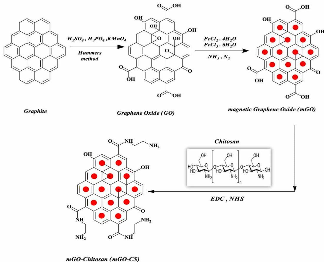
Fig. 1 – Scheme of mGO-CS synthesis steps.
