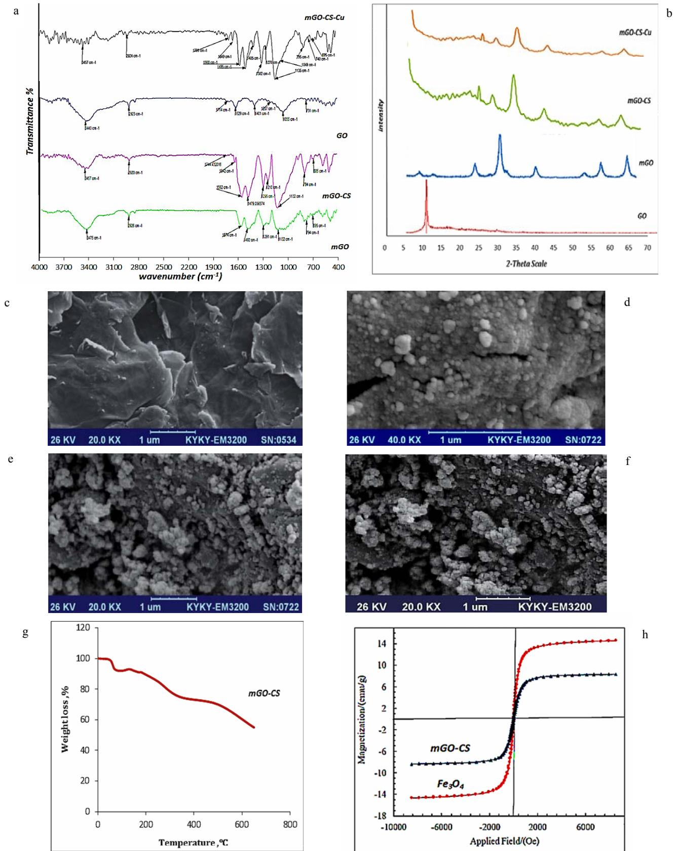
Fig. 3 – Characterization of the adsorbent: (a) FTIR pattern of GO, mGO, mGO-CS, mGO-CS-Cu; (b) XRD pattern of GO, mGO, mGO-CS, mGO-CS-Cu; (c) SEM image of GO; (d) SEM image of mGO; (e) SEM image of mGO-CS; (f) SEM image of mGO-CS-Cu; (g) TGA analysis of mGO-CS; (h) VSM magnetization curves of  $Fe_3O_4$  and mGO-CS.
