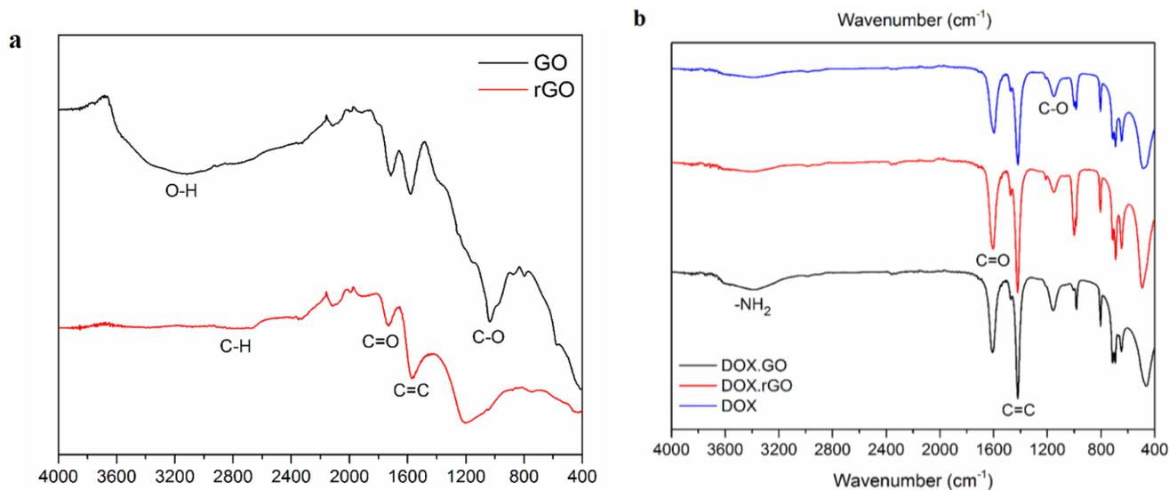
Fig. 1 – The FTIR spectra of graphene oxide (GO) and reduced graphene oxide (rGO) (a) and Doxorubicin (DOX), Doxorubicin graphene oxide (DOX-GO) and Doxorubicin reduced graphene oxide (DOX-rGO) (b).
