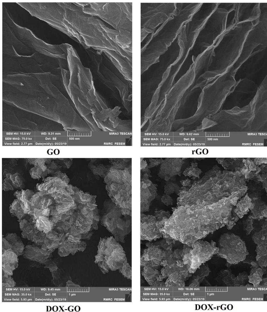
Fig. 3 – The Field emission scanning electron microscopy (FESEM) images from graphene oxide (GO), reduced graphene oxide (rGO), Doxorubicin (DOX), Doxorubicin graphene oxide (DOX-GO) and Doxorubicin reduced graphene oxide (DOX-rGO).
