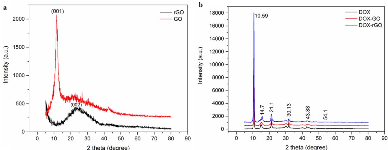
Fig. 2 – The XRD patterns of graphene oxide (GO) and reduced graphene oxide (rGO) (a) and Doxorubicin (DOX), Doxorubicin graphene oxide (DOX-GO) and Doxorubicin reduced graphene oxide (DOX-rGO) (b).
