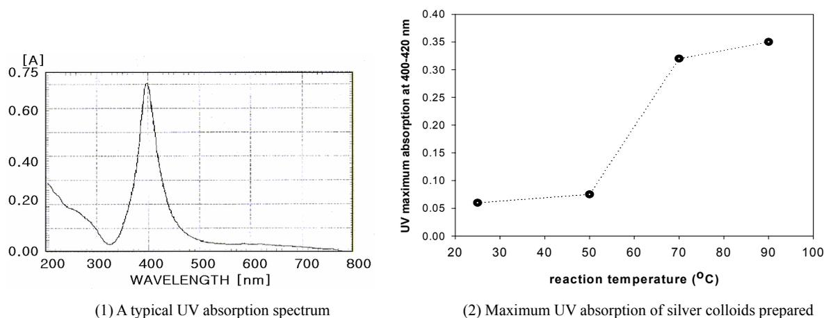
Fig. 3 – The typical UV absorption spectrum and the maximum UV absorption by silver colloid formed by the alcohol reduction of silver nitrate at various reaction temperatures in the presence of stabilizer (reaction time, 2 hrs).
