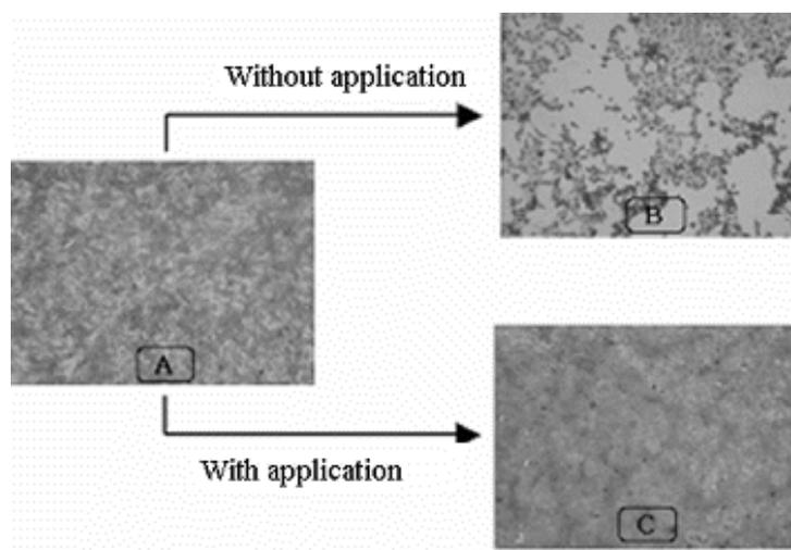
Fig. 6 – Comparison of anti-viral activity using formulated Silver/TiO<sub>2</sub>.
