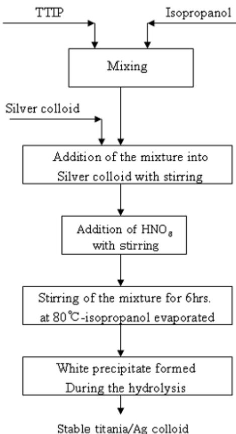
Fig. 2 – Procedure for manufacturing of the  $\text{TiO}_2/\text{Ag}$  formulation colloid.
