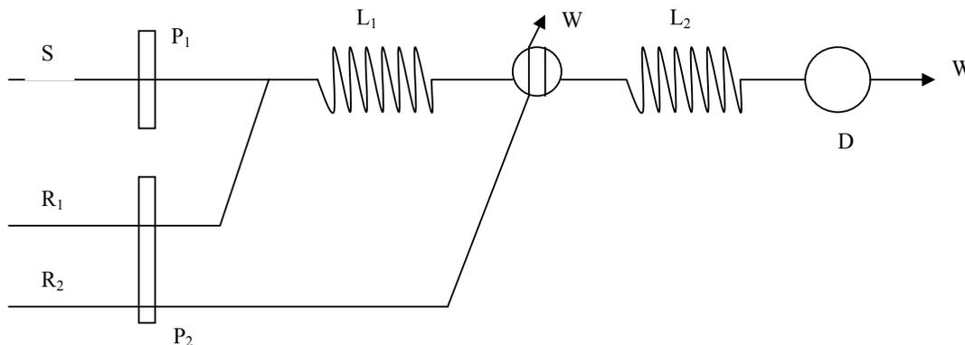
Fig. 3 – Schematic rFIA manifold. P<sub>1</sub> and P<sub>2</sub>, peristaltic pumps; I, injection valve; S, carrier-sample solution stream, R<sub>1</sub>, reagent 1; R<sub>2</sub>, reagent 2; L<sub>1</sub>, reactor 1; L<sub>2</sub>, reactor 2; D, spectrophotometric detector; and W, waste.
