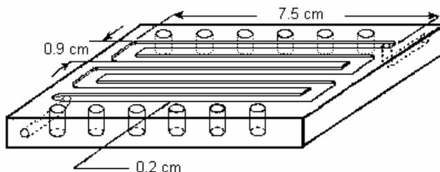
Fig. 2 – Methacrylate piece of the sandwich type gas-diffusion unit. The gas diffuser is made from two methacrylate blocks with a sandwiched porous membrane. The groove carved in the pieces formed a channel that is split by the membrane.
