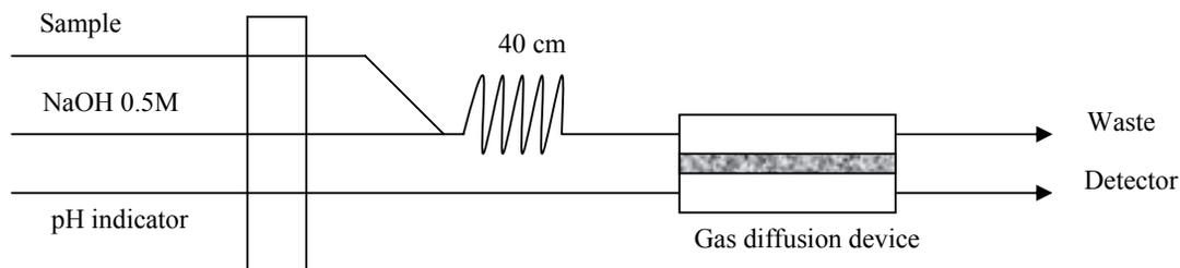
Fig. 4 – Continuous-flow manifold used for ammonia separation and spectrophotometric measurements based on the color change of a pH indicator and gas diffusion device.
