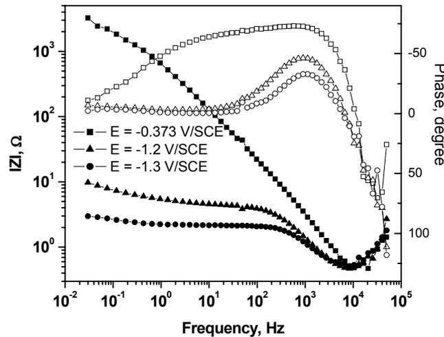
Fig. 7 – Bode diagrams at Ni electrode in artificial seawater at 25°C.
