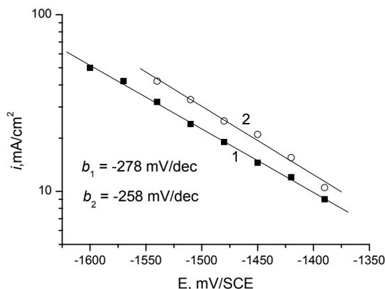
Fig. 2 – Tafel lines for the HER on Ni electrode in artificial seawater at 25°C:
